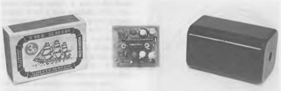
*Single limiter (centre) with case (right) for holding two for stereo.*
