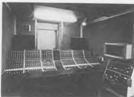
*A Calrec 40-channel mixing desk inside a Type B stereo control vehicle*
