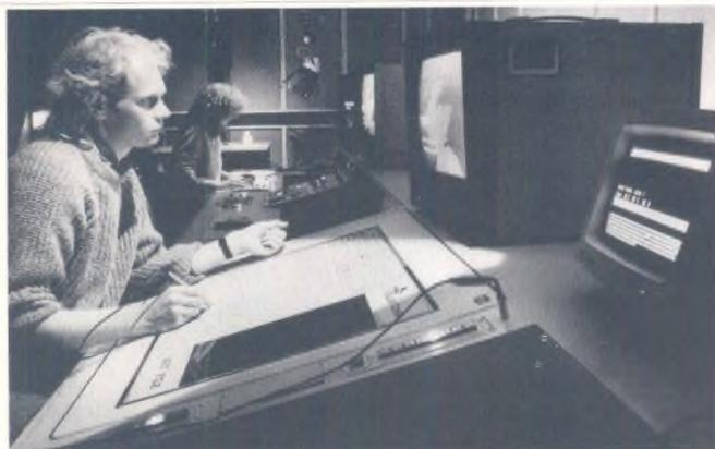
*The graphic artist is drawing with the magnetic pen on the graphics tablet whilst observing the effect on a colour monitor. The system VDU, which displays informative messages, is shown on the right.*
