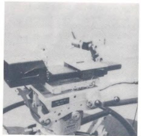
To help achieve compatibility between different camera/lens combinations, and to compensate for large temperature differences encountered in OB situations, the camera mounting shoe is sprung loaded.
