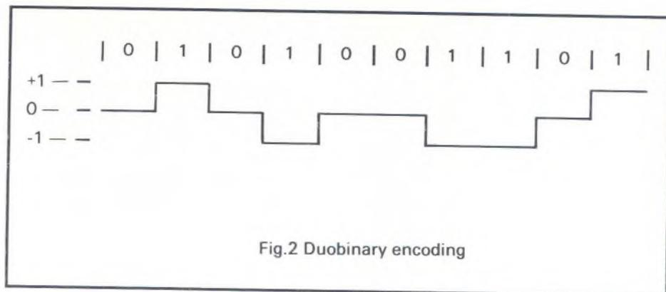
Fig.2 Duobinary encoding
