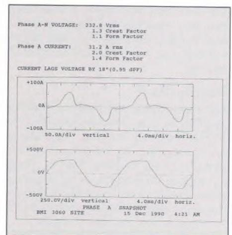
Fig. 2: current and voltage waveforms at a typical load centre
