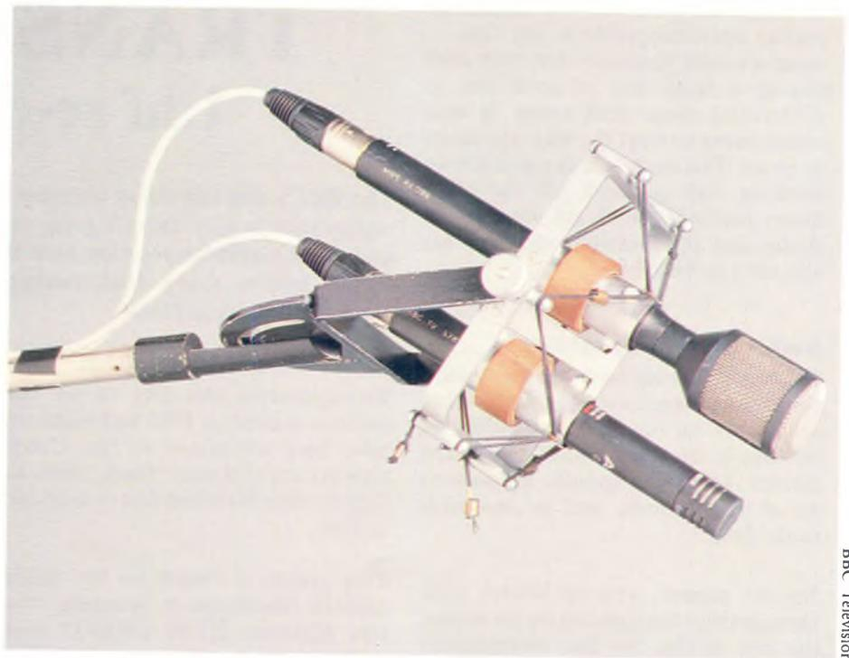
Double microphone mount carrying M-S mics as used on booms
