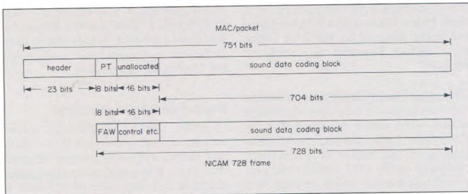
Fig. 1a: the frame structures of the MAC/packet and NICAM 728 systems
