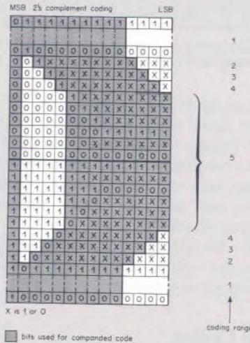
The diagram above shows the look-up table used in NICAM 728 to determine which 10-bit section of every 14-bit sample (within a given sound-coding block of thirty-two samples) will be transmitted. Note that three bits-per-block of thirty-two samples are needed to convey the range-code information to the decoders; in NICAM 728 these are conveyed using **Signalling-in-Parity** which is explained on page 17.
