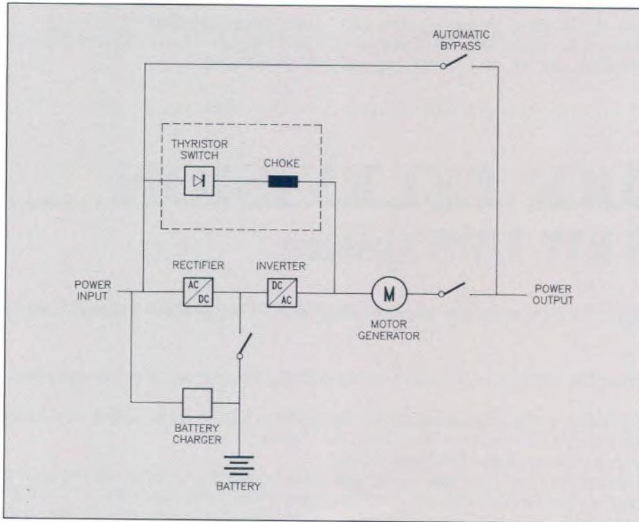
Fig. 1: the UPS system's block diagram
