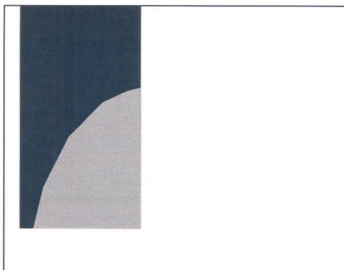
The photograph on the left shows presenter Martyn Lewis with graphic insert. On the right is the mask signal required to control the keying. The grey area allows CSO keying where the presenter's shoulder is likely to overlap the graphic. The black area forces the graphic through regardless of the backing and the white area forces the presenter and backing through.
