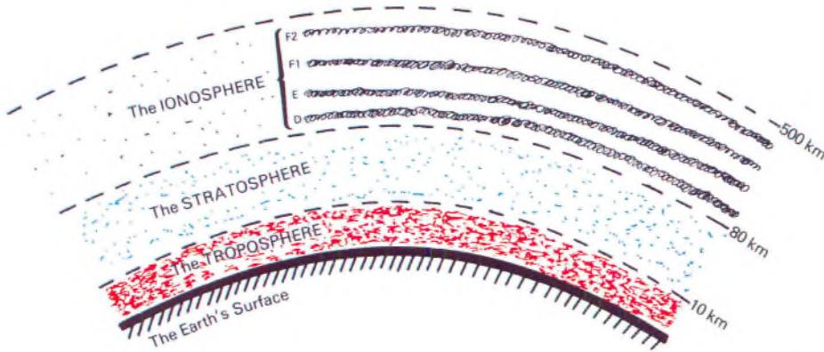
Fig 1: the earth's atmosphere showing the troposphere, the stratosphere and the D, E, F1 and F2 layers of the ionosphere
