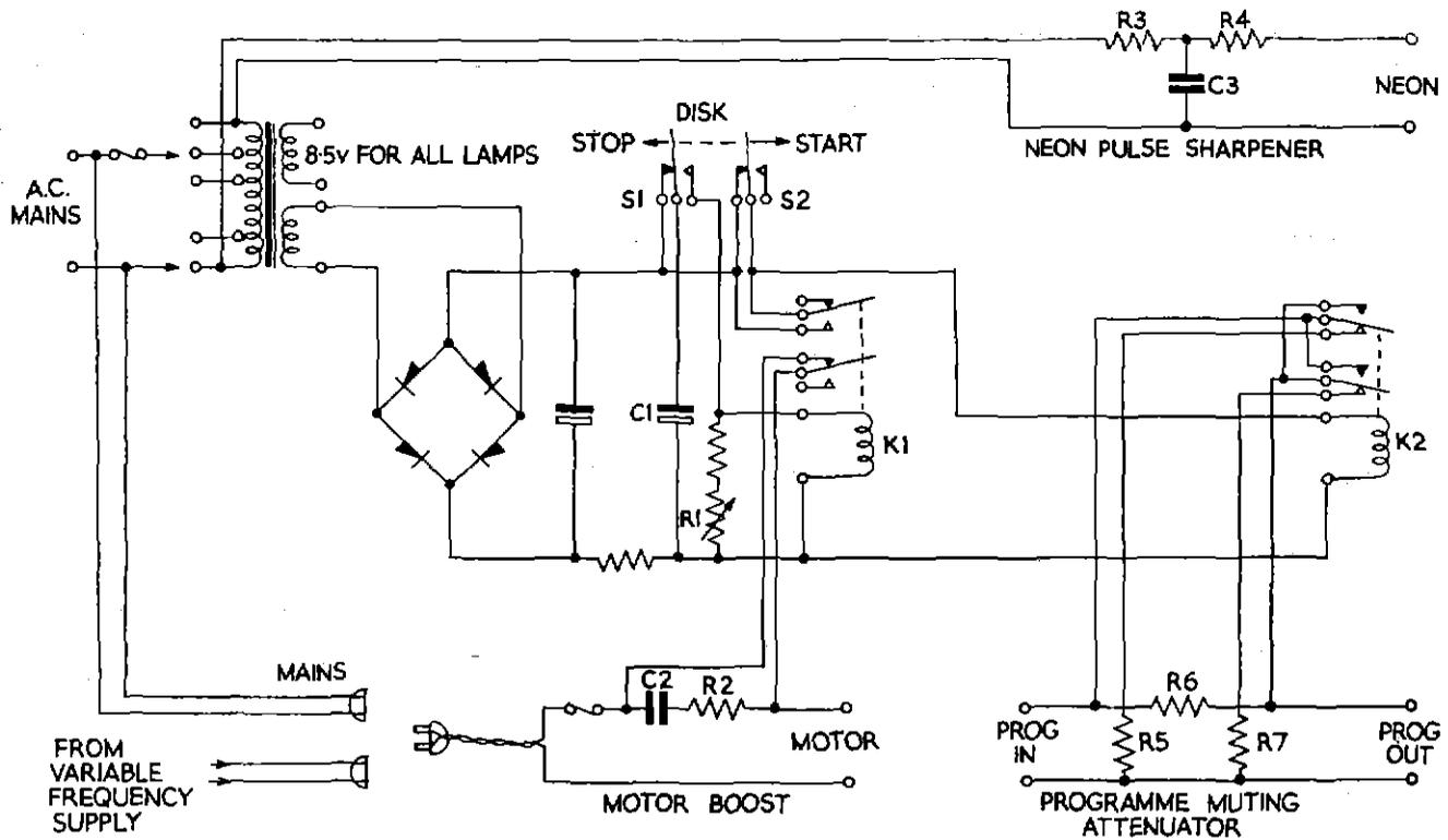
Fig. 5 — Diagram of circuit arrangements of control system
