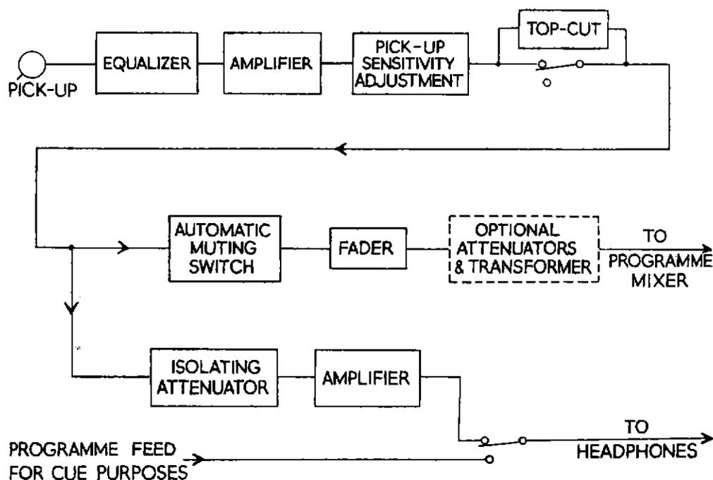
Fig. 8 — Block-schematic diagram of amplifier section
