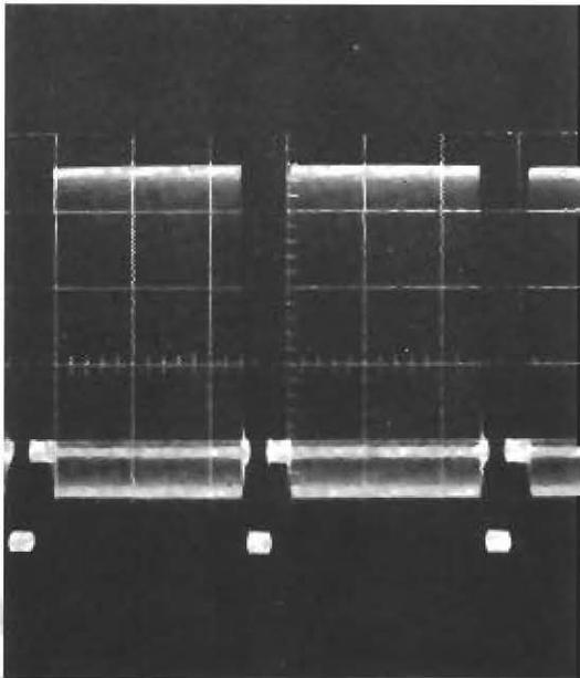
Fig. 11c — 4.4 Mc/s sine-wave after modulation and envelope demodulation
