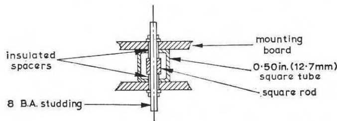
Fig. 15 — Construction of co-axial transmission-lines
