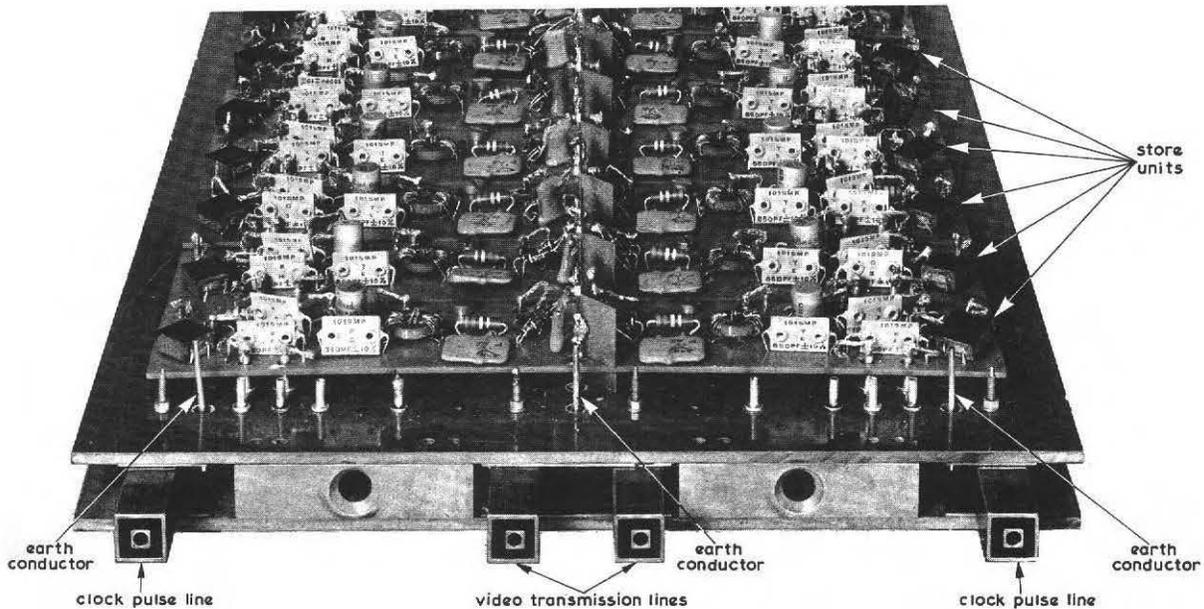
Fig. 14 — Store assembly layout using co-axial transmission-lines
