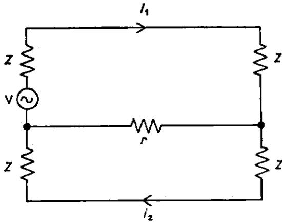
Fig. 11 — Equivalent circuit showing common earth impedance
