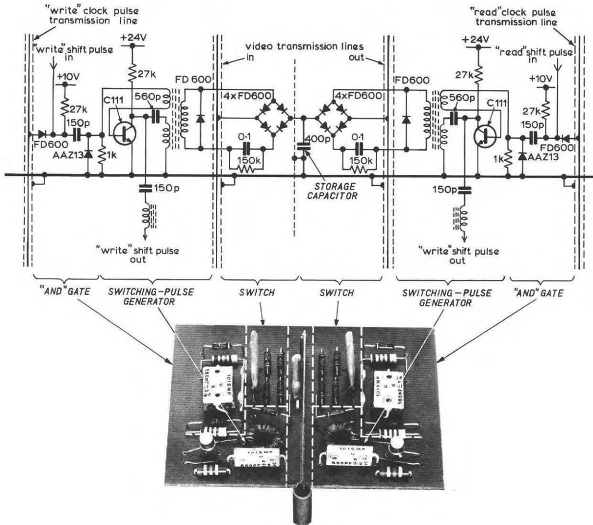
Fig. 7 — A specimen design of store unit
