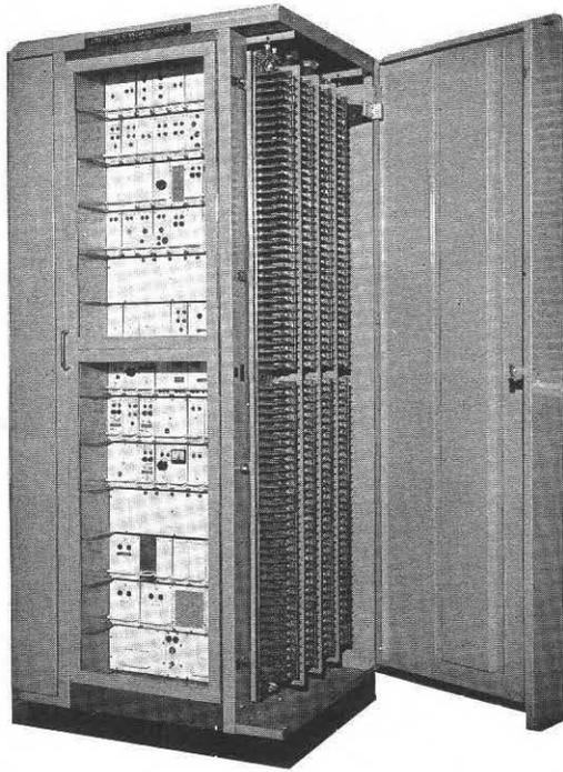
Fig. 19 — Prototype machine showing half of store assembly
