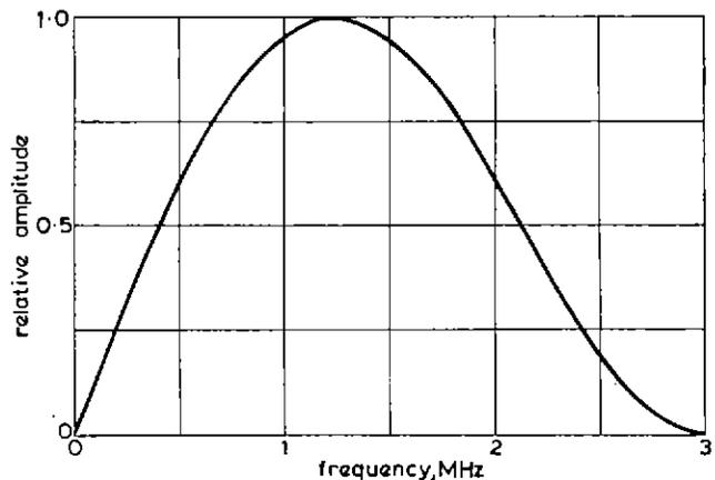
Fig. 8 — Bipolar sine-squared pulse spectrum
