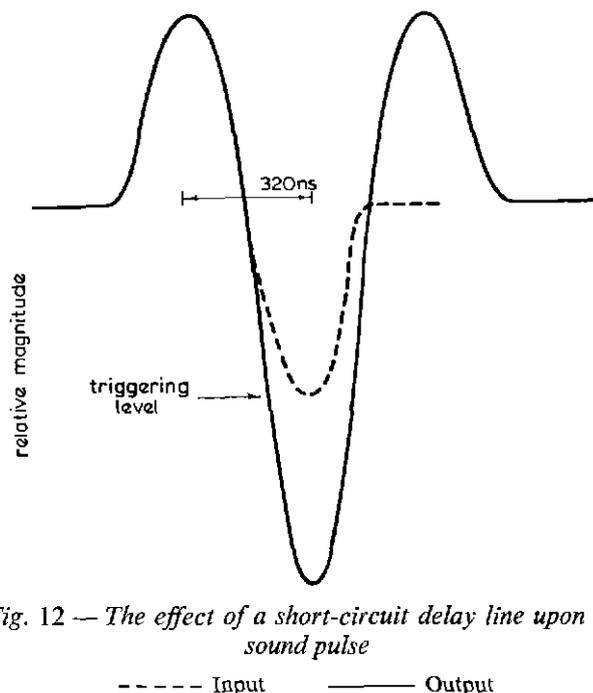
Fig. 12 — The effect of a short-circuit delay line upon the sound pulse
