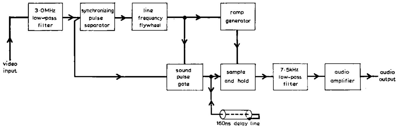
Fig. 11 — Pulse-sound decoder
