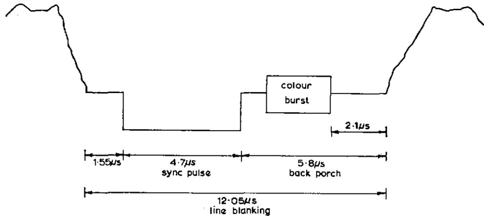
Fig. 1 — Conventional line-blanking interval. All durations nominal
