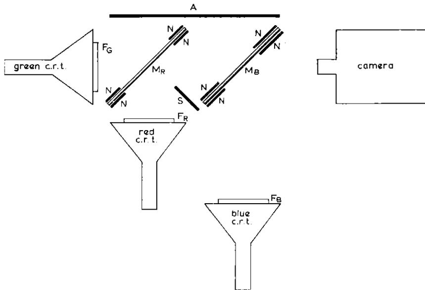
$F_R, F_G, F_B$ —Absorption-type shaping filters
