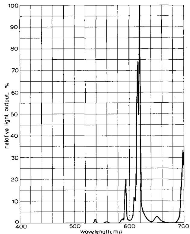
Fig. 3 — Spectral emission of the red phosphor
