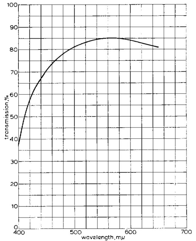
Fig. 12 — Spectral transmission of camera lens used for the film exposure tests
