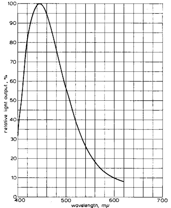
Fig. 5 — Spectral emission of the blue phosphor
