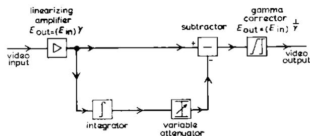
Fig. 13 — Illustration of a veiling-glare corrector
