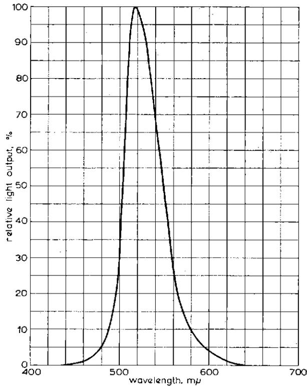
Fig. 4 — Spectral emission of the green phosphor
