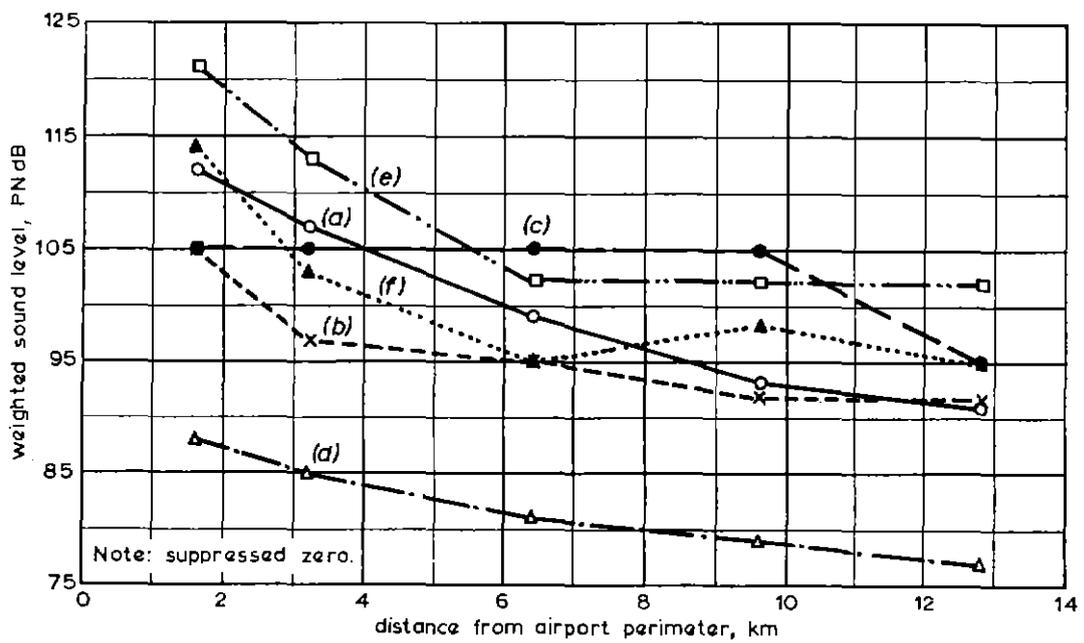
Fig. 13 — Weighted noise levels as a function of distance from the perimeter of London (Heathrow) Airport
