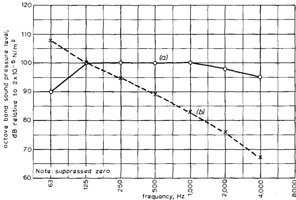
Fig. 9 — Noise spectra used in 1966 roof insulation demonstration recordings
