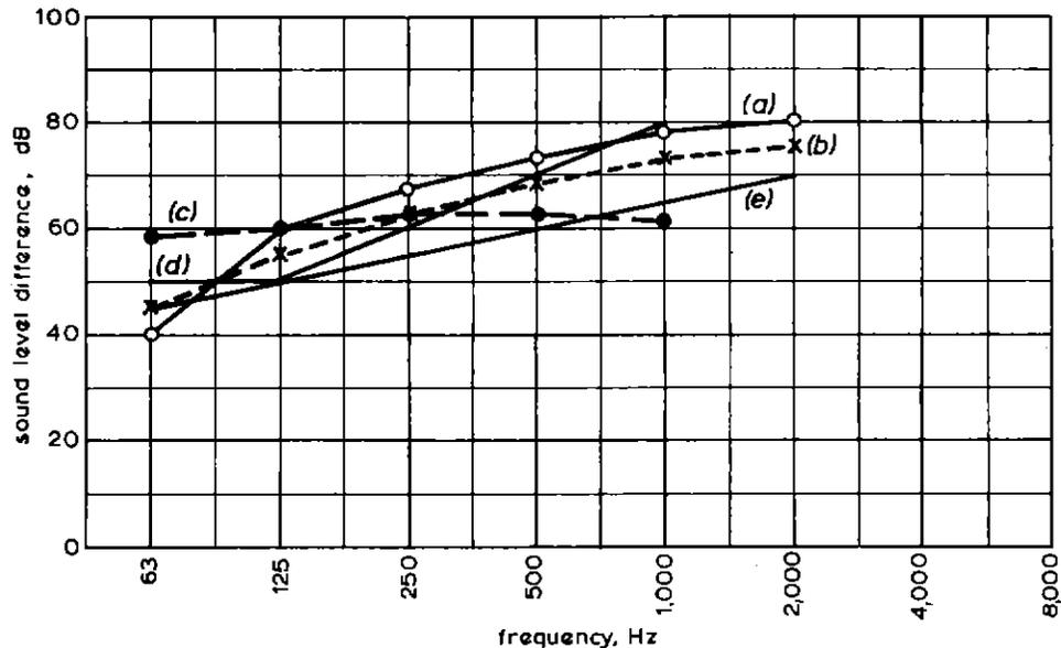
Fig. 17 — Sound level differences between aircraft noise levels and permissible background noise levels
