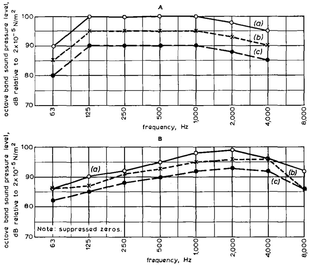
Fig. 12 --- Effect on a weighted sound level of transposing a spectrum
