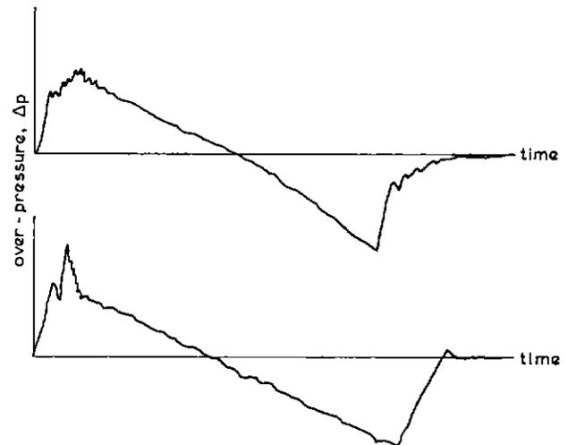
Fig. 2 — Observed pressure waves of two sonic booms
