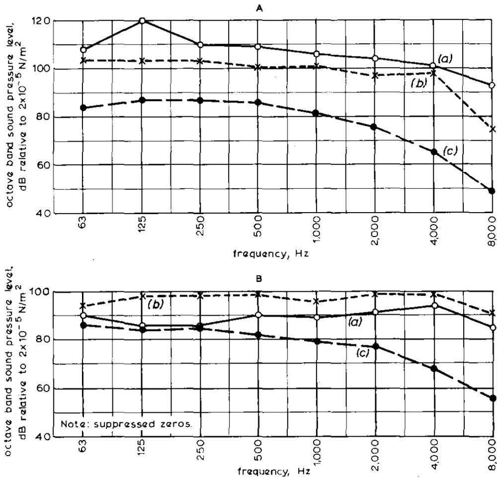
Fig. 14 — Measured aircraft noise spectra at different distances from an airport periphery
