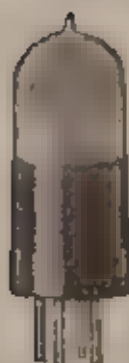
The Wundell Duff Emmitter Voltage 2.5 volts Consumption 100 m.p. Wt for Detector and I.F. 14 Wt for H.F. amplification 14
