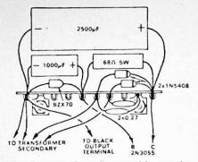
The diagram above is to guide you in wiring the 10-lug tagstrip used to support the basic rectifier components and those associated with the zener diode. Note the polarity of all three diodes, and of the electrolytics.
