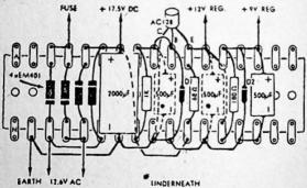
Filtering immediately after the rectifiers, is by one 2000uF 25VW electrolytic capacitor, the voltage at this point being about 17.5. This is sufficient filtering for this position, as it normally feeds a high level output stage, and earlier stages in the amplifier have extra filtering as required.
