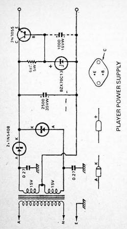
The circuit for the new supply, which is basically a conventional full-wave rectifier followed by a simple series-pass regulator.
