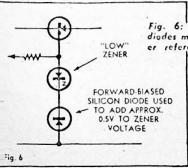
Fig. 6: Showing how "low" xener diades may be used to provide a higher reference voltage with a silicon diade.
