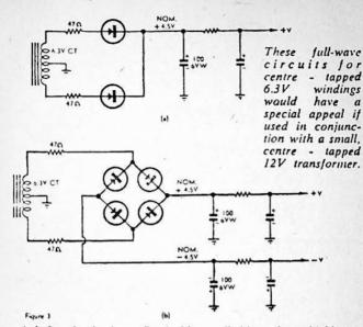
As before the circuits are fitted with surge limiting resistors, in this case having a value of 47 ohms to permit a maximum diode surge current of 90mA. Lower values may of course be used with diodes having higher surge ratings.
