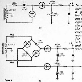
Novel arrangements which give peak or unloaded DC output approximately equal to 1.5 times the peak value of AC supply circuit. They would be suitable situations where voltage hum level were not critical factors.
