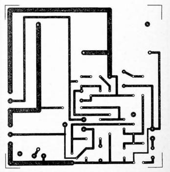
Fig.3.4 The copper track pattern for the MOSFET power amplifier
