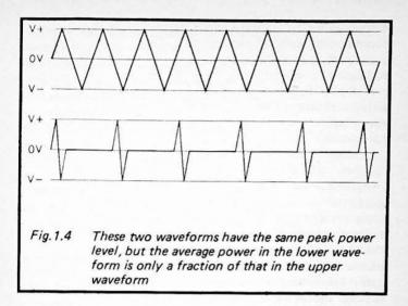
for both waveforms, but the average output power (and current consumption) are much lower for the pulsed waveform. This means that the supply voltage sags relatively little on a pulsed signal, permitting higher peak output powers to be produced. Provided the output transistors have suitably high ratings, on this type of signal relatively high peak output powers can be handled before the onset of clipping.
