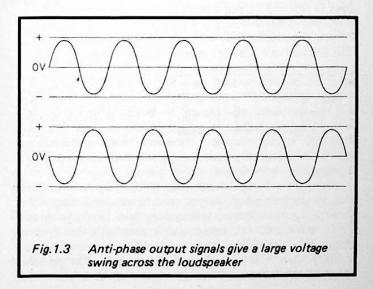
20 volts of the opposite polarity across the loudspeaker, this gives a total peak to peak value of 40 volts.
