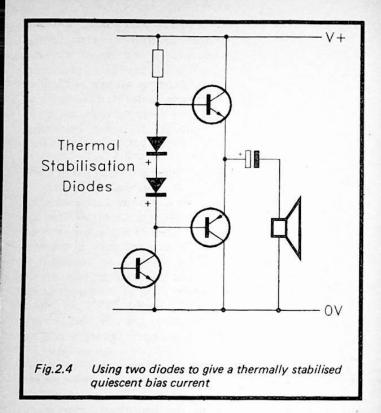
increase in the output bias current. Provided the diodes are suitable silicon types, they will have thermal characteristics that are a good match for the output transistors, and which give a stable quiescent current.
