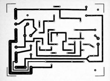
Fig.3.14 The track pattern for the inverting MOSFET power amplifier
