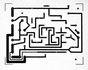
Fig.3.10 The copper track pattern for the power op. amp. unit
