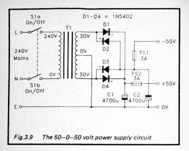
central 0-volt supply rail, and not a straightforward 100-volt supply. However, it requires few extra components in order to satisfy these modified requirements, and a suitably modified power supply circuit appears in Figure 3.9. Note that whereas the original power supply circuit could operate using either a 30-0-30 volt transformer (or one having twin 30volt secondary windings), or a 60-volt type, this design will only work using a 30-0-30 volt (or twin 30-volt secondary) type.
