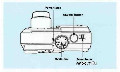
In the diagram above, the lever position T represents the Telephoto or "zoom in" setting used to capture distant objects. W represents the Wide angle or "zoom out" setting.
