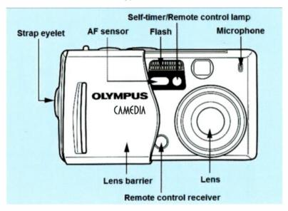
The above camera is switched on and off by moving the Lens barrier; alternatively a separate on/off switch is often located on the top of a camera. If the camera is not used for a few minutes it may go into standby mode to save power. You can usually exit standby mode by switching the camera back on or by gently pressing the shutter button. The shutter button is used to take photos and is shown on the diagram on the next page.
