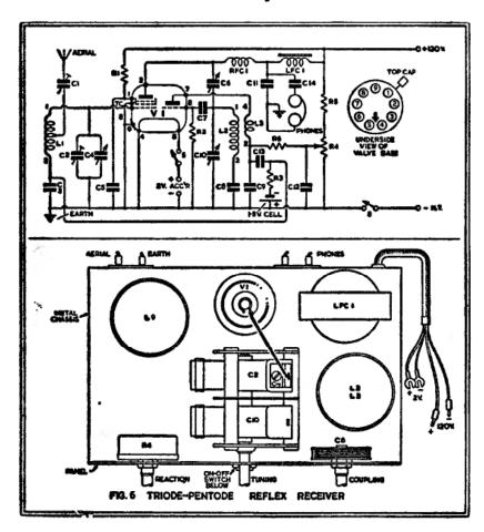
to-cray, and any method by which parts could be dispensed with was considered a major advantage. In a reflex receiver, one valve is made to perform the duty of two or more by shunting the signal round the circuit, by-passing any unwanted portion and returning it to its point of entry for yet further amplification. This system is not to be confused with the more orthodox process of using, perhaps, a double triode in a straight circuit one half as a detector and the other half as an amplifier.
