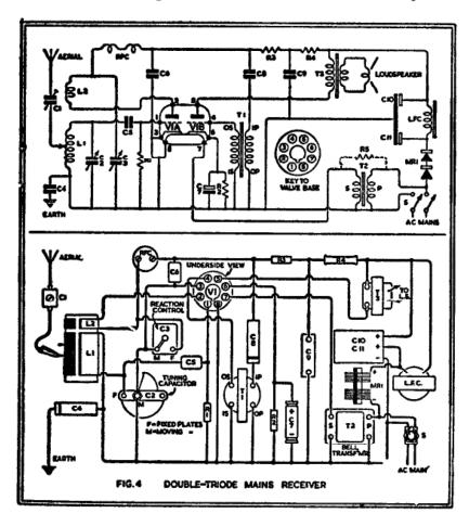
coil construction will present no difficulties. It is wound on a three-inch diameter former, three inches long, and the grid winding L1 consists of 45 turns of 22 S.W.G. enamelled wire with looped taps brought out at 15 and 30 turns. L2 is wound in the same direction and requires 28 turns of the same gauge wire. Constructional details of the coil are shown in Fig. 4.
