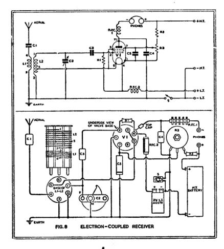
panel of metal. VI should be mounted horizontally to avoid having the anode lead unnecessarily long. The coils L1-2 are best wound on 6-pin formers, obtainable from any supplier dealing with short-wave components, complete with sockets to fit. Eddystone-threaded formers were used on the original. Three coils are usually sufficient to cover the popular bands, and the table gives the required turns and wave-band covered.
