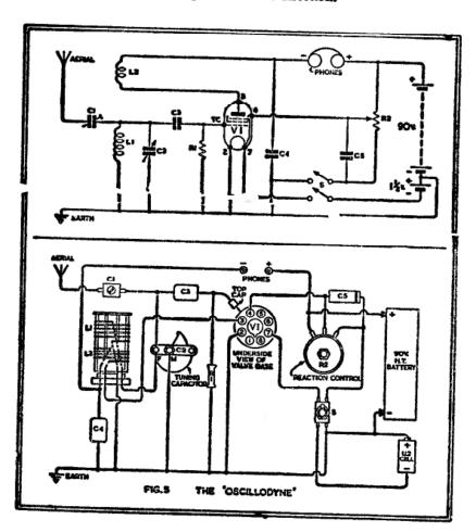
The coils are wound on 1½-inch diameter plug in coil formers. The author used Eddystone 6-pin formers which are readily obtainable in England though, of course, there is no reason why the constructor should not make up his own.
