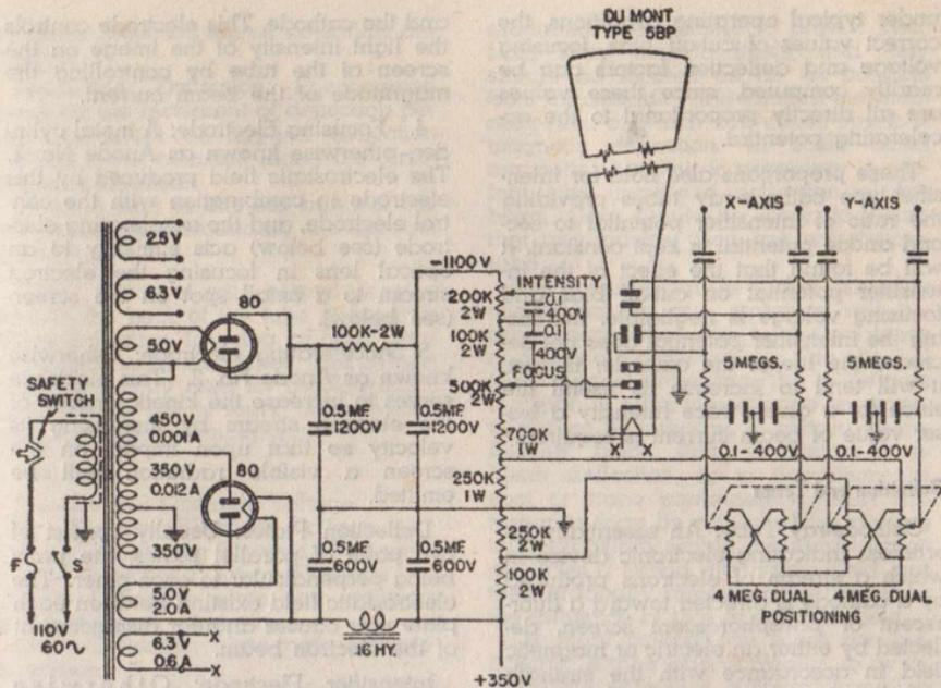
Fig. 3—Typical power supply for cathode-ray tube (no intensifier).
