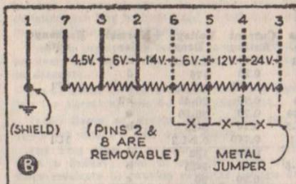
Fig. 1. The types A and B Ballastrons (metal ballast tubes) vary only in the rating of the resistance section between removable terminals 2 and 8. The type A is designed for a pilot light rated at 150 ma.; the type B is for a 250 ma. pilot light. The metal jumper may be snipped along the dotted lines that bisect the color-code dots, as shown at A, to unshort resistor sections inside the tube as shown at B (where X represents the snipping lines shown dotted in A).
