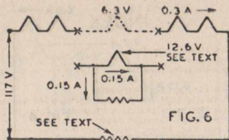
**FIG. 6—To substitute a 12.6 v. 150 ma. type for a 6.3 v. 300 ma. type, proceed as in discussion for Fig. 4. Value of shunt resistor is**
