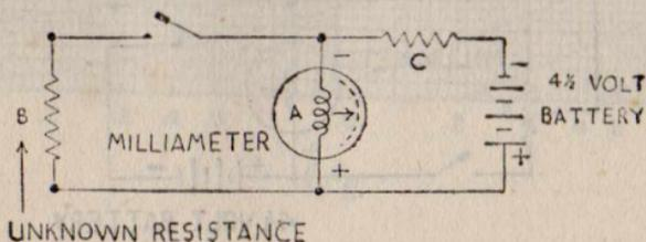
(g) To find ohmage value of unknown resistance by means of milliammeter, battery and any known resistor.
