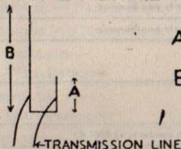
$$A = \left\{ \left( \text{WAVELENGTH IN METRES} \div 4 \right) \times 1.094 \right\} \text{ YDS.}$$
