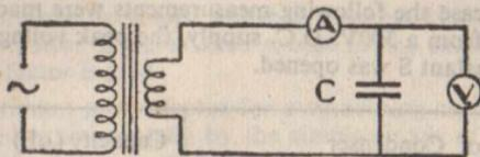
Fig. 10.—Capacity measurement by impedance method.
