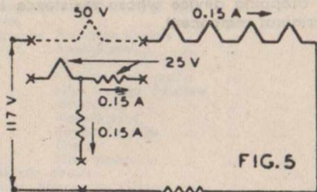
**FIG. 5—To substitute a 25 v. 300 ma. type for a 50 v. 150 ma. type** in string position as indicated, proceed as in discussion for Fig. 2. Value of shunt resistor R is
