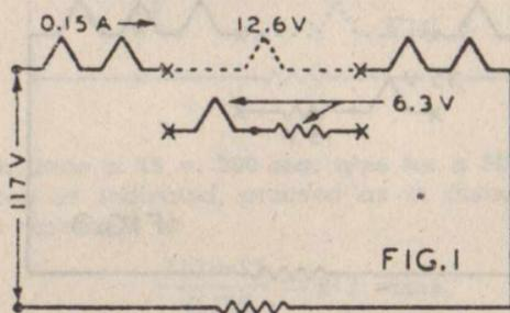
**FIG. 1—To substitute a 6.3 v. 150 ma. type for a 12.6 v. 150 ma. type,** calculate value of the resistor to be added in series with the 6.3-volt heater. Using the formula  $R = E/I$ , we have
