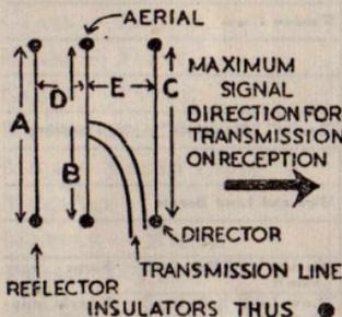
$$A = \left\{ 164 \div \left( \text{FREQUENCY IN MEGACYCLES} \right) \right\} \text{ YDS.}$$
