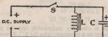
Fig. 9.—Electrolytic condenser used to absorb inductive surge.
