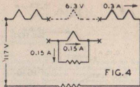
**FIG. 4—To substitute a 6.3 v. 150 ma. type for a 6.3 v. 300 ma. type,** calculate value of shunt resistor to be added across the 0.150-ampere heater. Using the formula  $R = E/I$ , we have
