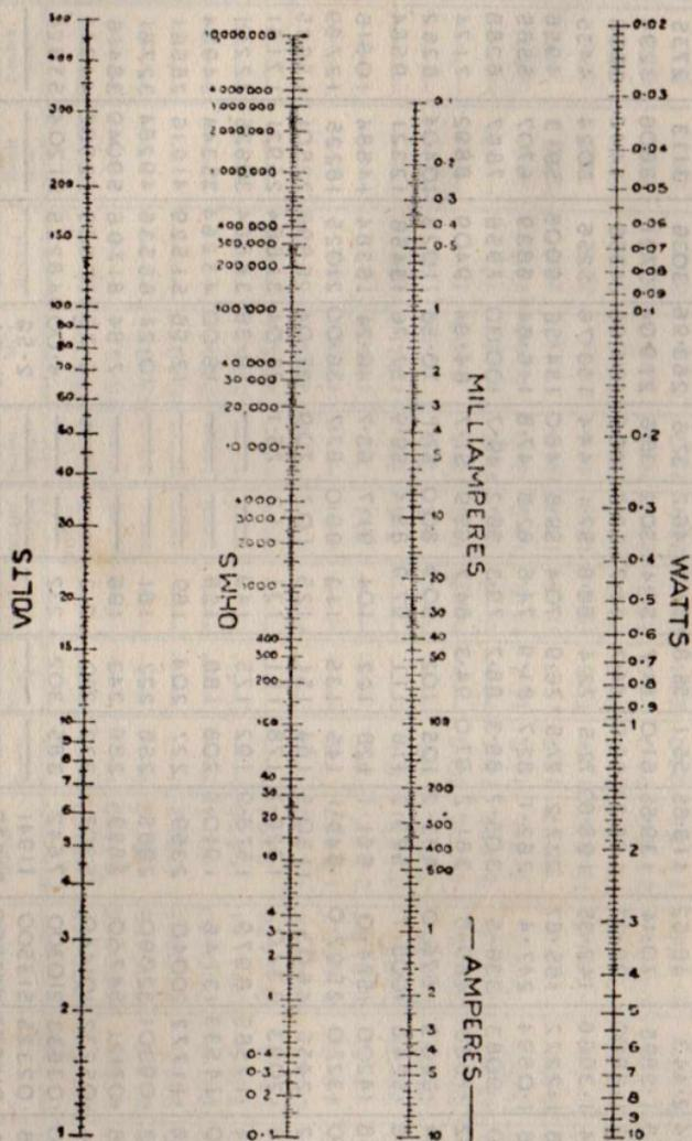
A straight edge placed across any two known quantities on the Calculator will enable either of the two unknown quantities to be read off.
