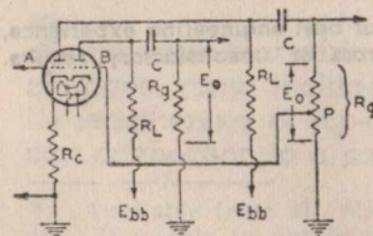
Information given for triode amplifiers, in general, applies also to this case. Condensers  $C$  have been chosen to give output voltages equal to  $0.9 E_o$  for  $f_1$  of 100 cycles. For other values, multiply values of  $C$  by  $100/f_1$ .
