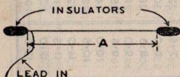
$$A = \left[ \left\{ 164 (\text{NUMBER OF HALF WAVES ON THE AERIAL MINUS } \cdot 05) \right\} \div \text{FREQUENCY IN MEGACYCLES} \right] \text{ YDS.}$$
