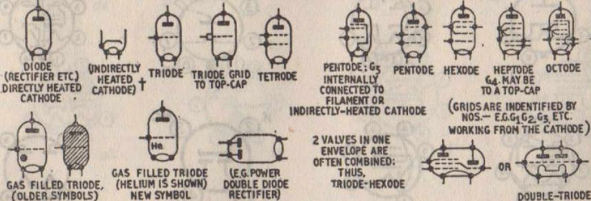
† ANY TYPE SHOWN MAY HAVE AN INDIRECTLY HEATED CATHODE
