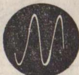
Sine waves of a tuning fork. A-440 cycles per second.
