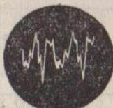
G-392 cycles per second as produced by a single reed of an accordion.
