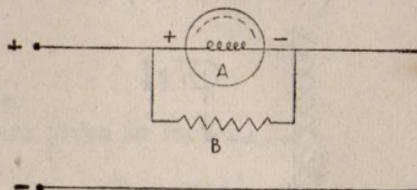
(d) To find ohmage value of unknown resistance by using a voltmeter and battery.
