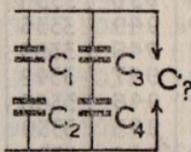
$C = \frac{1}{\frac{1}{C_1} + \frac{1}{C_2}} + \frac{1}{\frac{1}{C_3} + \frac{1}{C_4}}$                                 |
