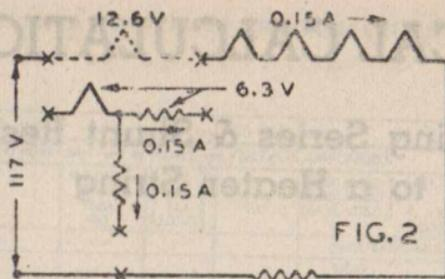
**FIG. 2**—To substitute a 6.3 v. 300 ma. type for a 12.6 v. 150 ma. type in string position as indicated, calculate value of resistor R which must shunt all components in the heater string except the substitute type. Using the formula  $R = E/I$ , we have
