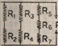
$R = \frac{1}{\frac{1}{R_1 + R_2} + \frac{1}{R_3 + R_4} + \frac{1}{R_5 + R_6 + R_7}}$ | <p style="text-align: center;"><b>CONDENSERS<br/>IN SERIES-PARALLEL</b></p>
