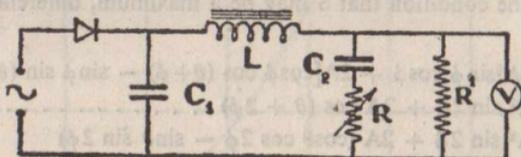
Fig. 8.—Circuit for demonstration of optimum power factor for smoothing condenser
