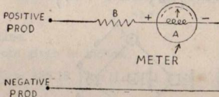
(c) To increase range of milliammeter for current reading by any desired multiplier.
