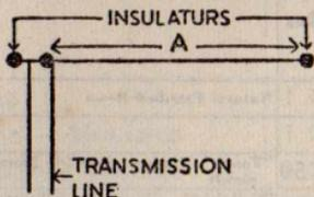
$$A = \left[ \left\{ 164 \left( \text{NUMBER OF HALF WAVES ON THE AERIAL REQUIRED, MINUS } 0.5 \right) \right\} \div \left( \text{FREQUENCY IN MEGACYCLES OF MOST USED BAND} \right) \right] \text{ YDS.}$$
