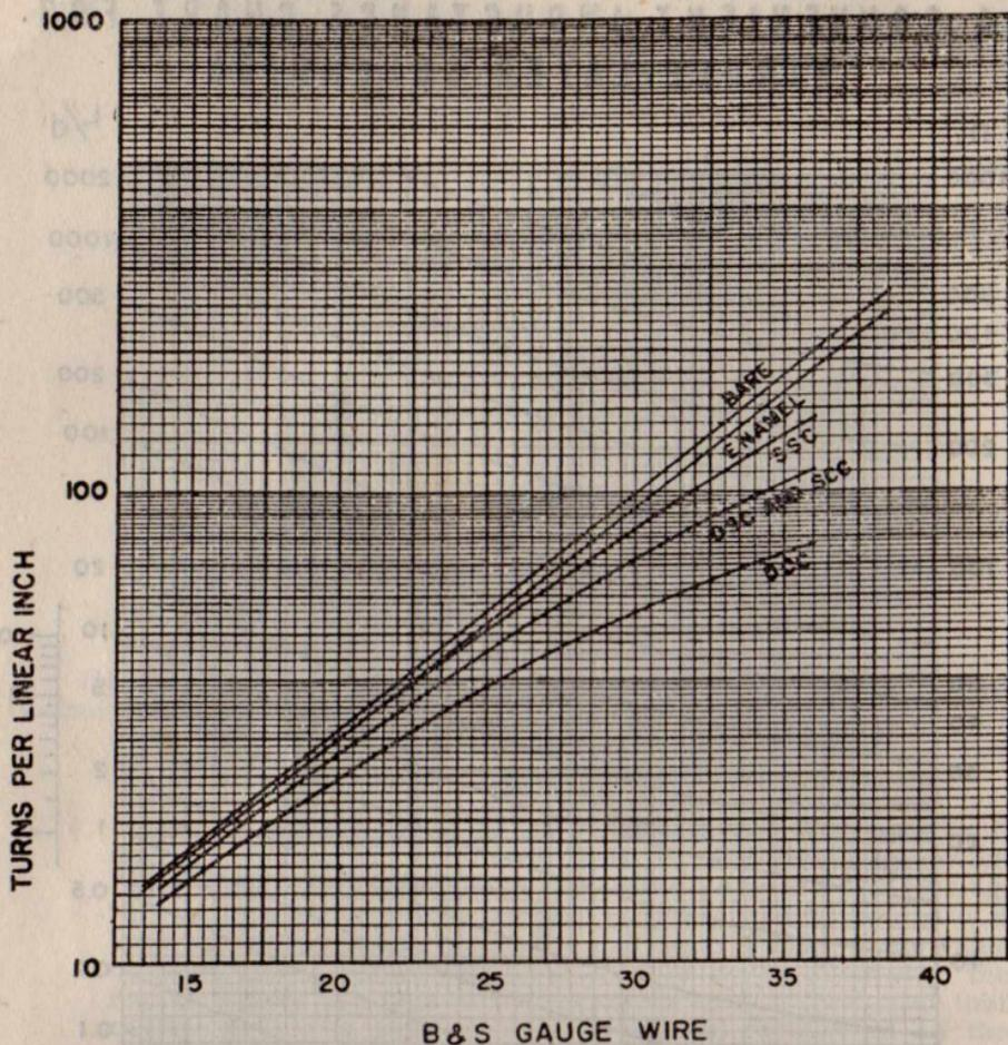
● ON THESE TWO PAGES are presented charts for determining the number of turns and the size of wire to be used in order to obtain a given inductance on a given winding form.
