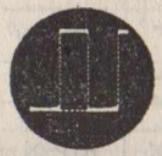
Oscillogram of the response of a given amplifier to a 100 kilocycle square-wave signal.
