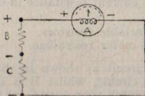
(f) To find ohmage value of unknown resistance by means of milliammeter and battery.
