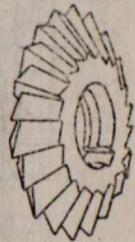
FIG. 17. CONVEX MILL.
