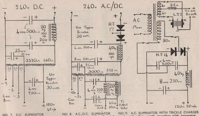
NO. 7. D.C. ELIMINATOR NO. 8. A.C./D.C. ELIMINATOR NO. 9. A.C. ELIMINATOR WITH TRICKLE CHARGER WARNING ! Under certain circumstances the circuits of Figs. 7 and 8 may be "live" to earth, together with apparatus connected to them. If earthing is necessary the negative lead must be earthed through a condenser of .1 mfd. 400 volt working capacity.
