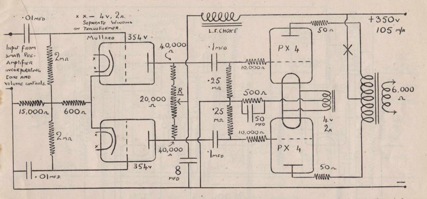
To adjust R for balance :—Insert 50 \_\_\_ resistor at X and connect phones or an oscilloscope across its ends. Feed in a small signal of constant pitch between 400—1,000 c.p.s. Adjust R until the response at X is at its minimum.
