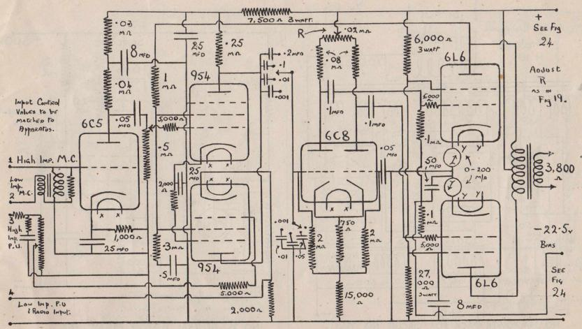
NO. 23. 50 WATT A.C. AMPLIFIER (CLASS AB<sub>2</sub>) Basic circuit by kind permission of G. I. Turner.
