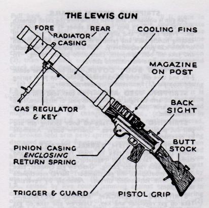
LOADING.—(a) Place cocking handle forward. Fit magazine on magazine post, with magazine catch to right, on British and American 47-round magazine, and magazine with round indicator facing firer on American 97-round. (b) Push magazine down on catch until it engages. Turn magazine by hand until resistance is felt. Pull back cocking handle. Gun is now ready to fire.
