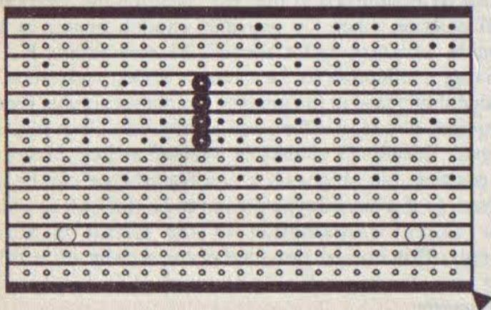
Fig.2.18 The underside of the two tone train horn
