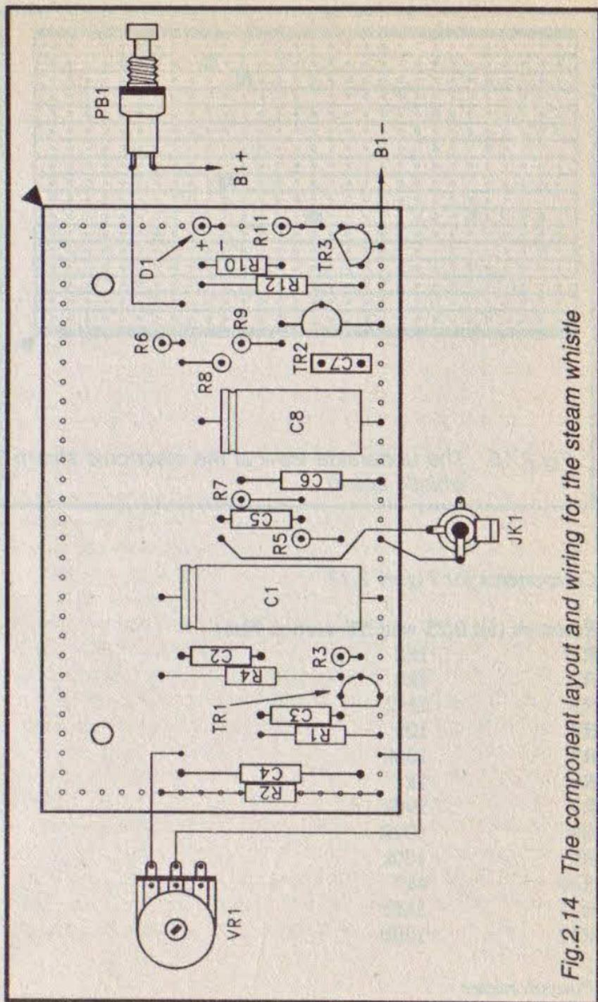
Fig.2.14 The component layout and wiring for the steam whistle
