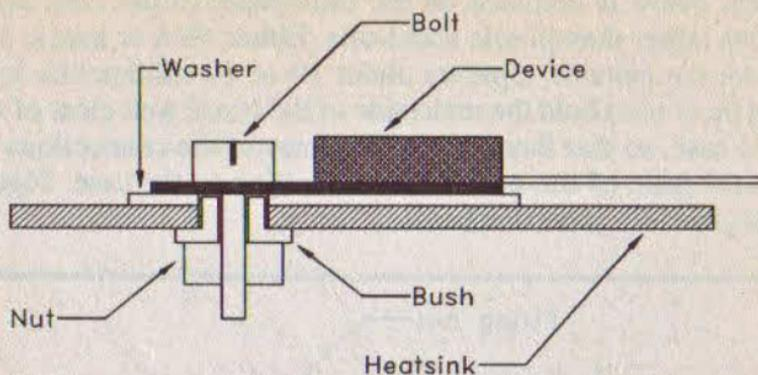
*Fig.1.8 Insulating a plastic power device from its heatsink*
