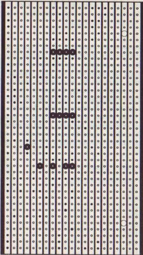
*Fig.1.24 The underside of the pushbutton controller board*
