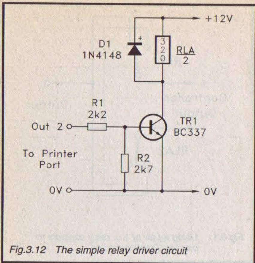
Fig.3.12 The simple relay driver circuit
