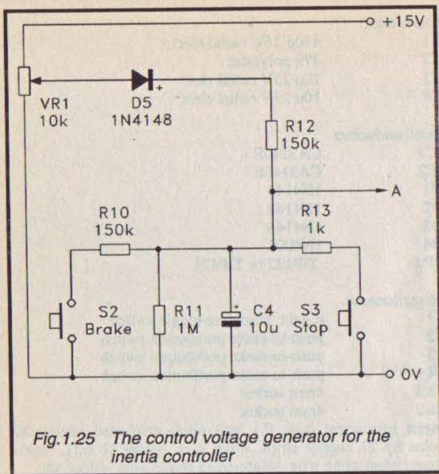
*Fig.1.25 The control voltage generator for the inertia controller*
