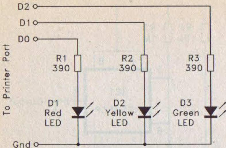
*Fig.3.6 Driving three l.e.d.s from the printer port*
