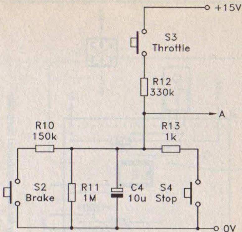
*Fig.1.22 The control voltage generator for the pushbutton controller*
