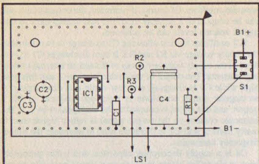
Fig.2.17 The component layout and wiring for the two tone train horn
