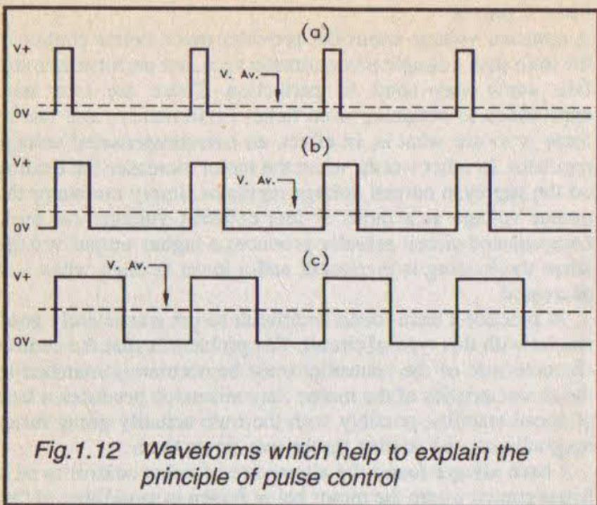
*Fig.1.12 Waveforms which help to explain the principle of pulse control*
