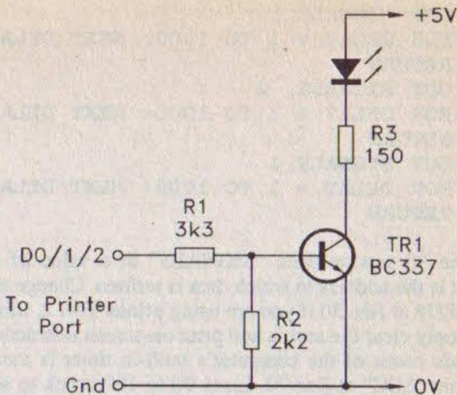
*Fig.3.7 A l.e.d. driver which gives a l.e.d. current of 20mA*
