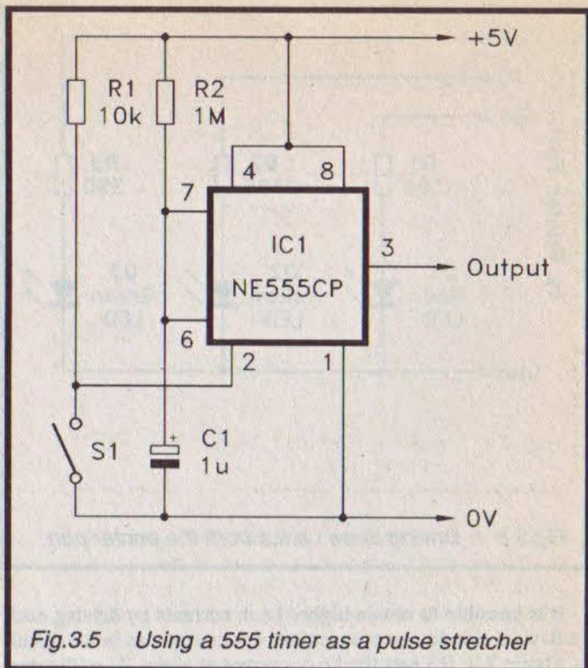
*Fig.3.5 Using a 555 timer as a pulse stretcher*
