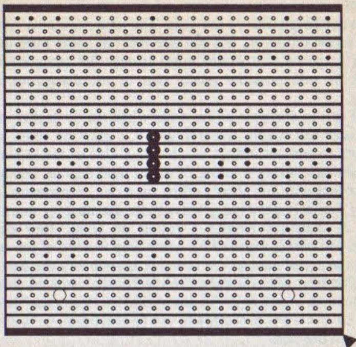
*Fig.1.11 The underside of the p.s.u. board*
