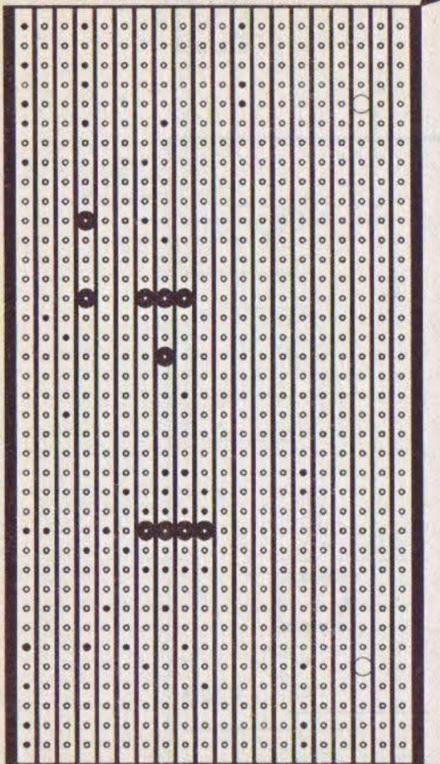
Fig.2.34 The underside view of the track "cleaner" board
