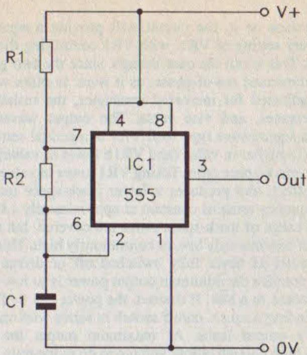
*Fig.1.14 The circuit for a basic 555 astable*
