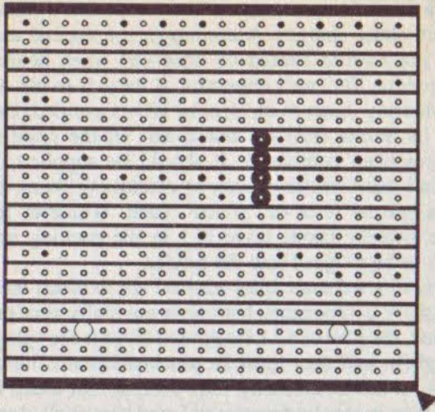
*Fig.1.7 The underside of the constant voltage controller board*
