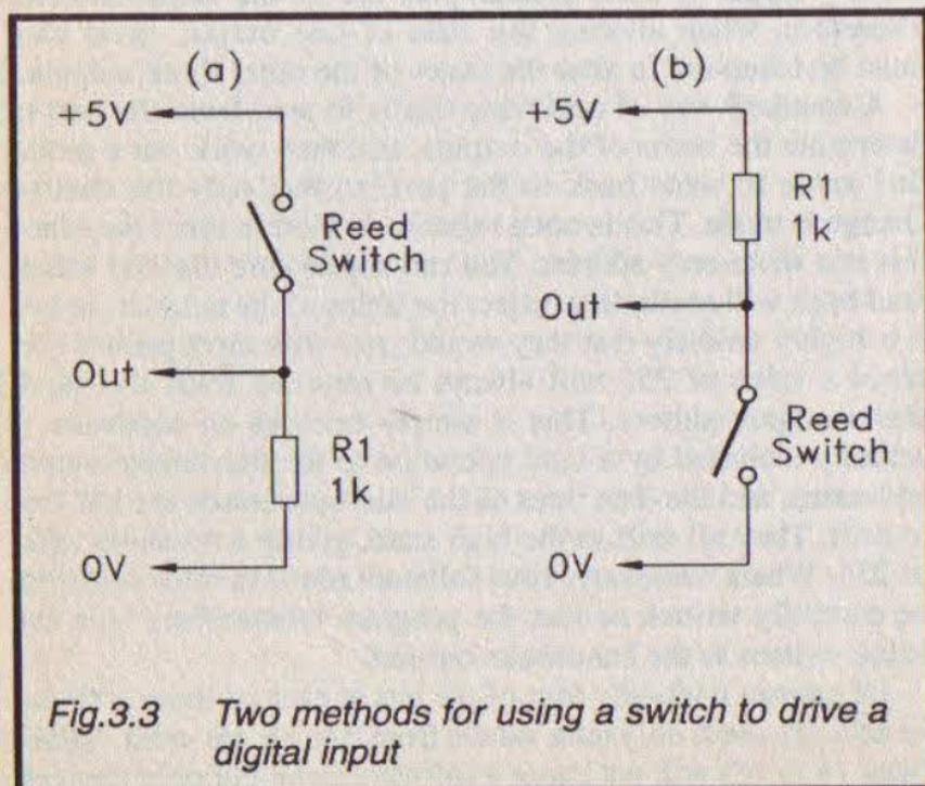
*Fig.3.3 Two methods for using a switch to drive a digital input*
