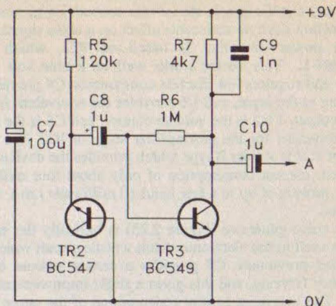
*Fig.2.25 The noise generator stages of the chuffer circuit*
