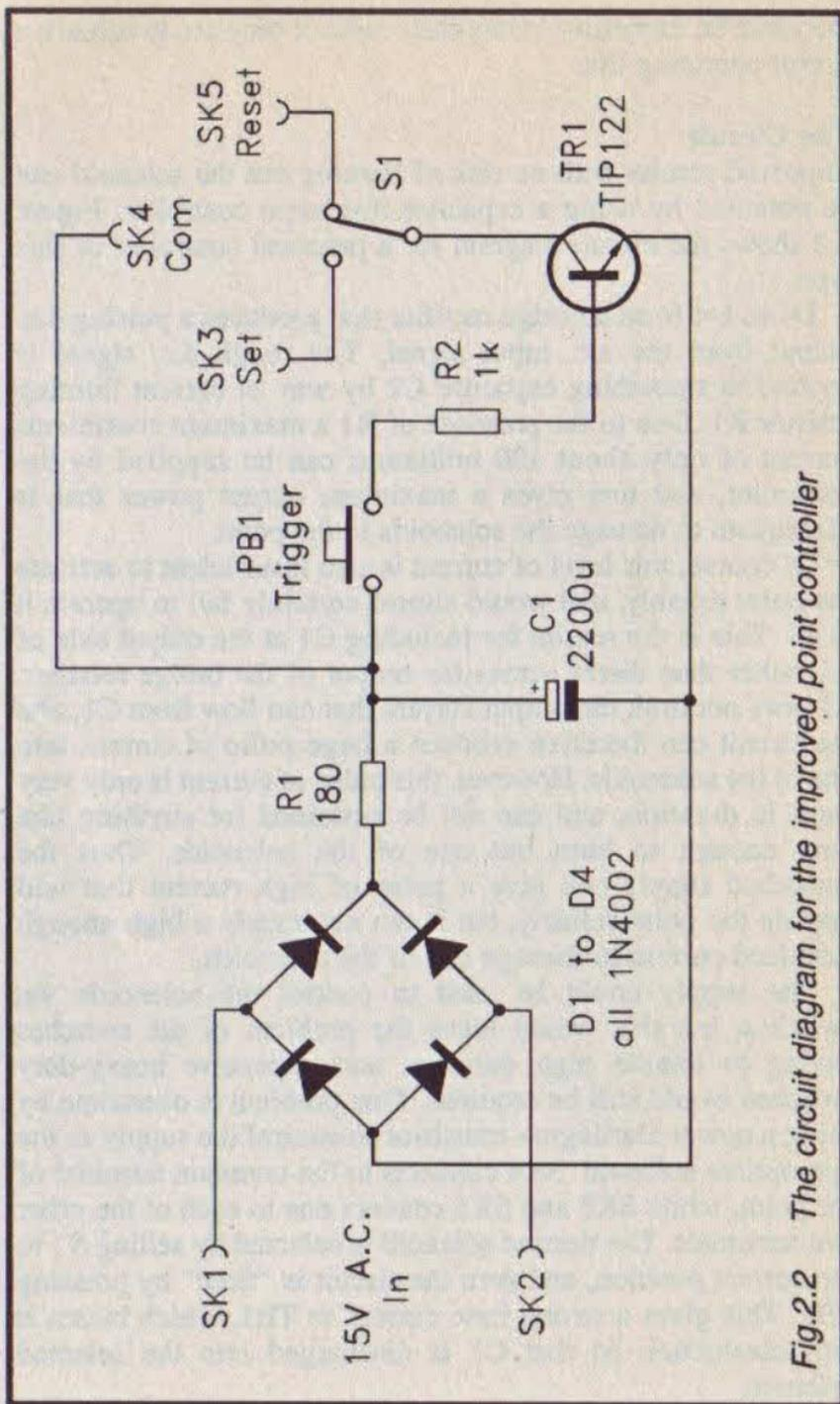
Fig.2.2 The circuit diagram for the improved point controller
