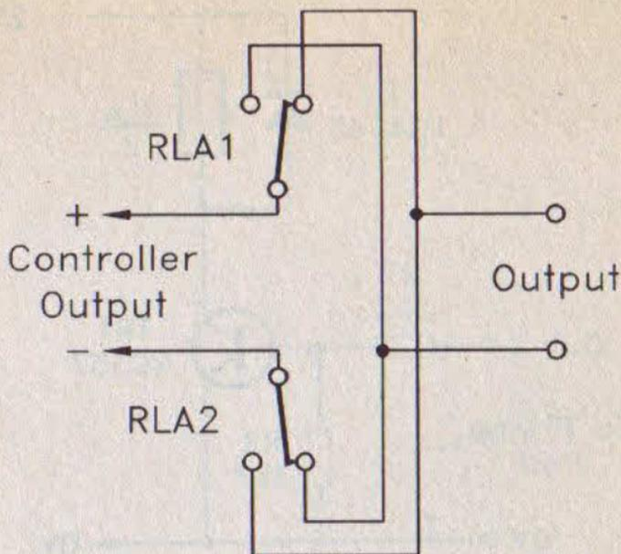
*Fig.3.11 Using a pair of c.o. relay contacts to provide direction control*
