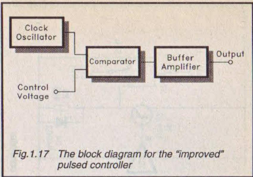
*Fig.1.17 The block diagram for the "improved" pulsed controller*
