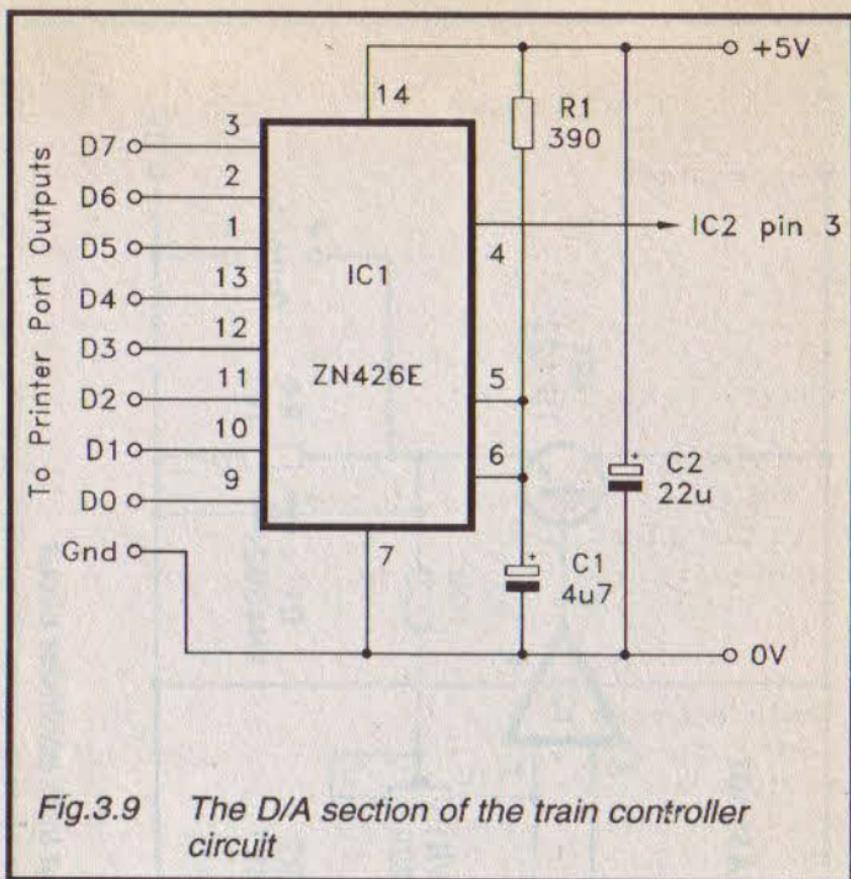
*Fig.3.9 The D/A section of the train controller circuit*
