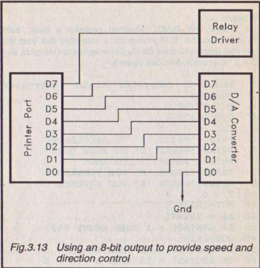
*Fig.3.13 Using an 8-bit output to provide speed and direction control*
