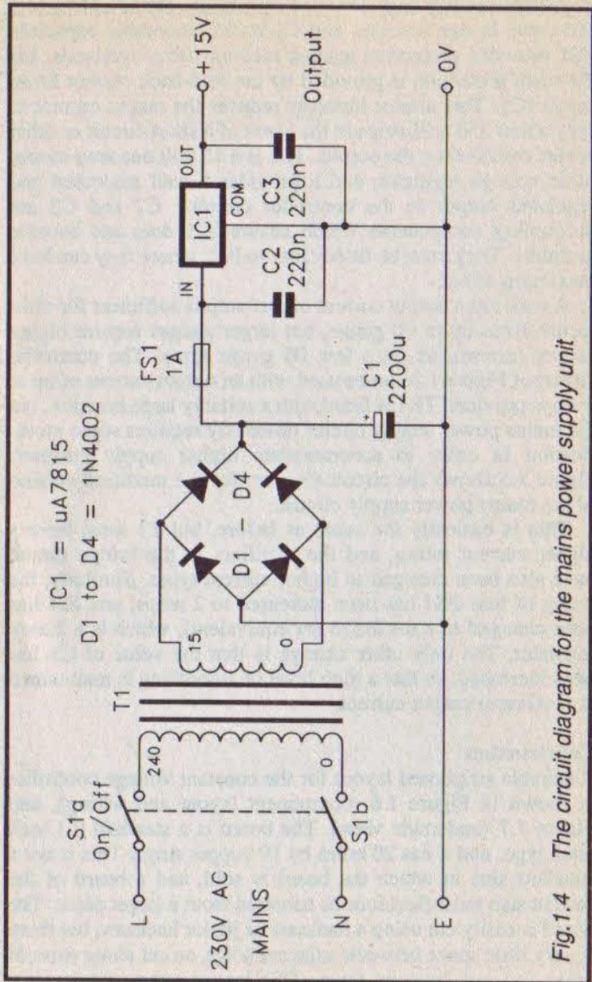
Fig.1.4 The circuit diagram for the mains power supply unit
