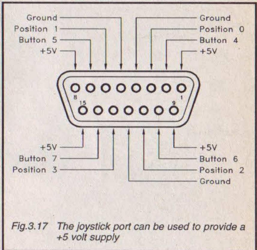
*Fig.3.17 The joystick port can be used to provide a +5 volt supply*
