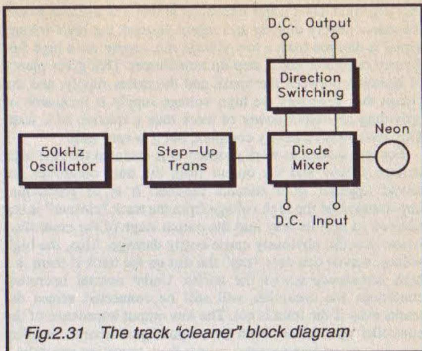
*Fig.2.31 The track "cleaner" block diagram*
