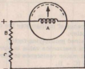
(f) To find ohmage value of unknown resistance by means of milliammeter and battery.
