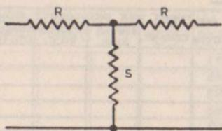
75 ohm Feeder - "T" Section.
