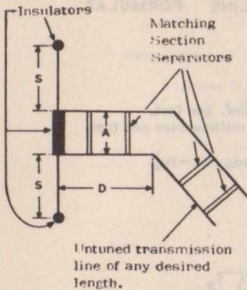
The dimension A depends upon the aerial impedance and the impedance of the transmission line and the impedance in ohms of the matching section is equal to
