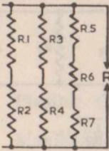
$R = \frac{I}{\frac{I}{R_1+R_2} + \frac{I}{R_3+R_4} + \frac{I}{R_5+R_6+R_7}}$      | <p style="text-align: center;"><b>CONDENSERS</b><br/>IN SERIES—PARALLEL</p>
