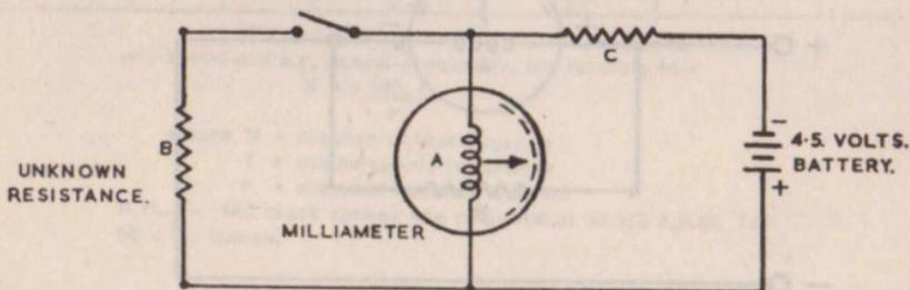
(g) To find ohmage value of unknown resistance by means of milliammeter, battery and any known resistor.
