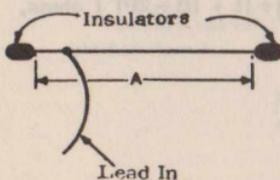
$$A = (164 \times \text{Number of half waves on the aerial minus } .05) \div (\text{Frequency in Megacycles}) \text{ yds.}$$
