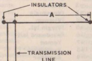
$$A = [164 (\text{Number of Half Waves on the Aerial Required, Minus } .05) \div (\text{Frequency in Megacycles of most used brand})] \text{ yds.}$$
