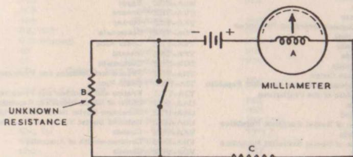
(h) To find the direct current resistance in ohms of an unidentified voltmeter or milliammeter.
