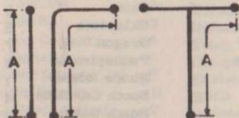
$$A = (\text{Wavelength in metres} \div 4) \times 1.094 \text{ yds.}$$
