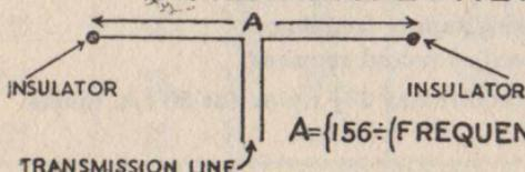
$$A = \left\{ 156 \div \left( \text{FREQUENCY IN MEGACYCLES} \right) \right\} \text{ YDS.}$$
