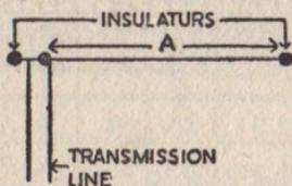
$$A = \left[ \left\{ 164 \left( \text{NUMBER OF HALF WAVES ON THE AERIAL REQUIRED, MINUS } \cdot 05 \right) \div \left( \text{FREQUENCY IN MEGACYCLES OF MOST USED BAND} \right) \right\} \right] \text{ YDS.}$$
