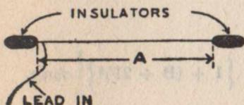
$$A = \left[ \frac{164 (\text{NUMBER OF HALF WAVES ON THE AERIAL MINUS } 0.5)}{\text{FREQUENCY IN MEGACYCLES}} \right] \text{ YDS.}$$
