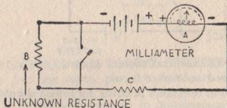
(h) To find the direct current resistance in ohms, of an unidentified voltmeter or milliammeter.
