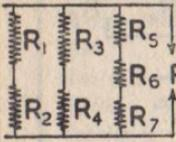
$R = \frac{1}{\frac{1}{R_1 + R_2} + \frac{1}{R_3 + R_4} + \frac{1}{R_5 + R_6 + R_7}}$ | <p style="text-align: center;"><b>CONDENSERS<br/>IN SERIES-PARALLEL</b></p>
