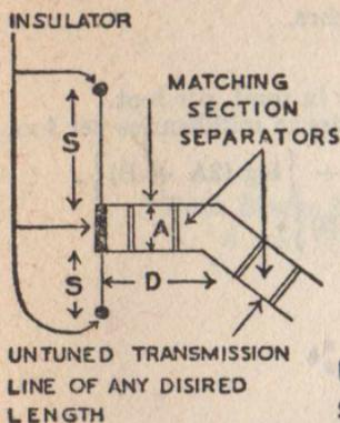
THE DIMENSION **A** DEPENDS UPON THE AERIAL IMPEDANCE AND THE IMPEDANCE OF THE TRANSMISSION LINE AND THE IMPEDANCE IN OHMS OF THE MATCHING SECTION IS EQUAL TO
