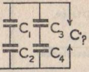
$C = \frac{1}{\frac{1}{C_1 + C_2} + \frac{1}{C_3 + C_4}}$ |
