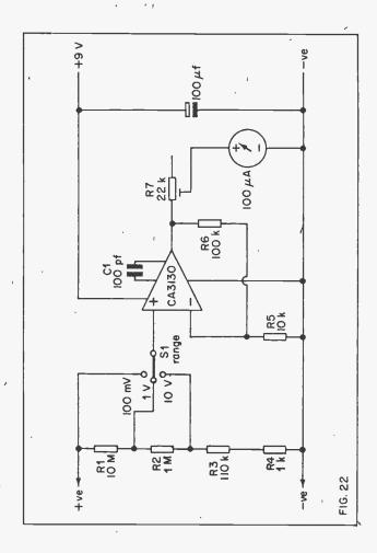
It is an interesting feature of this circuit that it does not need to be powered from a dual balanced power supply. It operates perfectly well from a single supply of 9 valts. The reason for this is that the CA3130 will provide an output that can swing to within a few millivolts of either supply rail, provided the output is only lightly loaded, as it is here. Thus under quiescent conditions the voltage across the meter is insignificant, and it will read zero.
