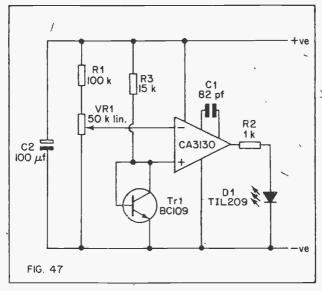
phase shift, which brings the inverting input and the output into phase, and the circuit thus oscillates at the operating frequency of the phase shift network. With the specified values the circuit oscillates at approximately 1kHZ.
