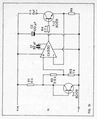
The second advantage is that with this circuit there is not output voltage drop when the unit is passing output currents a little below the threshold level. The output current threshold is so well defined that it is not really possible to significantly improve upon the circuit in this respect.
