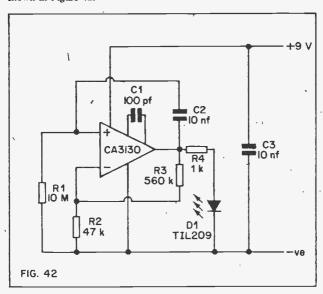
This circuit is very similar to those of the Continuity Tester and Metronome which appear in Figures 30 and 31 respectively, in this book. It is a non-inverting, D.C. amplifier with positive feedback between its output and input. It briefly switches the L.E.D. on at approximately one second intervals. The average current consumption of the unit is only about 2.5 mA.
