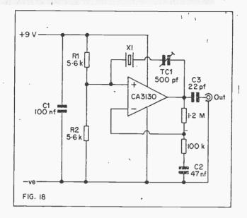
apart, with the series resonant one being the lower of the two. At the parallel resonant frequency the crystal exhibits a very high impedance and at series resonance it has a very low impedance. At other frequencies a crystal has a fairly high impedance.
