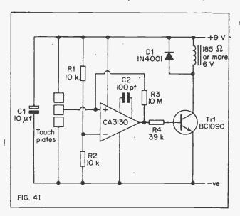
divider network formed by R1 and R2. The non-inverting output is fed from the output of the I.C. via R3, and it will therefore remain at virtually earth potential. Thus at switch on the output of the I.C. is low, and Tr1 receives no significant base current. Tr1 is cut off and the relay is energised.
