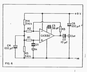
capacitor. D.C. blocking capacitors are needed at the input and output, and these are C1 and C3 respectively.
