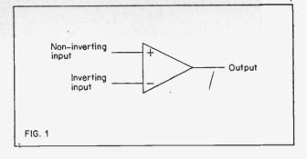
In a few switching applications this full gain is required, but in all circuits needing linear amplification, this gain is greatly reduced by the application of negative feedback.
