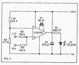
circuit thus provides the necessary action, as if either or both the P.L.I. outputs are high, D1 comes on.
