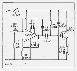
This circuit is based on the continuity tester circuit just described. However, the circuit values have been adjusted to provide a much slower rate of oscillation, and by enabling the time constant of the feedback circuitry to be varied, the oscillation frequency is made variable. VR1 can be adjusted to produce any beat rate from about 50 beats per minute to over 200 beats per minute.
