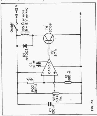
VR1 is adjusted so that under normal conditions there is a higher voltage at the inverting input than there is at the non-inverting input. This causes the output of the I.C. to be normally low, with Tr1 cut off and no significant current flowing through the relay coil.
