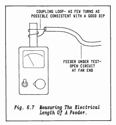
tuned from its lowest frequency upwards until a dip is noted. This frequency should be noted as it is the primary resonant frequency. However, it is wise to check this by tuning further
