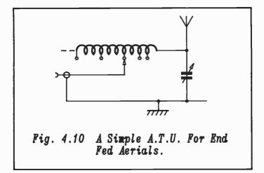
variable capacitor should be up to about 500 pF although this is by no means critical. However, if it is to be used for transmitting it should be a widespaced one. The coil should be an inch or two in diameter and it should have fifty turns or more of 16 s.w.g. wire or thicker, depending upon the bands likely to be used. Taps should be placed along the winding, spaced every turn or so at the beginning, but spaced out more further along its length.
