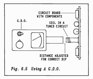
As a rough guide a distance of about a centimetre can be expected if the coil has a large number of turns. If it only has a few then the G.D.O. coil may have to be placed over the tuned circuit under test. However, with a little experience it soon becomes obvious how much coupling is required.
