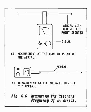
coupling can be obtained the best way is to short out the feed point and place the coil as close as possible to the aerial as shown in Figure 6.6. Using the method shown in Figure 6.6(a) the best dip will be obtained at a current maximum, i.e., at the feed point of most aerials. If the method of Figure 6.6(b) is used then the best dip will be obtained at a point of voltage maximum. This can always be found at the end of an aerial.
