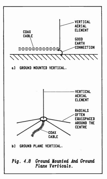
on the installation of a ground mounted vertical.
