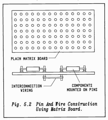
Although this method of construction does take longer to build it does afford much more flexibility than stripboard. This means that sensitive leads can be kept short and the circuit can be arranged more easily as required. Also earth leads can be made thicker if needed. Even so it does have its shortcomings and is certainly not ideal for use above 30 MHz.
