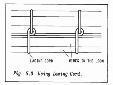
The wires should be carefully laced together. The cord should be run along the length of the loom and tied at intervals of an inch or so as shown in Figure 5.3. The exact spacing is not critical but will depend to some extent on the number of wires in the loom and the control which is needed for the wires.
