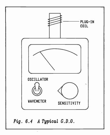
when the oscillator is tuned to the resonant frequency of the tuned circuit under test.
