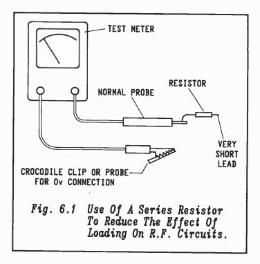
reduce the value of any stray capacitance. Even so the presence of the resistor may well affect the circuit slightly and this should be borne in mind when taking measurements.
