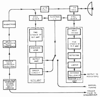
Fig. 9.—Transmitter-receiver—block diagram.
