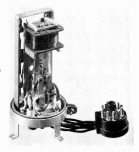
The work so far undertaken permits the construction of efficient power packs in the range of a few milliwatts working from a 1.5-V battery to 250 W on a 24-V battery. In constructing a power pack it must be remembered that the vibrator is essentially a current device.
