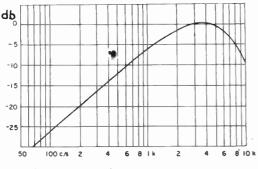
Fig. 2.—L.C. tape characteristic at 15 in per sec.
