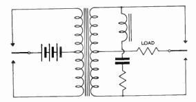
Fig. 10.- Parallel commutating circuit. Rectified load.
