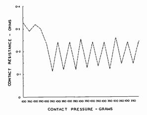
Fig. 1.—Relation between contact resistance and contact pressure.
