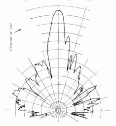
Fig. 6.—Vertical polar diagram with maximum tilt.
