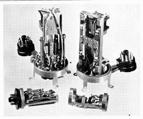
Fig. 13.—Methods of mounting vibrators.
