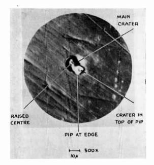
Fig. 4.—Shadow photograph of cathode contact after a single break at 1.5 V, 28 A.
