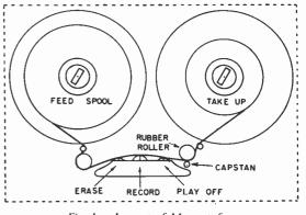
Fig. 1.—Layout of Magnetofon.
