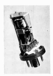
Fig. 14 (above, left).—Low-power (30 mW) vibrator.
