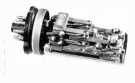
Fig. 17 (left).—Cleaned-up version of A.M. Type 14 vibrator (X331).
