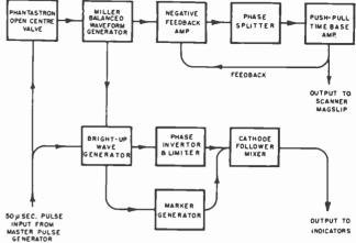
Fig. 10.—Synchronizer unit—block diagram.
