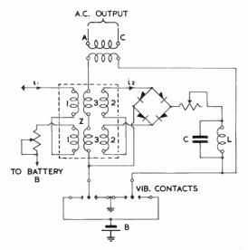
Fig. 11.—Power pack regulated by a saturable reactor in primary circuit.
