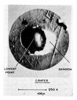
Fig. 5.—Shadow photograph of anode contact after 180,000 operations at 6 V, 1 A.
