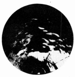
Large sections of coastal routes such as Karachi-Bahrein were flown at night using the radar as the prime navigational aid, and approaches to marine airports were particularly easy. An example is shown in Fig. 16, where a breakwater (not shown on the map) together with responses from vessels in the harbour can be clearly distinguished.
