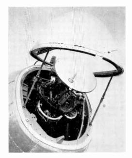
Fig. 3.—Scanner installed in nose of Viking with radome open.
