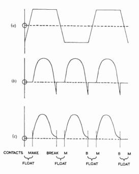
Fig. 8.—Voltage and current waveforms for circuit of Fig. 7. (a) Buffered transformer, output voltage waveform, (b) input (d.c.) current waveform, undamped output circuit, (c) input (d.c.) current waveform, damped output circuit.
