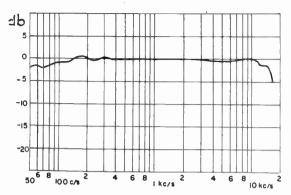
Fig. 6.—Overall frequency characteristic (L.C. tape).
