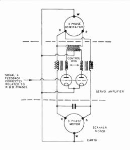
Fig. 7.—Simplifier servo amplifier unit.
