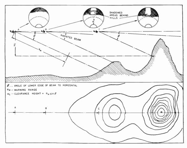
Fig. 2.—High ground warning by the safety circle technique.
