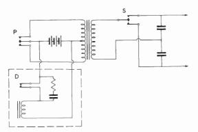
Fig. 2.—Split reed, separately-driven vibrator power pack.
