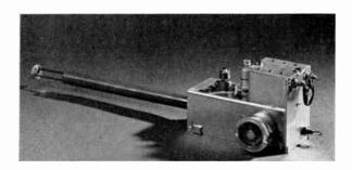
Fig. 5. Mechanical construction of the circuit of Fig. 4, showing the coaxial input, the tuned line, the variable resistor to set emitter current, the input trimmer, and the measured transistor.
