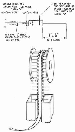
Fig. 7. Dimensional and packaging requirements for the components.
