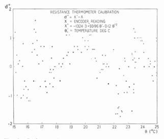
Fig. 6. Resistance thermometer calibration—deviation from linear plus square law.
