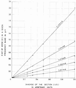
Fig. 3. Relation between noise and cross-section.
