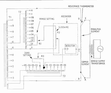
Fig. 3. Resistance thermometer bridge circuit.
