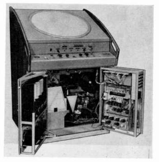
Fig. 7. A shipborne relative motion bright display console.
