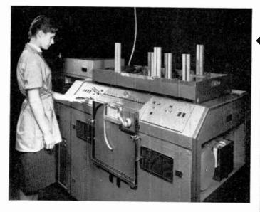
The printed circuit cards used in the control computer can be easily removed and the rack itself can be tilted and withdrawn on telescopic runners for inspection purposes.
