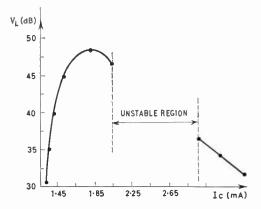
Fig. 6. Power amplification plotted against emitter current for an operating frequency of 350 Mc/s for the transistor AF 106. The region between the dashed lines represents unstable i.f. operating conditions.
