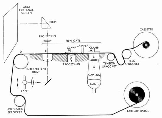
Fig. 1. Schematic representation of the 35 mm rapid photographic processor and projector.
