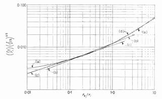
Fig. 1. The beam parameter, normalized screen distance  $\times \sqrt{\text{perveance}}$ , shown as a function of the normalized spot radius. (a) From exact solutions of the space-charge equations (1) and (2).
