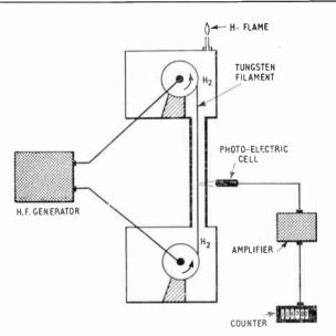
Fig. 1. Automatic test equipment for tungsten filaments employing an invisible crystal-cleavage searching technique.
