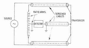
Fig. 2. Circuit to reduce ratio arm lead capacitance.
