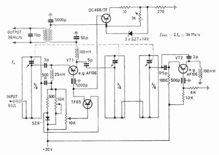
Fig. 8. The circuit of an experimental u.h.f.-tuner covering 400 Mc/s to 1200 Mc/s (or higher) using coaxial tuning elements. The input frequency is converted by a pump oscillator operating in the transit-time mode to an output i.f. of 36 Mc/s. The first coaxial cavity is  $\lambda/2$  to the oscillator frequency and  $\lambda/4$  to the input frequency.
