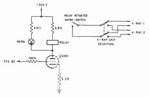
Fig. 8. X-ray unit control.
