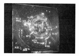
Fig. 4. An air surveillance radar picture on a semi-transparent screen which is edge illuminated to show up the annotation on the back of the screen.
