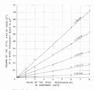
Fig. 2. Relation between noise and total resistance.
