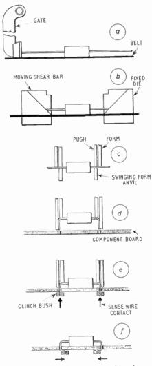
Fig. 5. Stages in component insertion.
