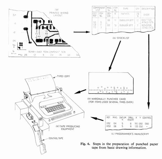
After the first few boards of a batch are completed the possibility of finding an out-of-tolerance component is reduced since items (a) and (b) above have been checked.
