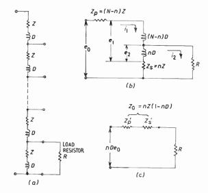
Fig. 4. Equivalent circuits for the ratio transformer.
