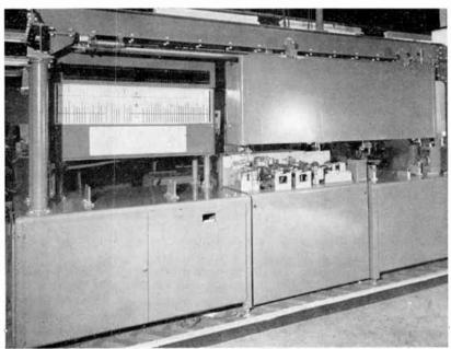
Fig. 2. Three-stage transfer multi-dimension crankshaft inspection machine.
