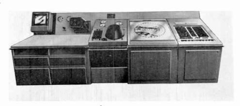
Fig. 8. The navigational console on the P & O-Orient liner S.S. Canberra.
