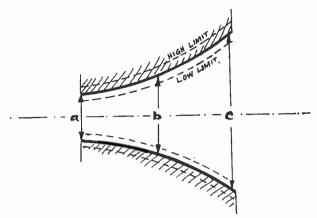
Fig. 6. Interdependent inspection example: measurements on a nozzle curvature.
