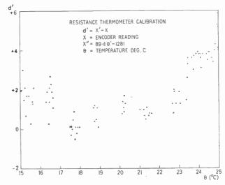
Fig. 5. Resistance thermometer calibration—deviation from linear law.
