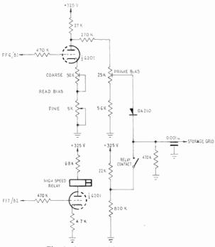
Fig. 6. Storage-grid bias switching.
