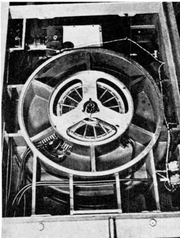
(e) Rotary Inductosyn *in situ* in machine shown in Fig. 5.
