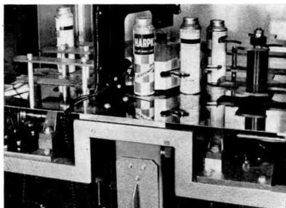
Fig. 4. Handling mechanism used with the check weigher.
