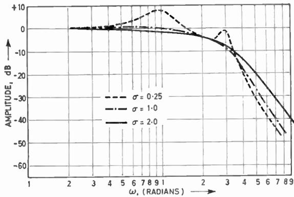
Fig. 6.  $N = 4$  In-line pole amplitude response.
