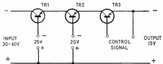
Fig. 3. Use of transistors TR1 and TR2 as pre-regulators.
