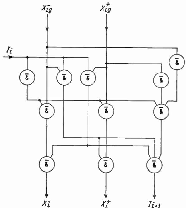
Fig. 2. Code conversion logic for a single binary-coded three-valued digit pair.
