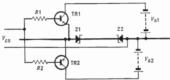
Fig. 19. Common-collector circuit using complementary transistors.
