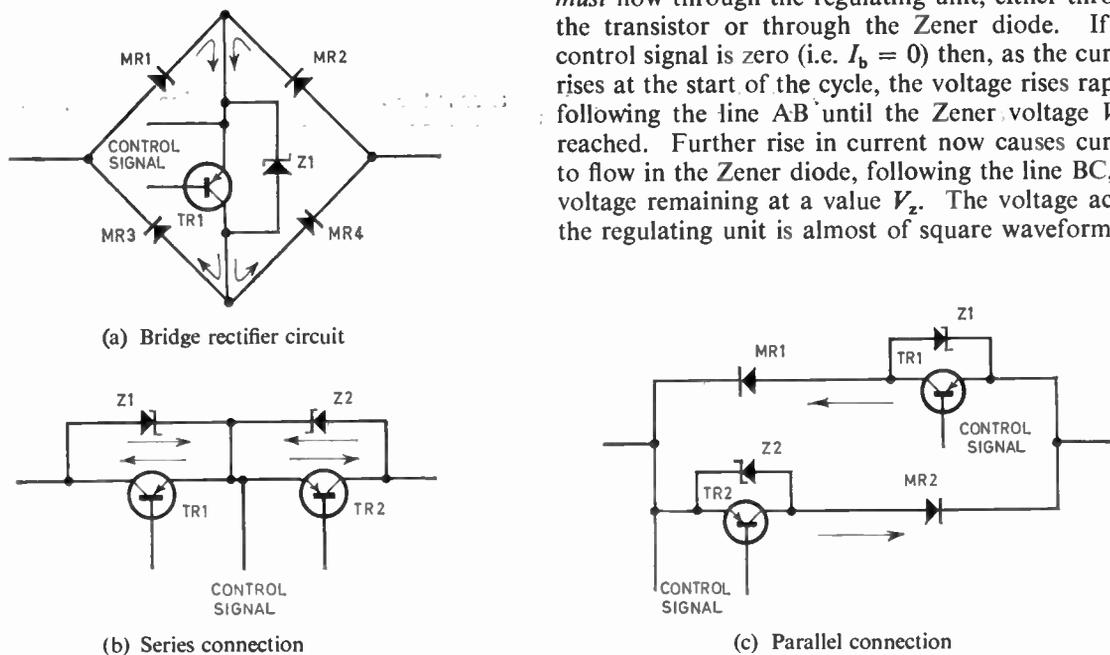
Fig. 6. Methods of connecting transistors in a.c. regulating units.
