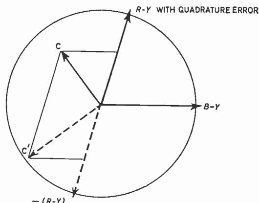
Fig. 11. The effect of a quadrature error in a PAL coder.
