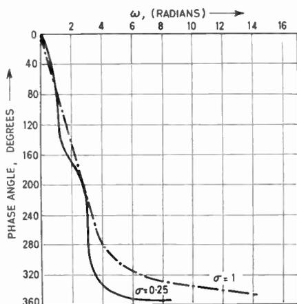
Fig. 4.  $N = 4$  In-line pole phase response.
