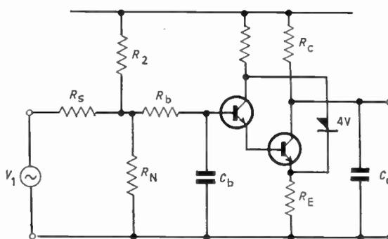
Fig. 11. Circuit diagram showing two active devices connected as a Darlington pair to generate a higher input impedance and higher voltage gain.
