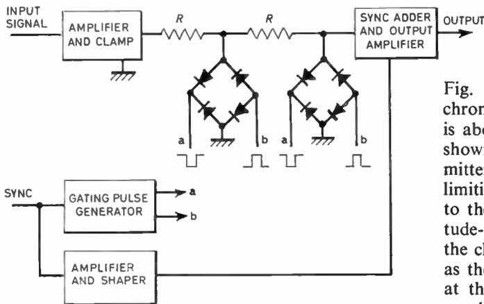
Fig. 6. Stabilizing amplifier.
