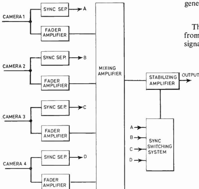
Fig. 5. Schematic of a 'knob-a-channel' type of mixer.
