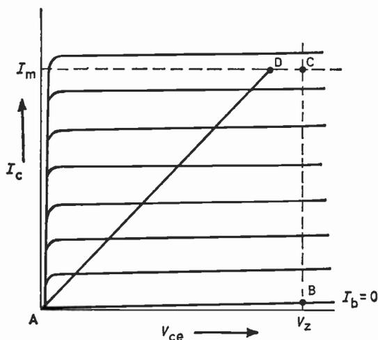
Fig. 9. Common-emitter characteristics and operating line with a.c. control signal.
