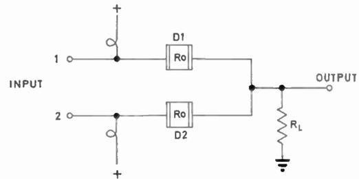
Fig. 5. Comparator circuit of two Gunn diodes in parallel.
