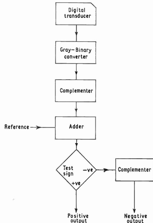
Fig. 1. Schematic arrangement of a typical digital position indicator.
