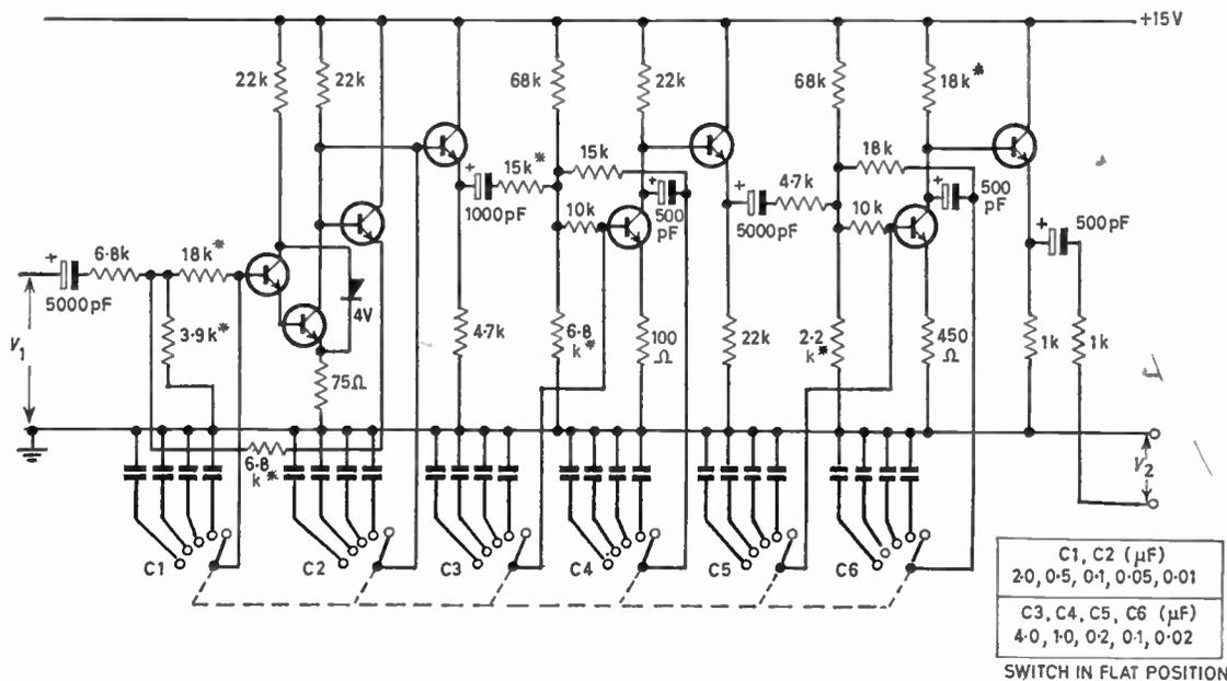
Fig. 12. Circuit diagram of the *N* = 6 in-line pole filter. \* shows high-stability type resistors.
