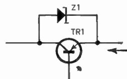
Fig. 5. Use of Zener diode to limit the voltage across the regulating unit.
