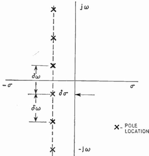
Fig. 1. The in-line pole distribution.
