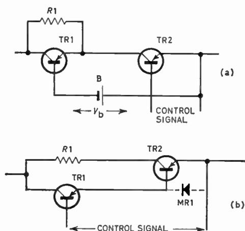
Fig. 4. Regulating units consisting of two transistors and a resistor for increased power.
