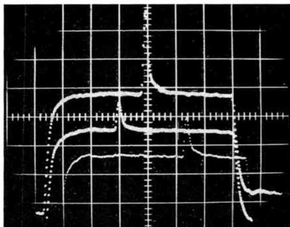
(b) Typical waveforms produced by the circuit of Fig. 7(a) horizontal scale: 10 ns/div; vertical scale: 10 V/div.
