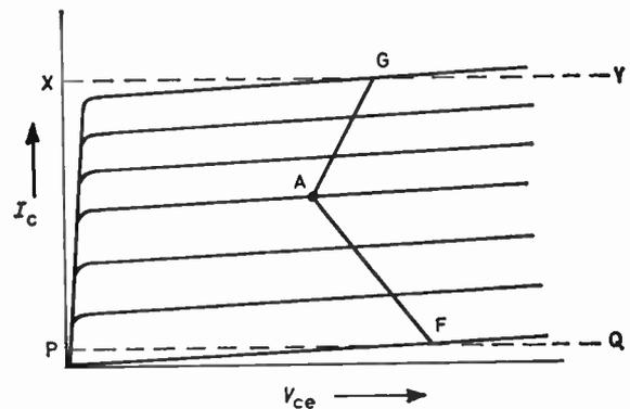
Fig. 13. Operating line for class-A common-emitter circuit showing serious distortion.
