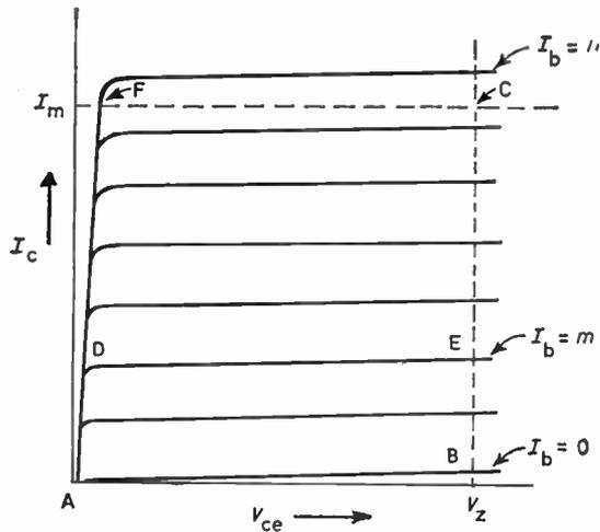
Fig. 7. Characteristics of a transistor in common-emitter configuration.
