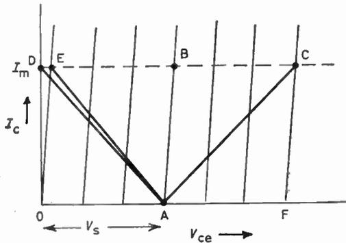
Fig. 23. Operating conditions of transistor with equal buck and boost voltages.
