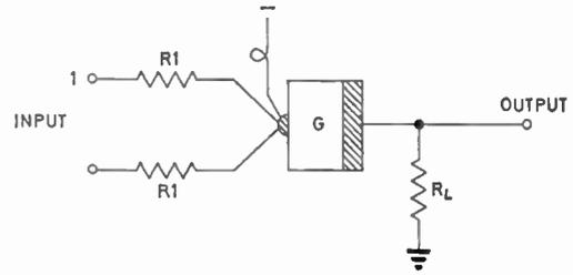
Fig. 9. A Gunn-effect AND circuit.
