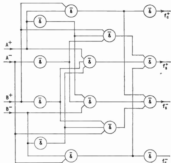
Fig. 4. Logic diagram of half-adder using NAND connectives.
