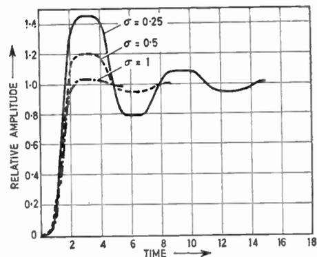
Fig. 8.  $N = 4$  In-line pole step response. Step height = 1.0.
