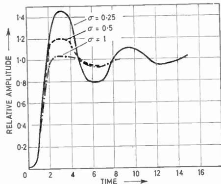
Fig. 9.  $N = 6$  In-line pole step response. Step height = 1.0.
