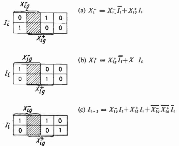
If it is assumed that NAND operators are used to construct these functions, the expressions for  $X_i^-$  and  $I_{i-1}$  can be written in the following form:
