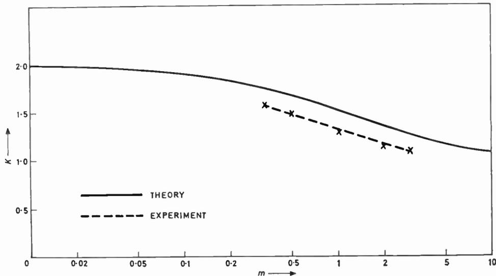
Fig. 6. Threshold ratio,  $K$ , as a function of  $m = R_0/R_L$  for the circuit of Fig. 5.
