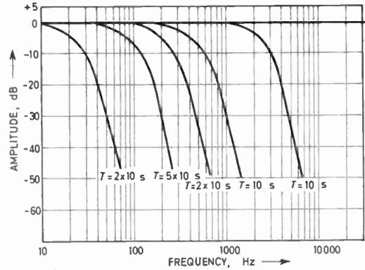
Fig. 14. Curves of  $N = 6$ ,  $\delta = 1$  in-line pole filter.
