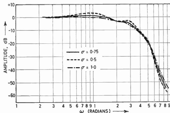
Fig. 3.  $N = 6$  In-line pole amplitude response.
