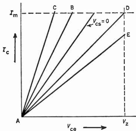
Fig. 10. Operation conditions with common-collector configuration and a.c. control signal.
