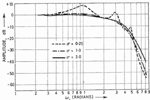
Fig. 7.  $N = 6$  In-line pole amplitude response.
