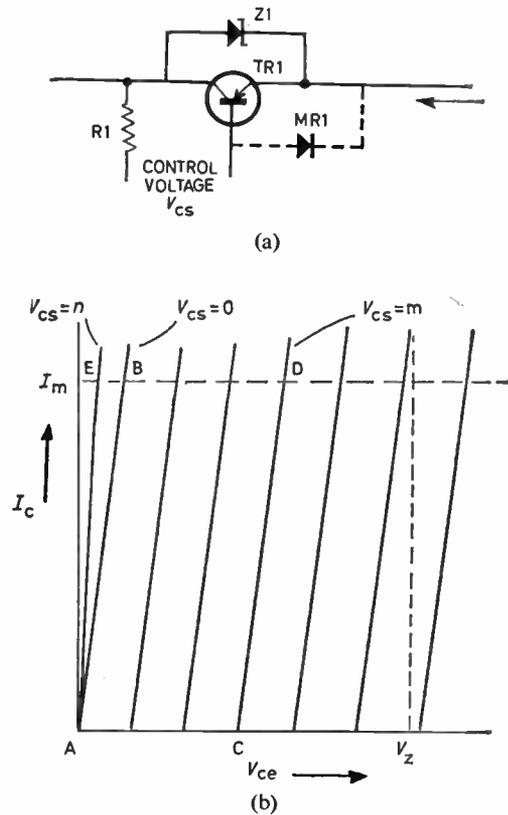
Fig. 8. (a) Common-collector circuit; (b) common-collector characteristics.
