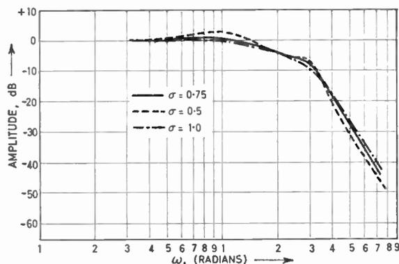
Fig. 2.  $N = 4$  In-line pole amplitude response.
