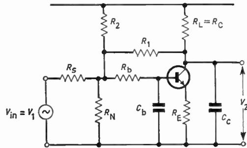
(c) Circuit diagram showing the connection details of a transistor for the generation of conjugate pole-pairs.
