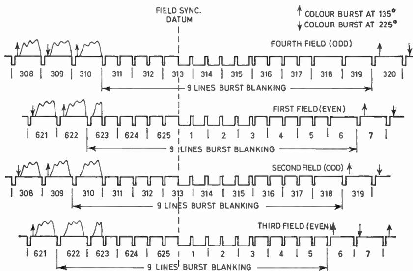
Fig. 2. Burst blanking.
