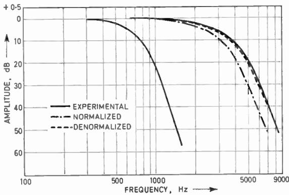
Fig. 13. Curves of  $N = 6$ ,  $\delta = 1$  in-line pole distribution.
