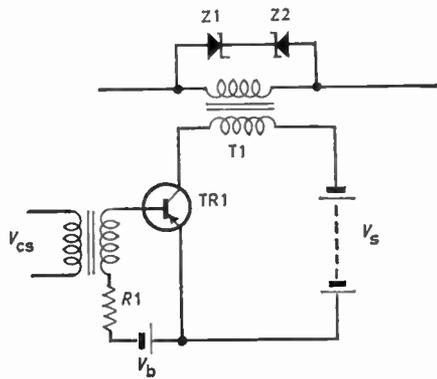
Fig. 11. Basic circuit for class-A operation using transformer; common-emitter configuration.
