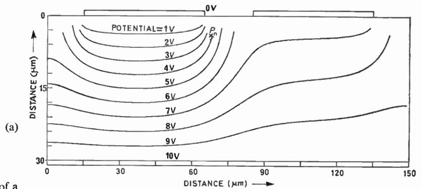
Fig. 4. (a) and (b) potential distribution of a Gunn-effect comparator.
