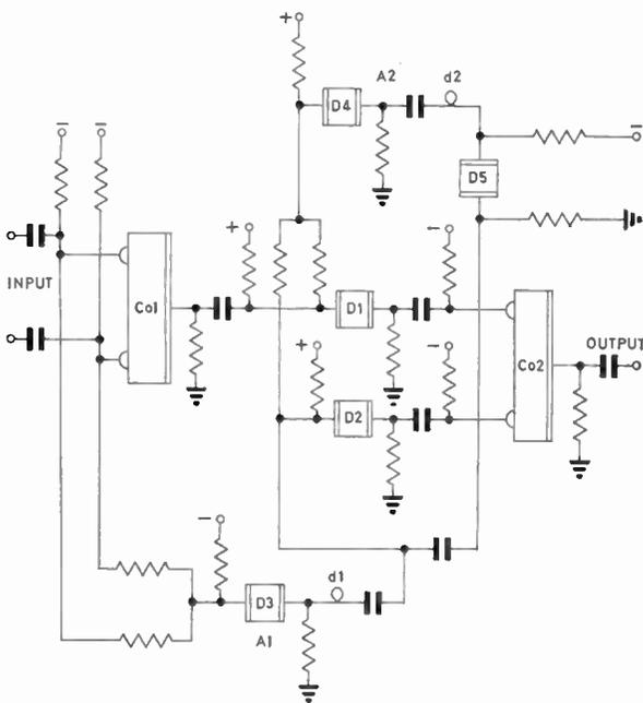
Fig. 10. Binary sequential adder.
