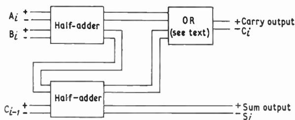
Fig. 3. Schematic arrangement of a full-adder.
