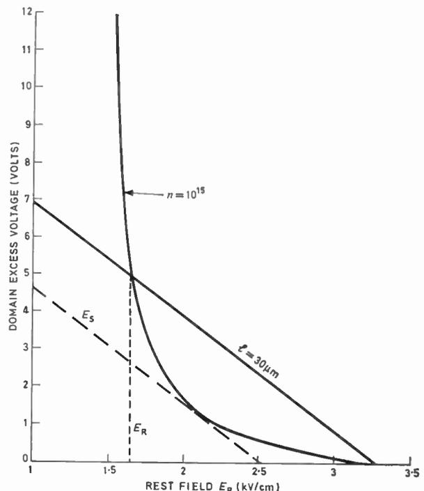
Fig. 1. Domain excess potential vs. rest field. (After Copeland.<sup>1</sup>)
