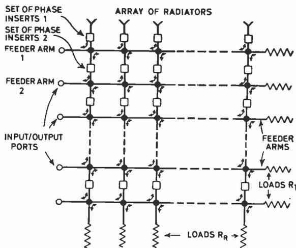
Fig. A. Schematic of Maxson multi-beam antenna.
