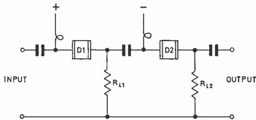
Fig. 2. Circuit of a two-stage amplifier.
