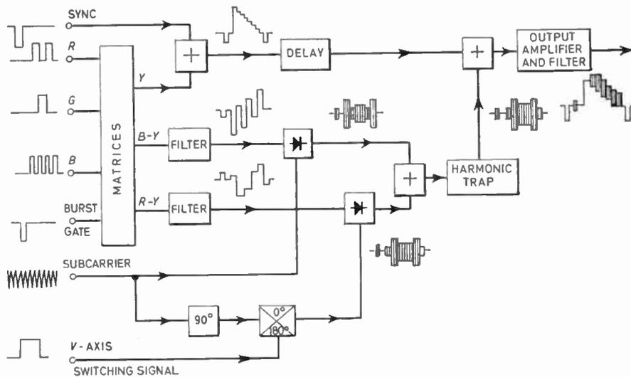
Fig. 3. Block diagram of a PAL coder.
