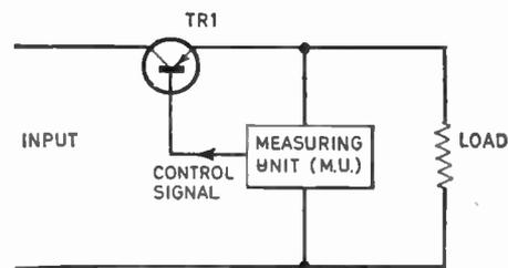
Fig. 1. Basic stabilizer circuit.
