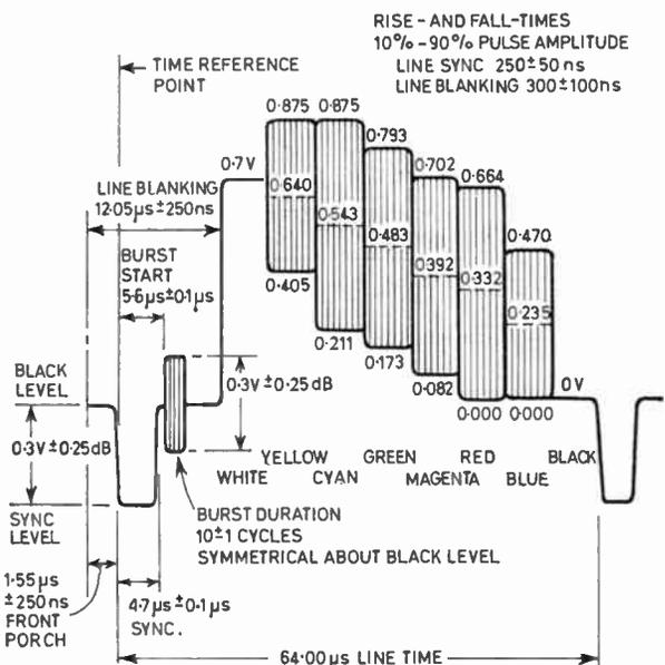
Fig. 7. 95% colour bars—line waveform.
