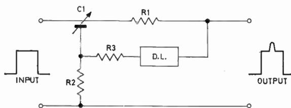
(a) Circuit for the production of a voltage spike, superimposed on a biasing pulse. DL = delay line.
