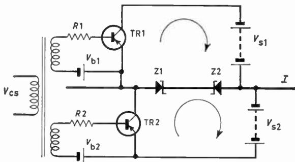
Fig. 14. Transformerless class-B common-emitter circuit.
