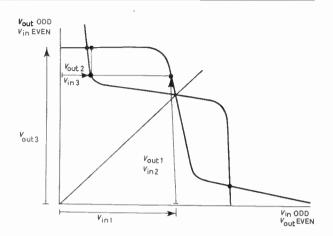
Fig. 10. Processing of a signal through a cascade of gates.
