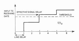
Fig. 4. Increase in signal delay time due to reflections.
