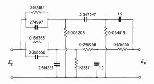
Fig. 2. Third-order rational transfer function network.
