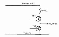
Fig. 7. 'Totem pole' output stage.
