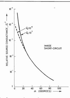
Fig. 9. Source conductance for narrow-band mixer using asymmetric diode.
