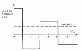
Fig. 5. Oscillations at input of receiving gate.
