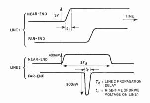
Fig. 3. Typical waveforms for system of Fig. 2, with matched lines.
