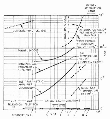
Fig. 1. Frequency band allocation, 'state of the art', and natural limitations based on Refs. 2, 3, 4.
