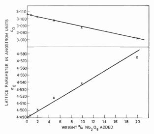
Fig. 1. Effect of additions of  $Nb_2O_5$  on the lattice parameters of  $RuO_2$  showing conformity to Vegard's law.
