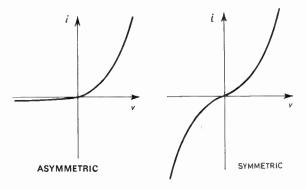
Fig. 2. Diode characteristics.
