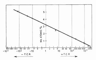
Fig. 2. Dependence of temperature coefficient of resistance (t.c.r.) on dopant level in host oxide.
