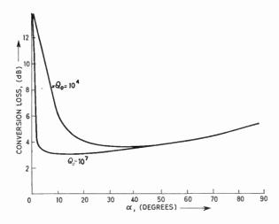
Fig. 10. Conversion loss of broad-band mixer using asymmetrical diode.
