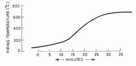
Fig. 3. Typical firing profile for ruthenium resistor glazes.
