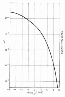
Fig. 2. Error probability in coherent p.s.k. system.  $\beta = \frac{E}{N_o}$  and  $P_o$  is the error probability per digit Note: In p.c.m. 1 digit = 1 bit of information
