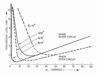
Fig. 8. onversion loss for narrow-band mixer using asymmetric diode.
