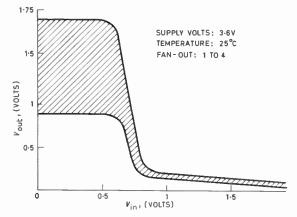
Fig. 8. Toleranced transfer characteristic for a RTL NOR/NAND gate.
