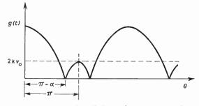
Fig. 3. Symmetrical diode conductance.  $(v_0 = V)$ .
