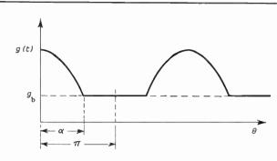
Fig. 7. Asymmetrical diode conductance.
