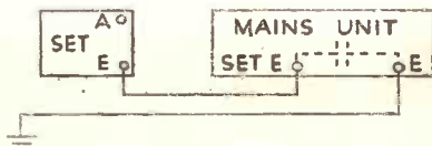
FIG. 17.—Essential safety condenser for the earth connection of a D.C. mains unit.
