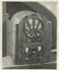
The Lumophon W.23 receiver is notable for its use of "direct coupling" which is stated to be very efficient.
