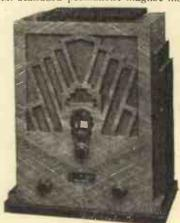
Double band pass tuning is employed in this three-valve British General set which can be examined on Stand No. 12a.
