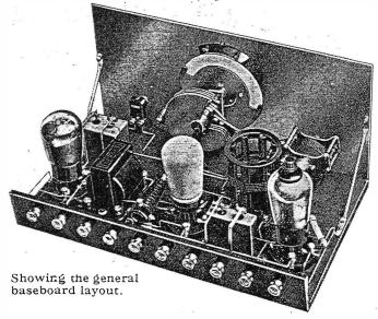
H.T. +1 should be 60-80 volts; H.T. +2, 40-60 volts; H.T. +3, 120 volts.
