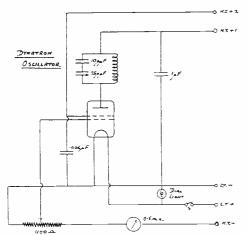
Showing the theoretical circuit. The valve should be Mazda S.G 215 with 2v.L.T. supply and H.T.+1,30-40 volts; H.T.+2,100 volts.
