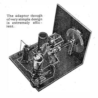
three leads from the adaptor terminals to the valve plug, for insertion into the detector valveholder of the set, should not be twisted together and must be of the shortest possible length. The lead from the terminal marked "To anode" is taken to the pin of the plug corresponding to the plate of the valveholder and the L.T.+ and L.T.— terminals to the two corresponding connections. Make sure that these two leads are not reversed.
