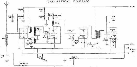
All connections marked  $\frac{1}{2}$  are taken to metal chassis for earth return.
