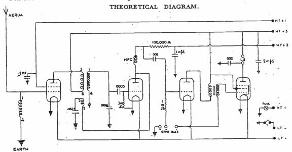
All connections marked  $\frac{1}{\equiv}$  are taken to metal chassis for earth return.
