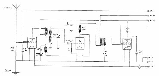
All connections marked  $\frac{1}{2}$  are taken to metal chassis for earth return.
