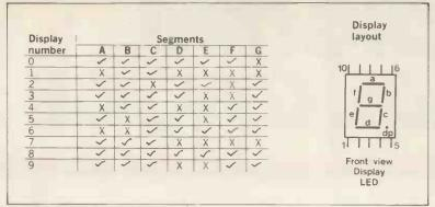
Figure 2. Display segment connection.
