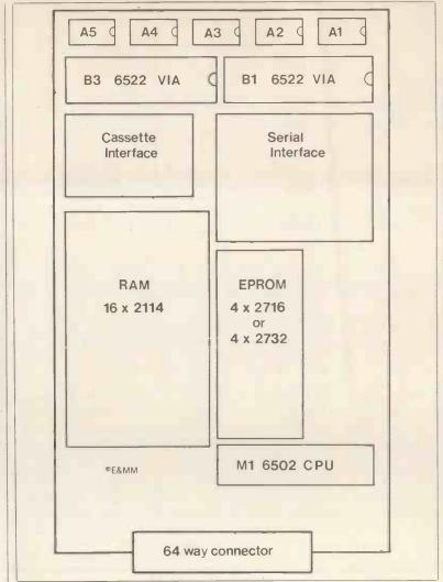
Figure 3. Simplified arrangement of controller card produced by Tangerine Computer
