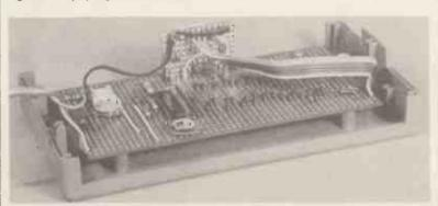
Component board and display board mounting.
