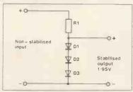
Figure 2. Example of a multiple diode shunt stabiliser circuit.
