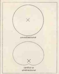
Figure 1. Microphone Polar diagrams.
