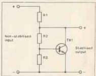
Figure 3. An 'amplified diode' regulator circuit using an NPN transistor.
