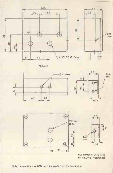
Figure 4. Case and bracket construction.
