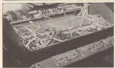
A large organ kit during assembly with wiring harnesses installed.
