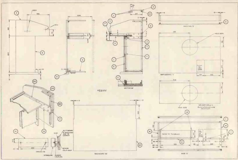
Figure 36. Cabinet construction details.
