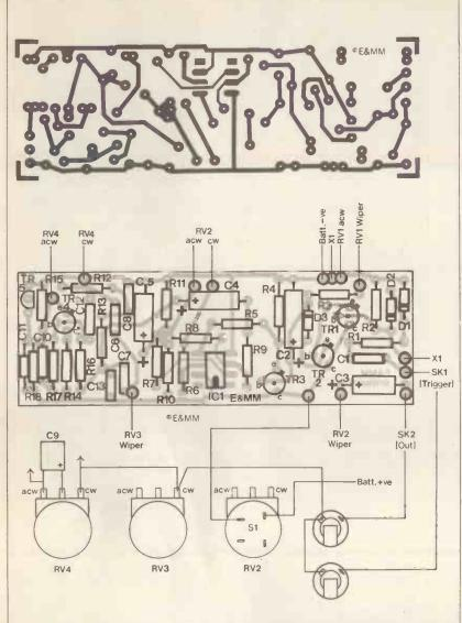
Figure 3. PCB track, component layout and wiring details.
