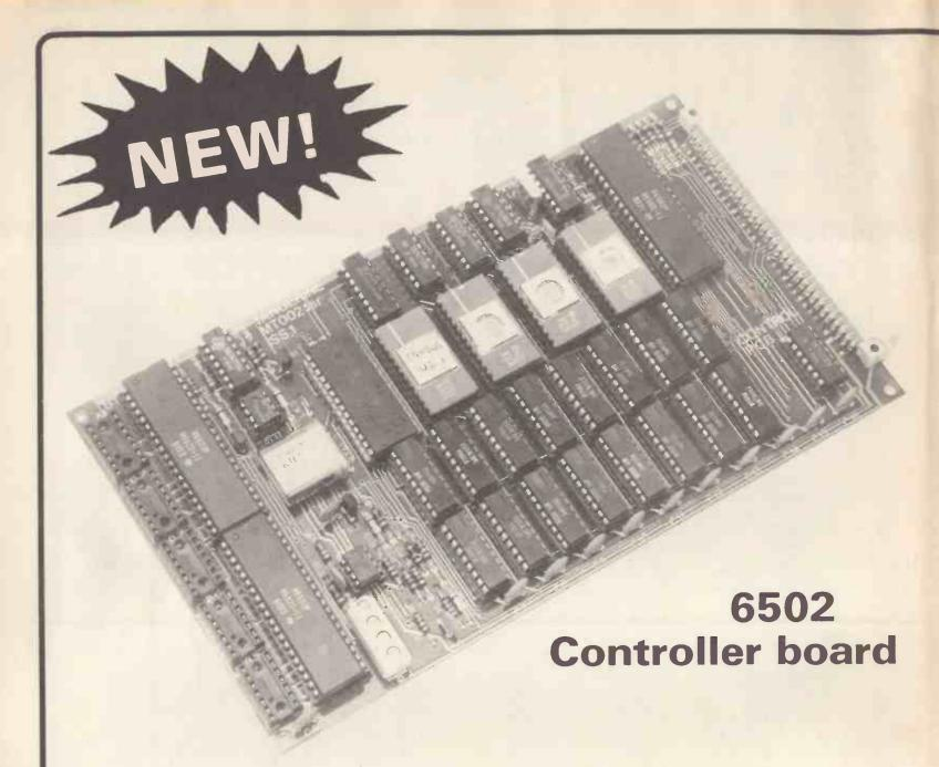
The 6502 Controller board has been designed to meet the needs of the O.E.M., but may also be considered by the serious enthusiast and laboratory engineers/technicians.
