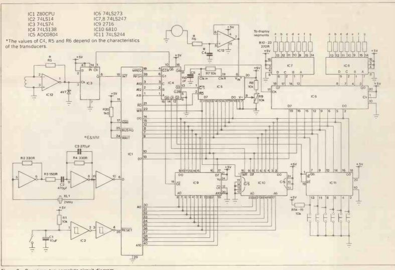
Figure 2. Car computer: complete circuit diagram.
