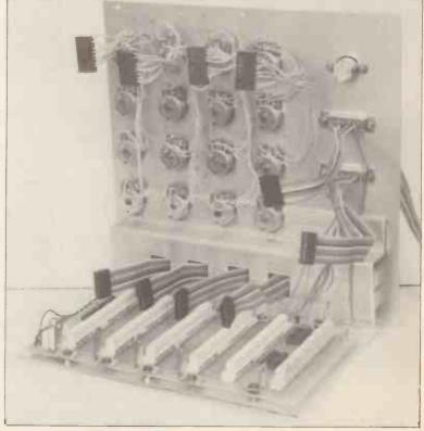
Motherboard and front panel wiring.
