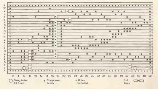
Figure 3. Wiring details and main board layout.
