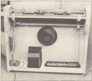
Rear view of cabinet with parts installed.
