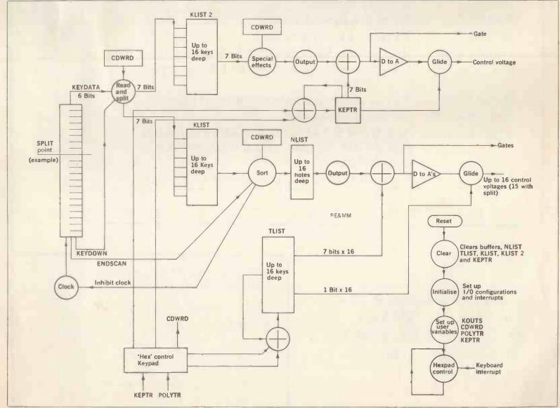
Figure 7. Block diagram of DIGI-1 program.
