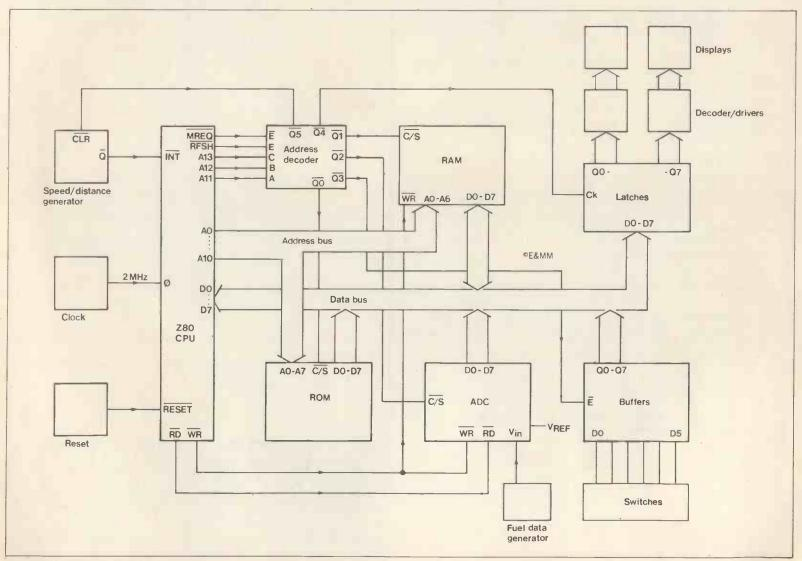
Figure 1. Car computer: block diagram.
