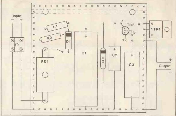
Figure 8. Veroboard layout for the car cassette power supply.
