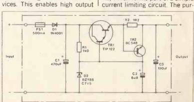
tion and only a small base | Figure 7. Circuit diagram of the car cassette power supply.
