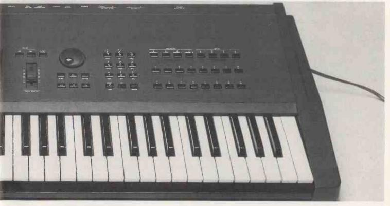
"Yamaha have taken advanced forms of their FM synthesis and AWM sample technologies, made them interactive and added digital filtering to each section."
