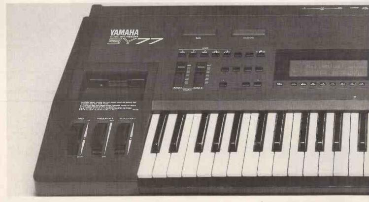
and AWM sample technologies (AFM and AWM2), made them interactive and added digital filtering to each section. The interactive bit means that you can use an AWM2 sample as a modulation input to any AFM operator (carrier or modulator), and/or use the AFM output as an AWM2 "sample". Yamaha call this Realtime Convolution and Modulation synthesis, but perhaps we can forgive them for that.
