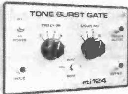
**TONE BURST GENERATOR** — This one won't access GB3LO but it's mighty fine for testing loudspeakers! The versatile unit will also test telephone channels and reverberation chambers, and can be modified for use as a 'silent switch' for A/B speaker testing.
