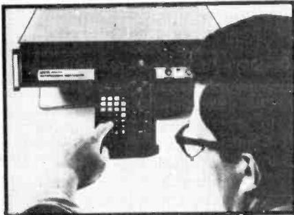
Both of the first models in the range to be announced (9015 and 9035) work to 100MHz in measuring frequency, period, period average, time interval, time interval average, frequency ratio and total count. Thanks to the microprocessor direct readout of preset operations, reciprocal calculations, and even answers in engineering units are easily achieved. 9-digit constants can operate on measurements through the keyboard.
