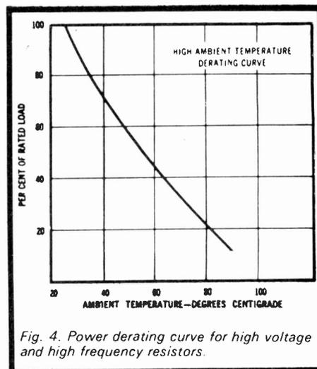
Fig. 4. Power derating curve for high voltage and high frequency resistors.
