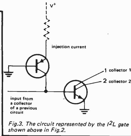
Fig. 3. The circuit represented by the I<sup>2</sup>L gate shown above in Fig. 2.
