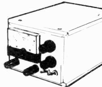
An invaluable piece of equipment for the enthusiasts workshop. This 3-30V d.c. power supply fulfills virtually all experimentation requirements. Avoid frustration and circuit damage with the variable current limit (0.1A max). Regulation typically better than 0.5% (max 3%). Ripple voltage typically better than 20mV (max 120mV).
