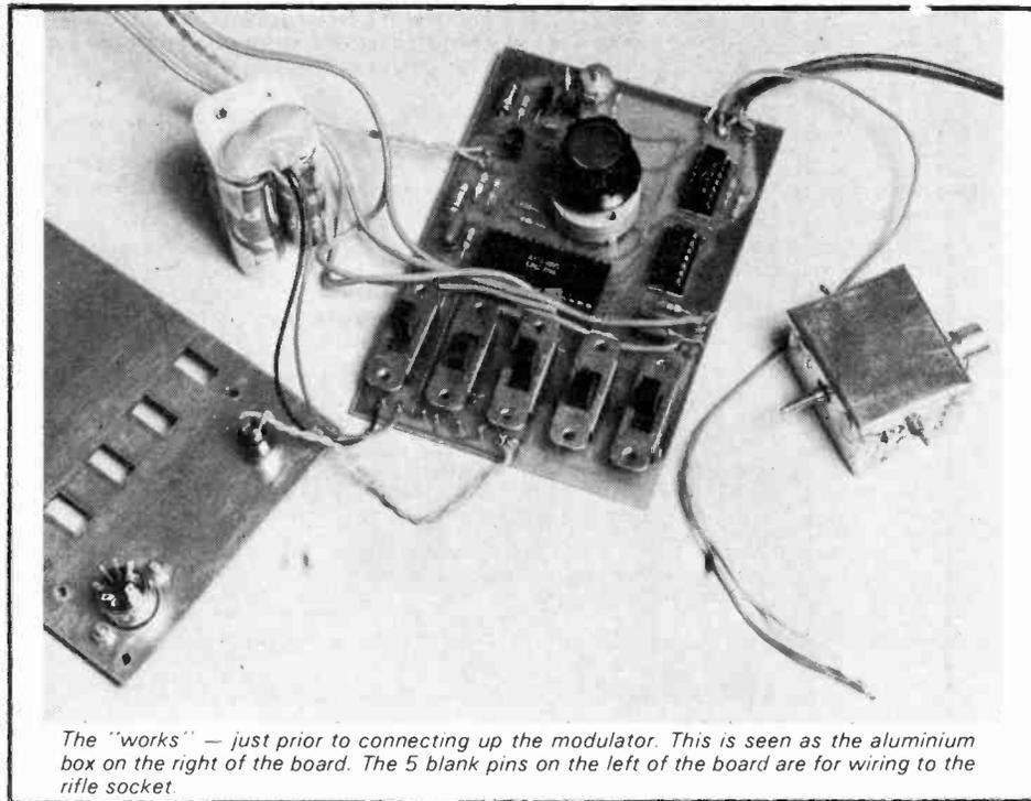
The "works" — just prior to connecting up the modulator. This is seen as the aluminium box on the right of the board. The 5 blank pins on the left of the board are for wiring to the rifle socket.
