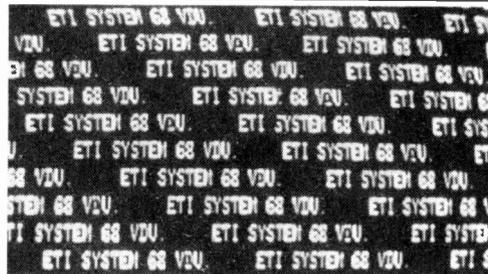
FEATURES include 64 character by 16 line display, parallel I/O with less than 1/4 second for full screen from memory, White on Black or Grey or any combination plus character flash. e.g. Black letters on grey flashing background. All built into a 2in module on two Eurocards!
