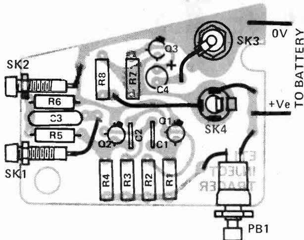
Fig 3. Component overlay. Note that SK2 and SK1 are held in place by the Verobox closing around them. SK3 and SK4 are attached directly onto the pcb, and face out of the box on the copper side of the board.
