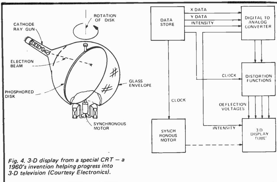
Fig. 4. 3-D display from a special CRT — a 1960's invention helping progress into 3-D television (Courtesy Electronics).
