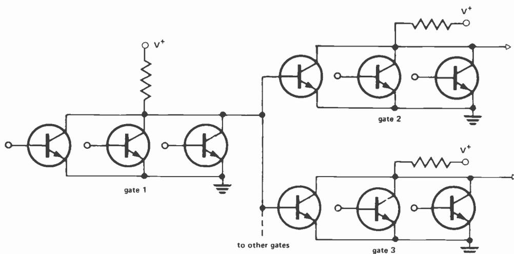
Fig. 1. A Direct Coupled Transistor Logic circuit (DCTL).
