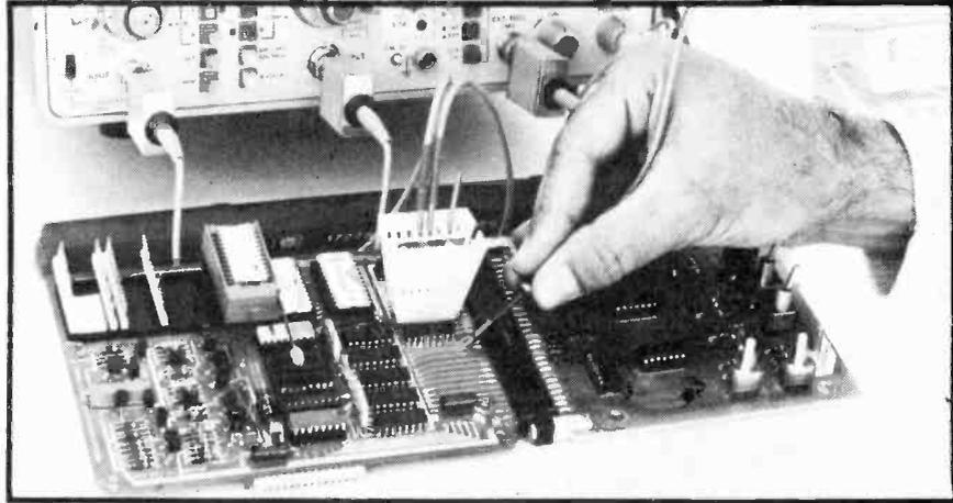
HP's solution to the problem consists of a clip that encompasses an entire DIP, and an accompanying set of demountable probes, believed the smallest yet commercially offered. The basic part of each probe can be inserted by itself into the DIP clip at any pin position; indeed, 15 of them can be inserted simultaneously into a DIP clip; one position is used with a grounding pin, so any pin on the DIP can be used as probe ground, holding lead inductance to a minimum.
