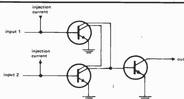
Fig.4. (above). I<sup>2</sup>L gates can be made by 'wire-ORing' the isolated collector outputs.
