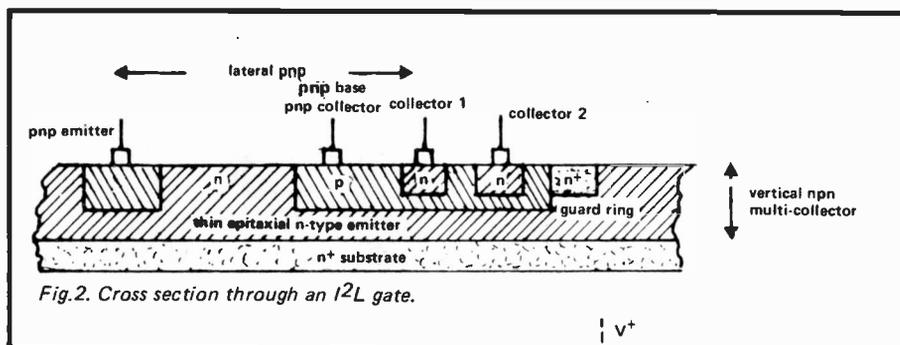
Fig. 2. Cross section through an I<sup>2</sup>L gate.
