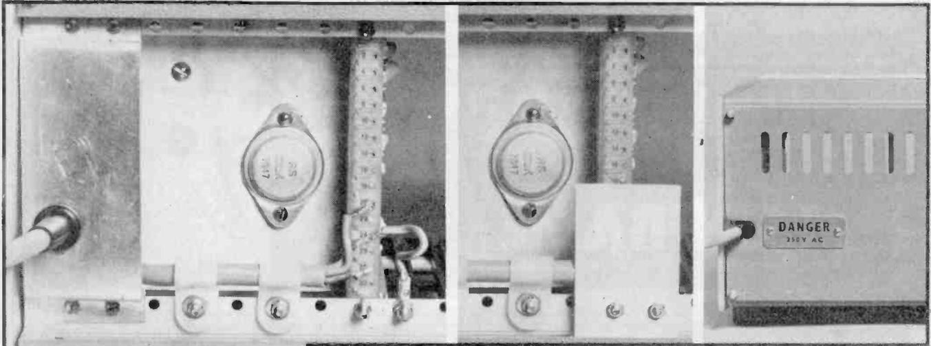
Fig. 3, 4, 5, the mains input on the back panel, note the positioning of 'p' clips and plastic guard. The sign came from a piece of surplus P.O. equipment.
