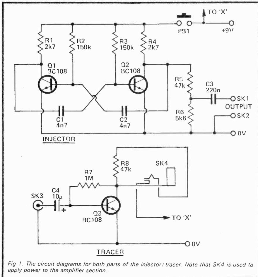
Fig 1. The circuit diagrams for both parts of the injector/tracer. Note that SK4 is used to apply power to the amplifier section.
