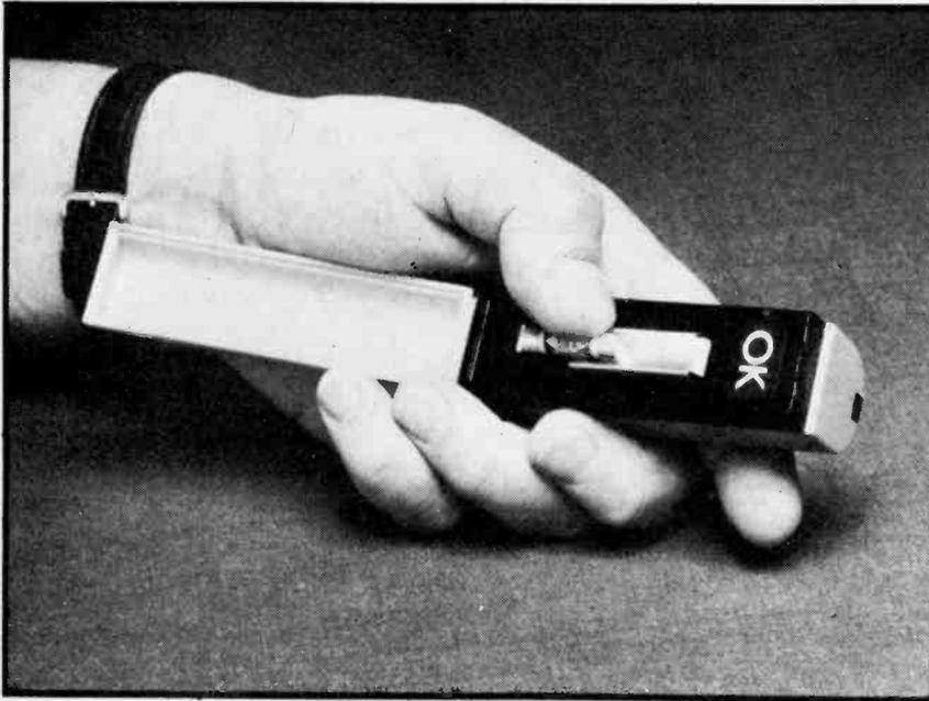
The first thing to check when a piece of mains equipment dies in its tracks is the fuse. Many an engineer has gone gibbering into a white coat with straps because he can't find the fault on a stubbornly inert heap of apparently perfect circuitry, while lurking in the plug is a burned out un-linking fuse.
