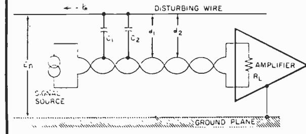
Fig. 5. Twisted wires provide best common-mode rejection when making connections between stages in which a symmetrical signal source is joined to a differential input amplifier.
