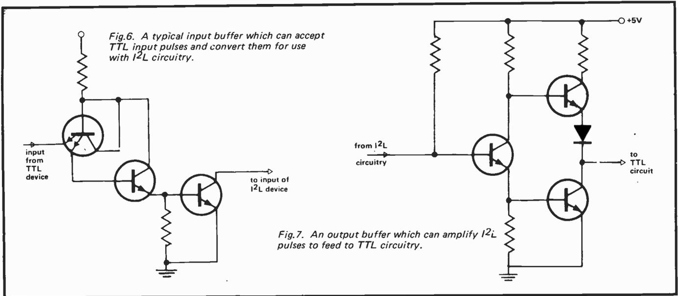
suitable only for the production of purely digital devices, although simple devices such as transistors and diodes can be fabricated on the chip. In contrast, Schottky TTL devices can be combined with I<sup>2</sup>L circuits on a single chip to produce products which are faster and which have higher component densities than can be achieved in other ways. The Texas Instruments SN74S201 and SN74S301 256 bit random access memories are examples of such products.
