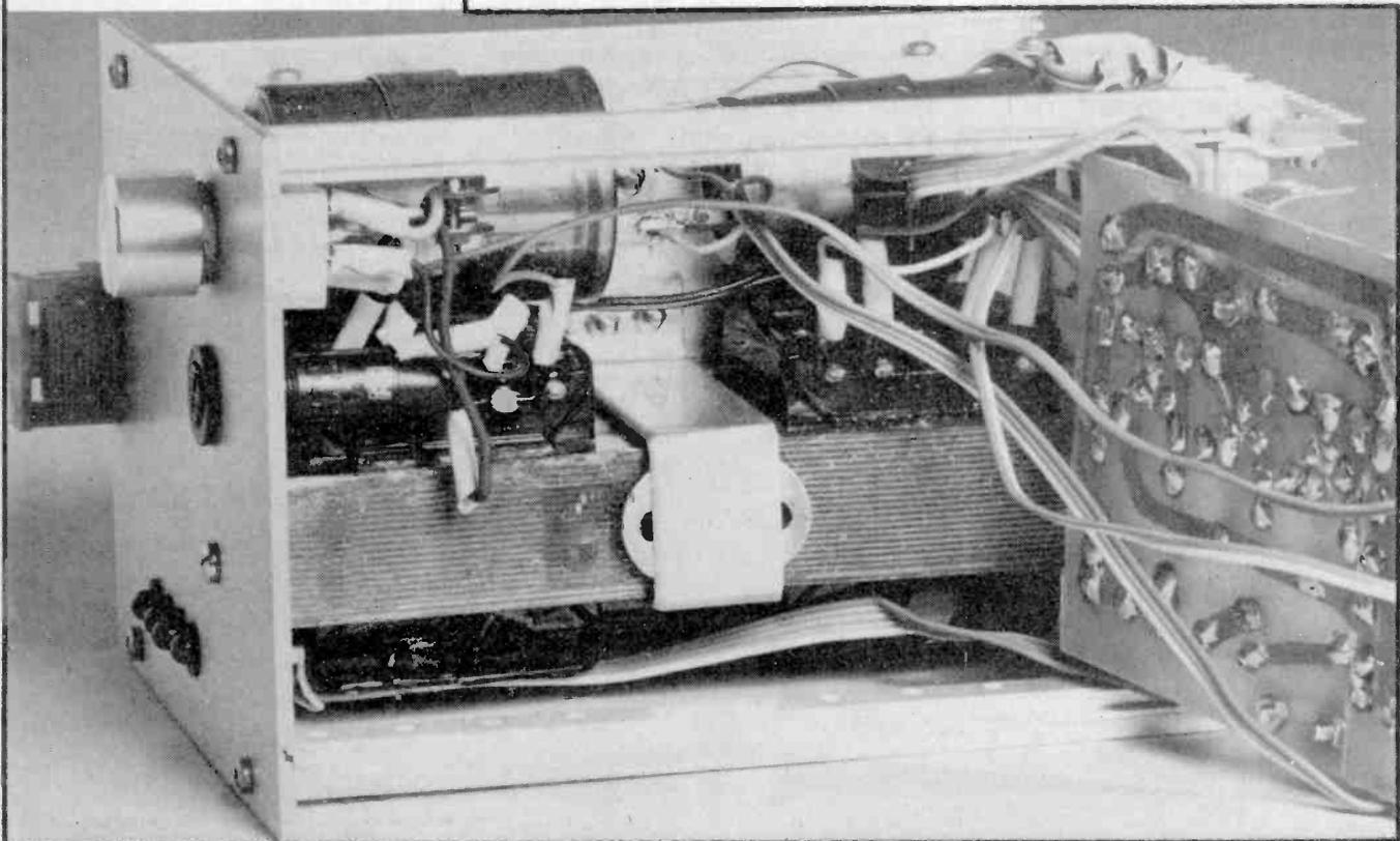
FS1, SW1 and LED 1-4 can be mounted on the front panel of the module. Ribbon cable and sleeving should be soldered to the LEDs (see figure on page 59). The two mains transformers can be strapped to the base plate, but first their mounting lugs must be bent. One lug is bent down through 90° and the other through 170°, see photographs to see how they mount. The two lugs bent through 170° are strapped under the mounting bracket. Both transformers should be wired up before C1 and C2 are mounted.
