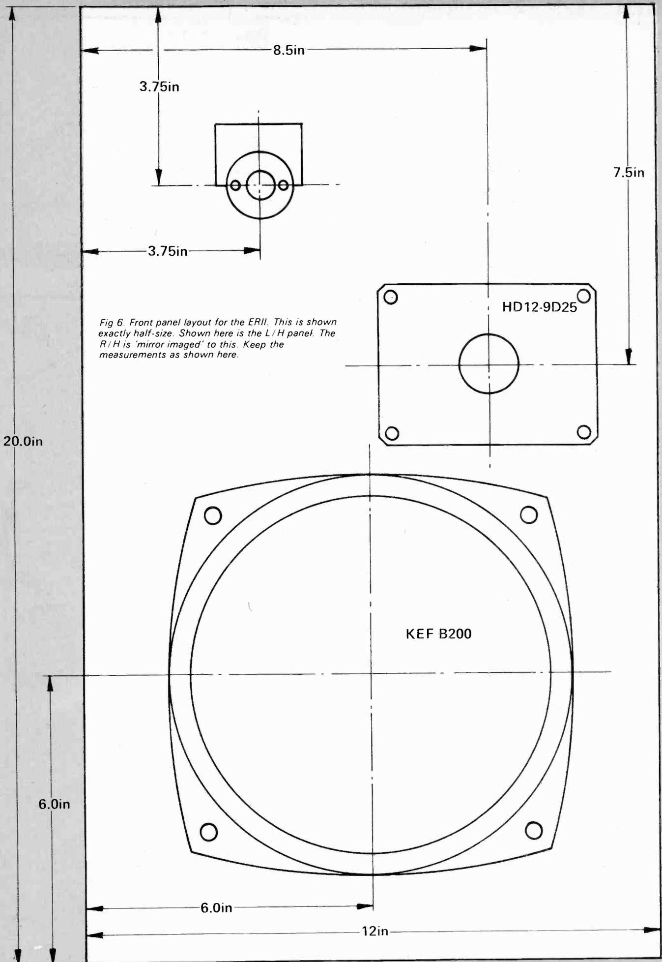
Fig 6. Front panel layout for the ER11. This is shown exactly half-size. Shown here is the L/H panel. The R/H is 'mirror imaged' to this. Keep the measurements as shown here.
