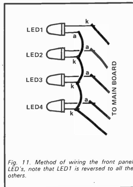
Fig. 11. Method of wiring the front panel LED's, note that LED1 is reversed to all the others.
