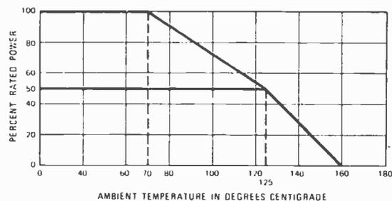
Fig. 3. Derating curve for dual-rated styles of cermet resistors.
