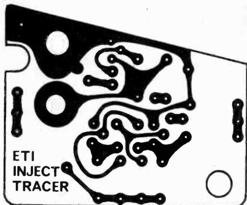
Fig 2. Pcb foil pattern for the circuit. Shown full size. The large areas of copper are where the sockets fix directly to the board.
