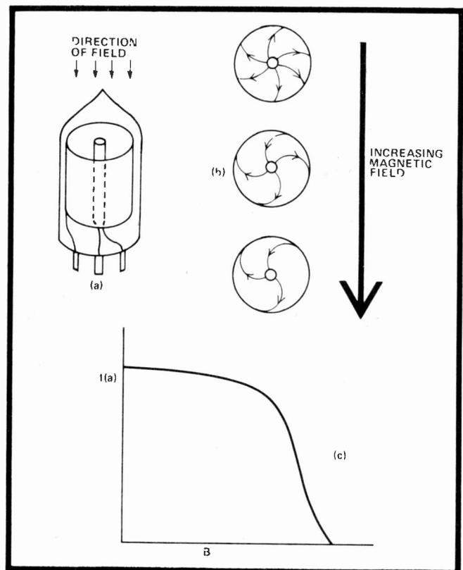
Fig 1. The magnetron effect. (a) Simple magnetron valve, magnet not shown. (b) Paths of electrons as the strength of the magnetic field is progressively increased. (c) Graph of anode current against magnetic field.
