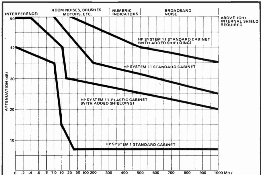
Fig. 6. Shielding of RF energy by various designs of enclosure used for H.P. instruments. The actual value of a particular unit depends upon the need for holes and shafts through the panels.
