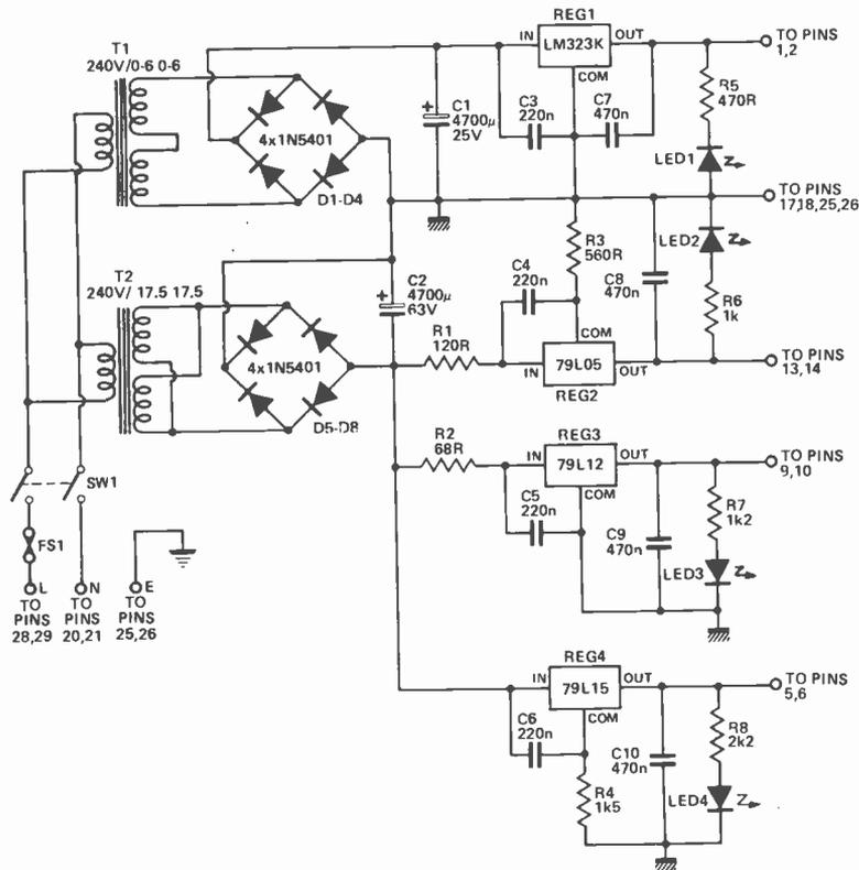
Fig. 7. Circuit diagram of the P.S.U.
