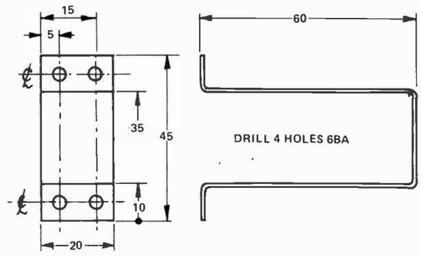
Fig. 9 Metal work details, front panel is not shown as exact positioning can be varied to allow for different components. See text.
