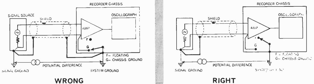
Fig. 3. Correct and incorrect methods of joining a sensor to a recorder. Most output instruments offer the user the choice of leaving the instrument floating above ground or grounding it.
