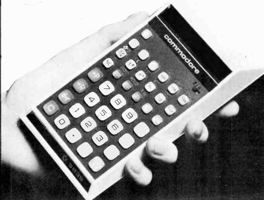
**FEATURES:** sin, cos, tan and inverse, change sign, exchange register,  $x^2$ ,  $y^x$ ,  $\log_e$ ,  $\log_{10}$ ,  $\sqrt{x}$ ,  $\sqrt{y}$ , rectangular and polar coordinates,  $e^x$ ,  $10^x$ , standard deviation and mean value, two memories, summation to memory,  $1/x$ , parenthesis, full arithmetic functions. Algebraic logic is employed.
