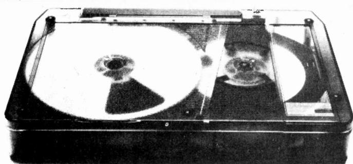
Fig. 6. This Sony cassette gives one hour of colour television with sound-tracks using a domestic television receiver to display the output of a special replay tape deck.
