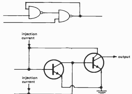
An output buffer circuit which can amplify the low voltage pulses from the output of an I<sup>2</sup>L circuit and provide enough current and voltage to drive a TTL input is shown in Fig. 7.
