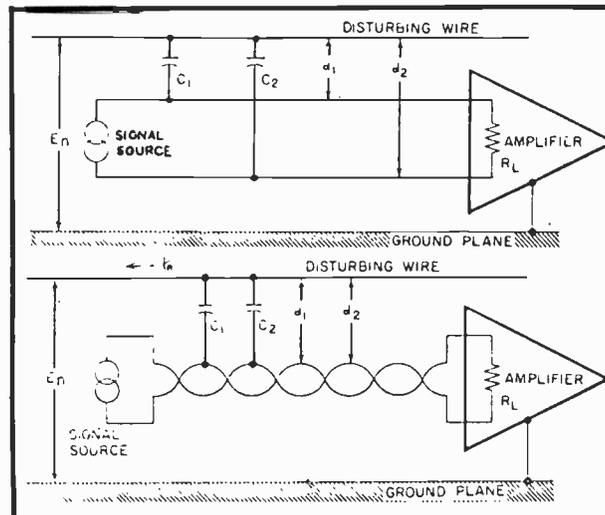
Fig. 4. Common-mode pick-up of noise is balanced out by the differential system.
