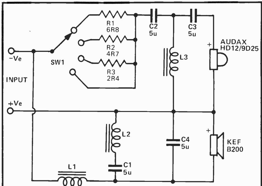
Fig 1. Circuit diagram of the crossover network. Component values are nominal. Note that R1-3 are mounted off board on to SW1 which is the h.f. level control. The units are wired in 'antiphase.'
