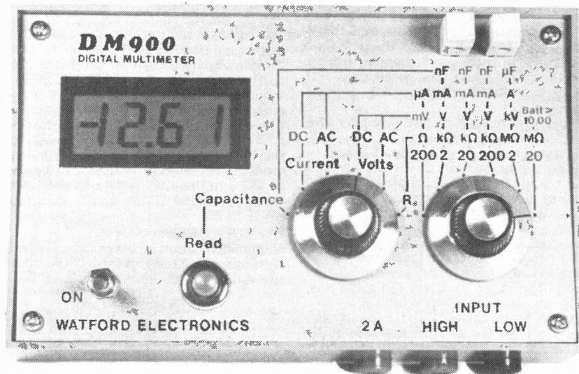
**Fig. 1. View of the final unit. Note, in order to ensure that the input sockets do not foul the PCB yet allow the probes to be inserted, the sockets should be mounted 10mm from the bottom of the case.**
