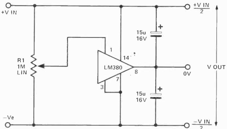
over 1 watt, and so extra cooling may be required. The device is fully protected and will go into thermal shut-down if its rated dissipation is exceeded, current limiting occurs if the output current exceeds 1A3.
