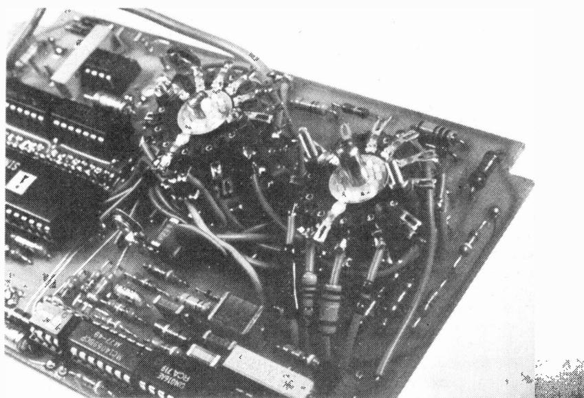
is obtained. If 1% resistors have been used where specified, changing to the next range should give a reading of exactly one tenth, and the next one hundredth, allowing for the plus or minus one digit accuracy. Calibration should ideally be done on the 200 mV range since this does not involve the attenuator, but this is not
