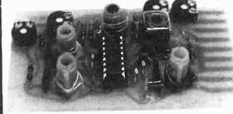
The EF5400, the first VHF tunerhead with one IC. It includes PIN diode agc loop, balanced osc/mixer, RF stage. Tunes 88-108 with only 2-Bv DC bias, and is adaptable up to 230MHz. £9.75 built/tested. Special frequency ranges on applic.
