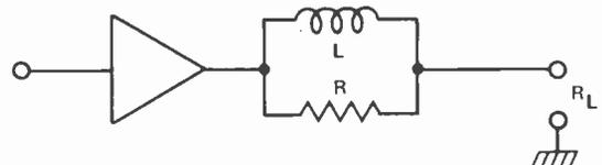
Ever wondered what this circuit in the output of an amplifier is for? Wonder no more — it's to aid the output stage in handling a capacitive loading by partially cancelling the effect.
