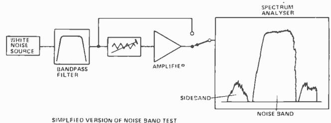
**Noiseband testing with a spectrum analyser, the sidebands produced by the amp are clearly visible.**
