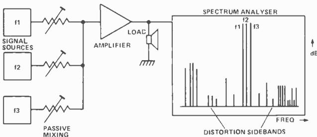
**Intermodulation distortion testing using three frequencies.**
