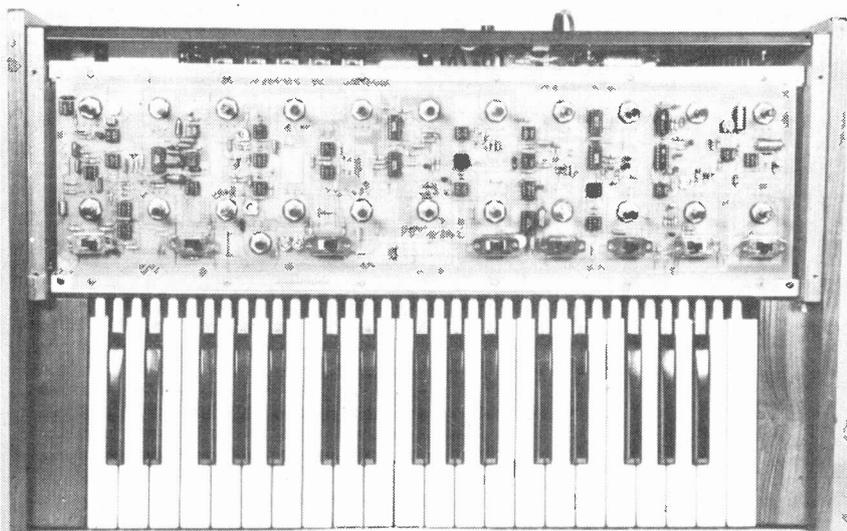
spacers for this purpose. Non-kit types have to work out the height of their front panels from the board and act accordingly. The switch toggles must come level with the pot spindles, when cut to take the control knobs.
