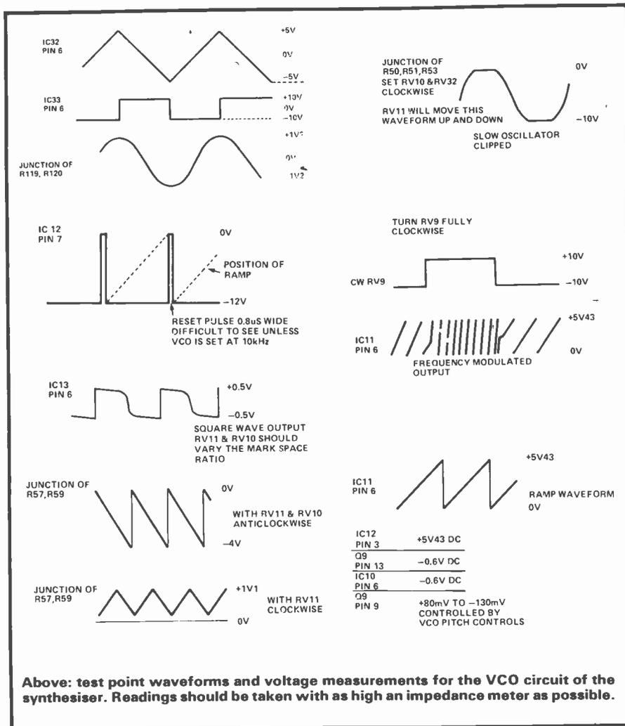
Above: test point waveforms and voltage measurements for the VCO circuit of the synthesiser. Readings should be taken with as high an impedance meter as possible.
