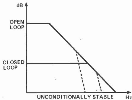
Above: Effect of adding an extra pole at the output of an unconditionally stable amplifier, such as might be added by a complex crossover network. Below: Same condition applied to marginally stable type. Phase shift now borders on 180°, i.e. oscillation.
