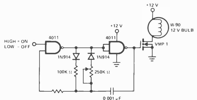
Fig. 8. Circuit of a high-efficiency light dimmer.
