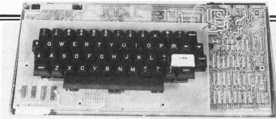
The interior of the TRS-80 reveals two PCBs, one of which carries the keyboard while the other deals with the rest of the TRS-80's circuitry. The flexible connector that joins the two boards can be seen bottom left while the expansion bus is at top left.
