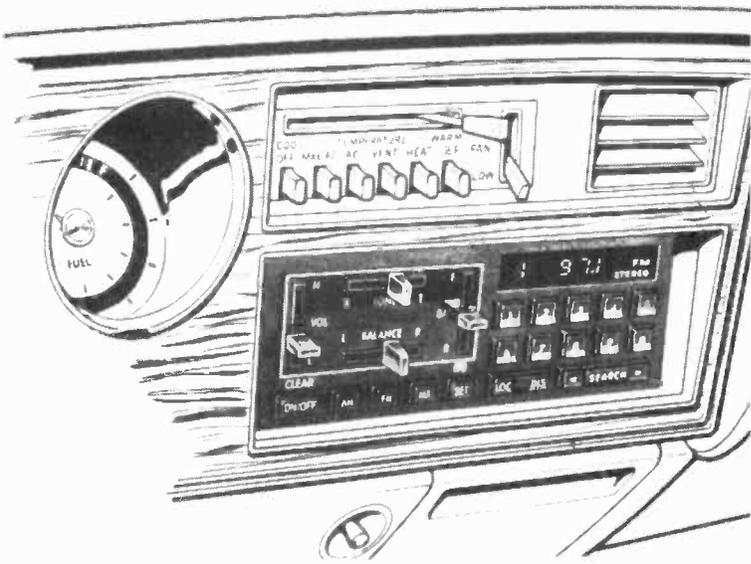
Fig. 3. Microprocessor control circuitry allows Chrysler's new AM/FM Stereo Search radio to recall ten stations from its internal memory. A LED display shows the frequency and number of the selected station.
