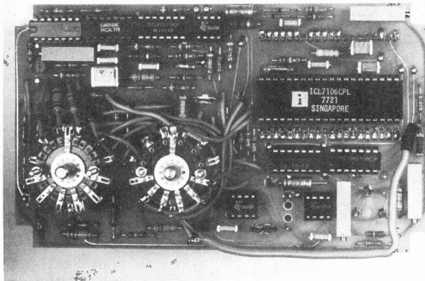
Fig. 6. Above, view of completed circuit, and Fig. 7 below, view of wiring around the range switches.
