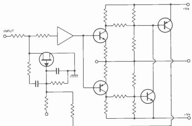
In this protection circuit the FET starts to turn-on when full-power is delivered into a 2 Ohm load. The main advantage over a conventional protection circuit is that the limiting is "soft" (i.e. very gradual) and thus audibly acceptable and secondly that the distortion is much lower — and still only about 0.1% at limiting.
