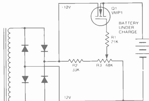
Fig. 16. Tapered-current voltage-limited battery charger.
