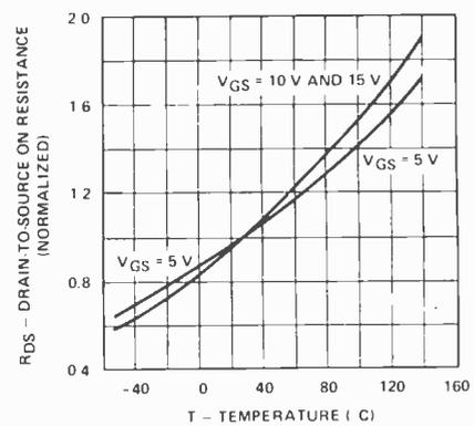
Fig. 6. Drain to source resistance against temperature (Siliconix).
