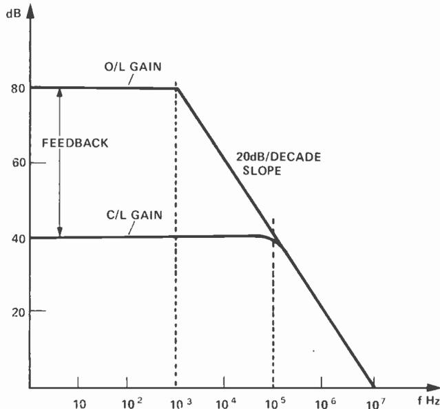
In the case shown in the diagram (unconditional stability) the open-loop response of the amplifier is stabilised by rolling it off at a slow 20 dB/decade slope with a single pole at 1 KHz. This amplifier would be stable with any amount of resistive feedback. However it will be seen that at higher audio frequencies the amount of feedback available reduces and so the distortion of the amplifier will increase. For this reason many amplifiers are of the "marginally stable" type.
