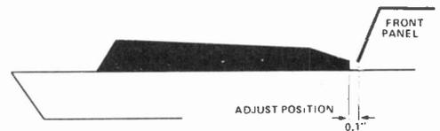
On the left is the diagram you'll need to line up the keyboard assembly with the casing and front panel. Follow this as carefully as you can, as if the keys are not in the right places, the contact blocks will not line up with the plungers, and the keys themselves will probably foul the front panel. Above is shown the alignment of keys and panel.
