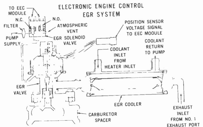
Fig. 6. Above, diagram of the Electronic Engine control system featured in the 1978 Lincoln Versaille.
