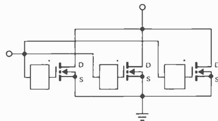
\*TO PREVENT SPURIOUS OSCILLATIONS, A 500 Ω 1K Ω RESISTOR OR FERRITE BEAD (FOR HIGHER SPEED) SHOULD BE CONNECTED IN SERIES WITH EACH GATE
