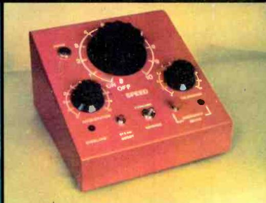
A pulse width train controller for smooth slow running plus inertia braking and acceleration. Full construction details in our catalogue.
