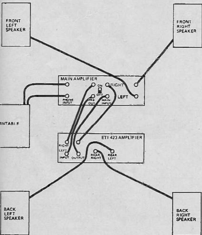
Fig. 1. This schematic drawing shows how the add-on unit is connected into the existing stereo system.
