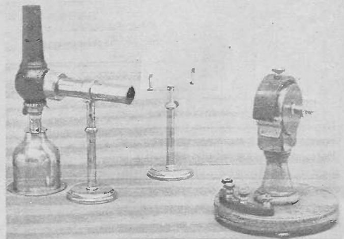
Fig. 1. Kelvin's galvanometer (1858). The oil lamp, at left, provided a light beam that was deflected by a mirror mounted on the coil of the galvanometer at right. The deflected beam moved across the calibrated scale at centre.
