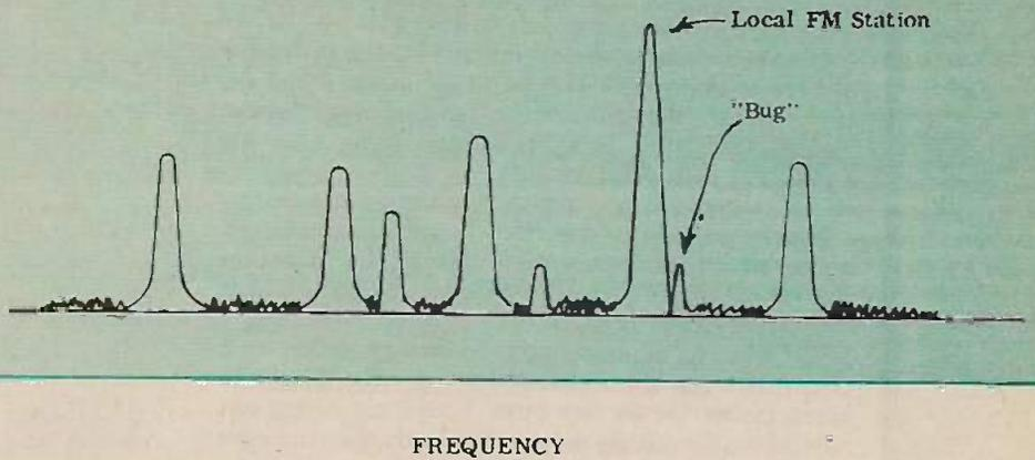
Fig. 4. Experienced bugging operators often tune a bug's transmitter frequency so that it is all but 'hidden' by a strong local station.
