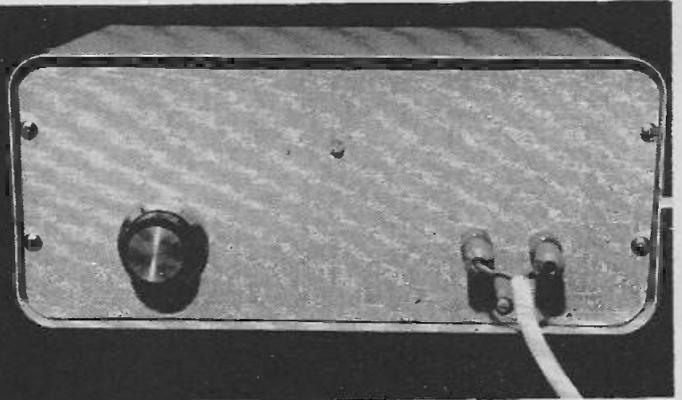
THIS UNIT is automatically operated by the level of general illumination, or the strength of light falling upon it. The most frequent uses of such a device include operating a child's night light, or switching on a light in a room, when darkness falls, as a deterrent to burglars, when leaving the house unoccupied.
