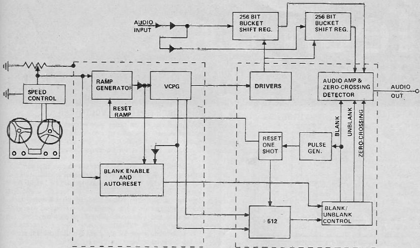
Fig. 1. Block diagram of the Variable Speech Control, a system which can slow or speed up speech without altering the frequency. This diagram shows the IC's which are being developed in the USA and how they control the tape recorder and the audio signals.
