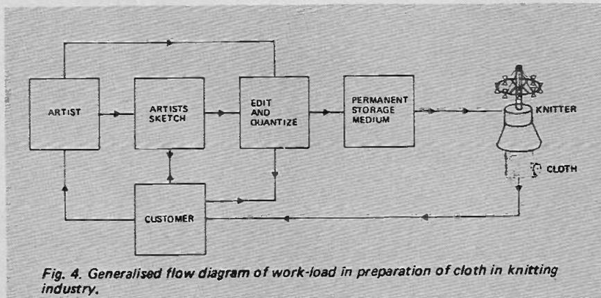
Fig. 4. Generalised flow diagram of work-load in preparation of cloth in knitting industry.
