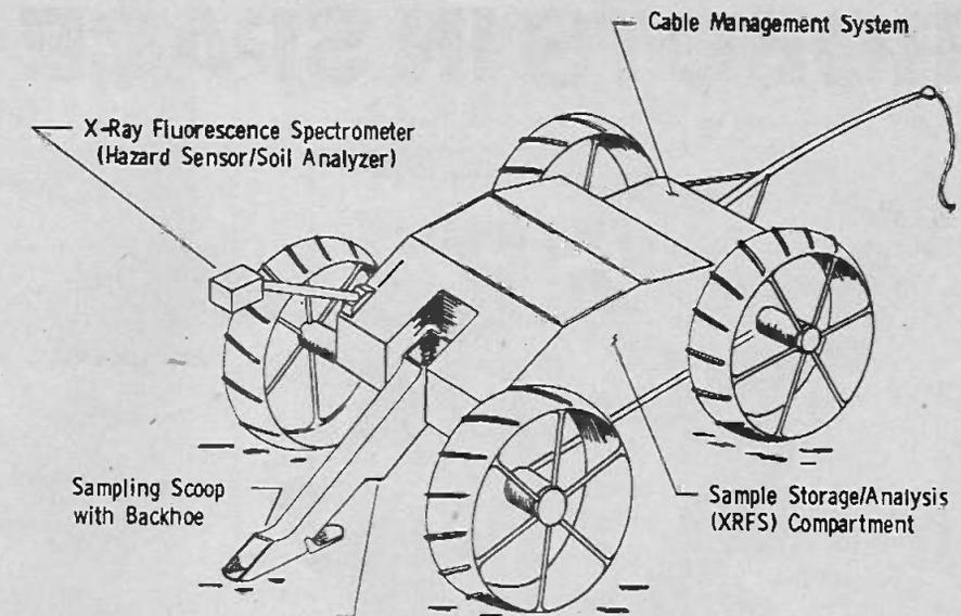
Fig. 2. Tethered rover associated with advanced lander.
