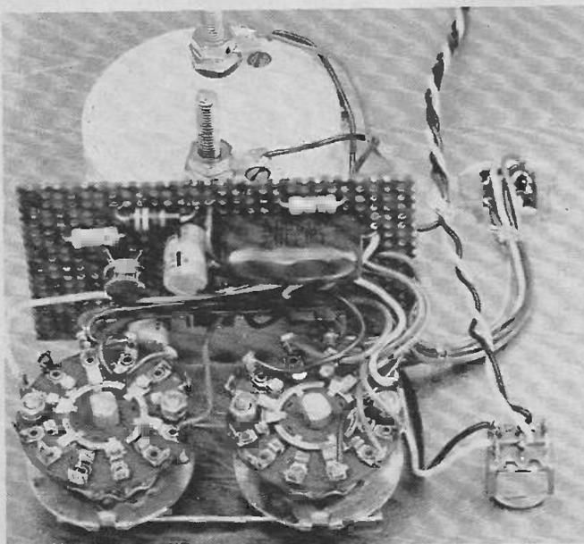
Showing the internal construction of the tester. Note that matrix board hold the majority of the components.
