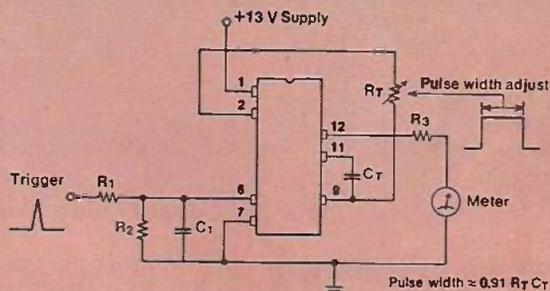
Block diagram and wiring of the SW781 Tachometer from Marshall's.
