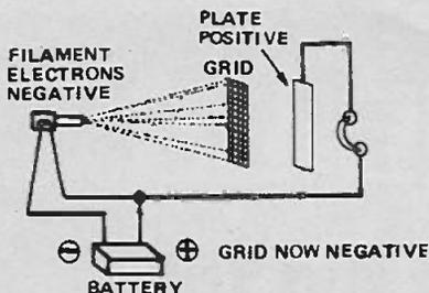
SHOWING HOW THE GRID PREVENTS THE ELECTRONS FROM REACHING THE PLATE
