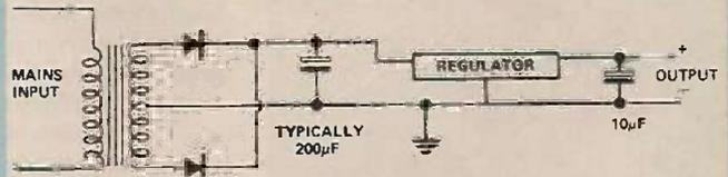
When experimenting with integrated circuits, constructors often employ a normal mains power pack or a battery which can give a large current on a direct short in the output circuit. Such accidental shorting can occur very easily during preliminary experiments with integrated circuits and some of these shorts will probably result in the destruction of one or more devices.
