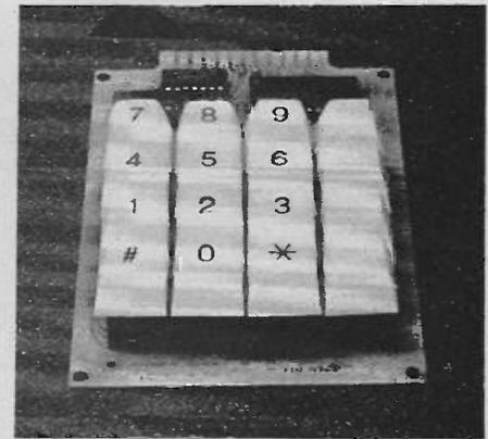
Each keyboard has a Harris HD-1065 keyboard encoder, giving a 4-bit parallel output and 2-key roll-over. All outputs are bounce-free and TTL-compatible. The keyboards are initially coded in BCD, but the coding can be altered in the field, if desired. In addition these keyboards are available with single line (uncoded) outputs.
