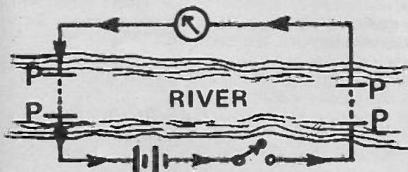
Fig. 6. In 1842 Morse demonstrated wireless electrical communications using the ground as "wires".
