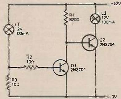
A signal lamp used to indicate failure of a vital piece of equipment is subject to failure itself.
