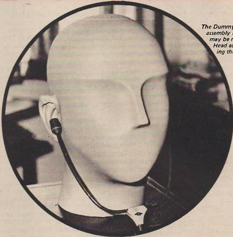
*The Dummy Head with microphone assembly in position. Recording may be made either by using the Dummy Head as shown here — or by using the microphones on*
