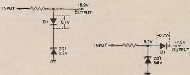
A silicon diode when forward biased has a constant voltage drop of 0.7 volts. A germanium diode has 0.2 volts.
