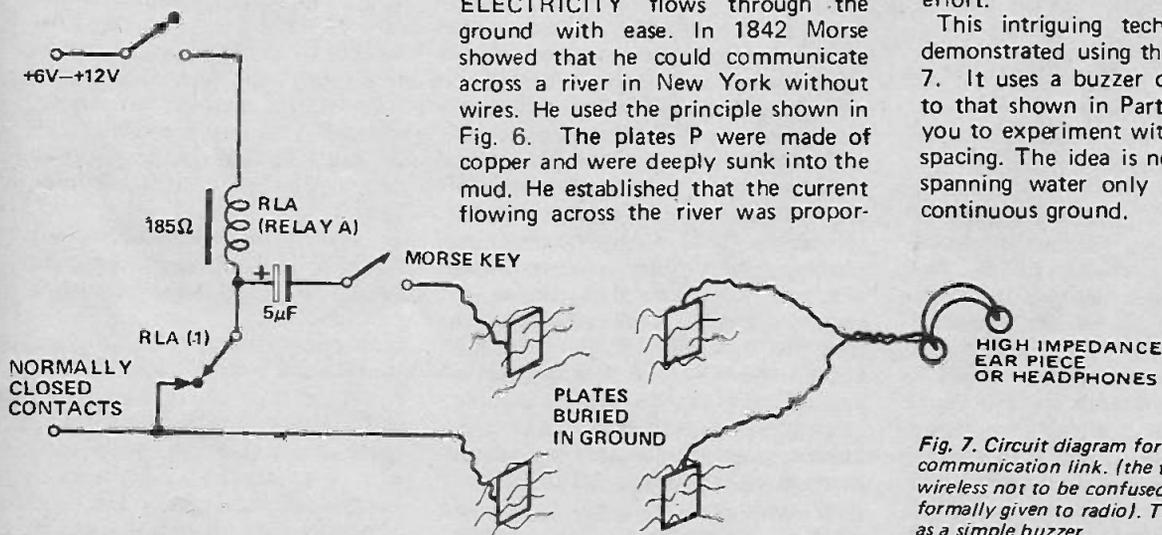
tional to the plate size, and to the distance between the plates on each side. (The current paths do not short out!) Lindsay signalled across the 1.5 km width of the river Tay, Scotland, in 1854 by this means. After this, many attempts were made to bridge larger distances but as the method is very inefficient little came of such effort.
