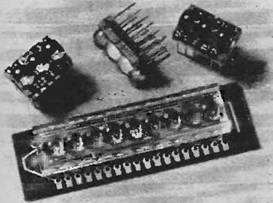
Litronix have a new pre-aligned PCB-mounted numeric display. Intended primarily for hand-held calculator applications, the DL-95 can be supplied either as an 8-digit display with a left-hand minus sign, or as a 9-digit display without polarity indication. The digits, which are slanted at 10°, have a magnified height of 0.1 in. on 0.2 in. centres, and include a decimal point.
