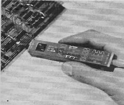
By means of the quasi-oscilloscope display, pulses can be easily verified. Differences can be observed between pulses at high and low levels, pulses at a duty cycle of 1:1 and pulses at duty cycles both  $>1$  and  $<1$ . This estimation of duty cycles provides unambiguous results up to a frequency of approximately 0.5MHz.
