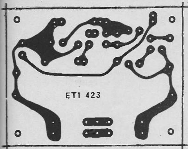
Fig. 6. Printed circuit board for the power supply.
