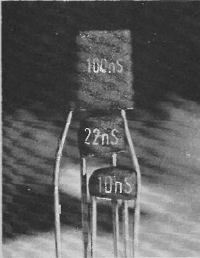
Utilization of parallel plate construction results in a capacitor of narrow profile suitable for high density component packaging in electronic equipment. Whilst primarily a radial component, because of its 26mm leads of 0.6mm diameter, the B37448/9 also lends itself to axial applications, for example in RF circuitry. Typically the 10nf version measures 6mm wide x 4mm high x 2mm thick, and is priced at £2.90 per 100.
