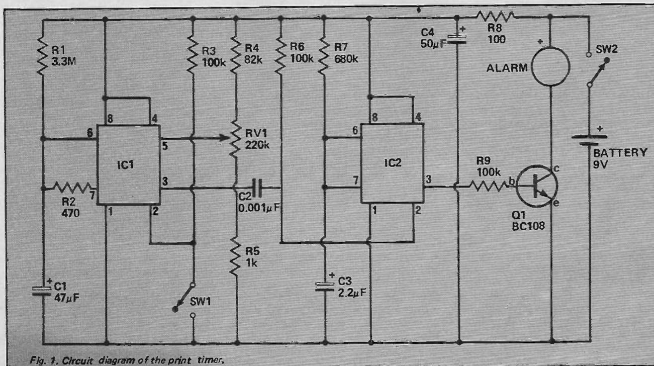
Fig. 1. Circuit diagram of the print timer.
