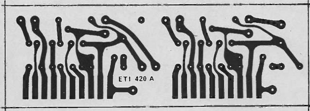
Fig. 3. Printed circuit board for the twin power amplifier assembly.
