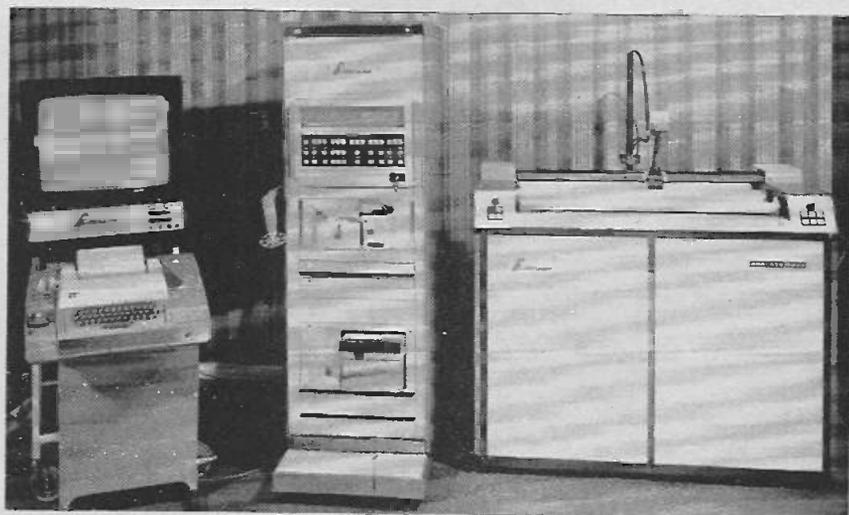
Fig. 6. Time saver pattern data preparation system.
