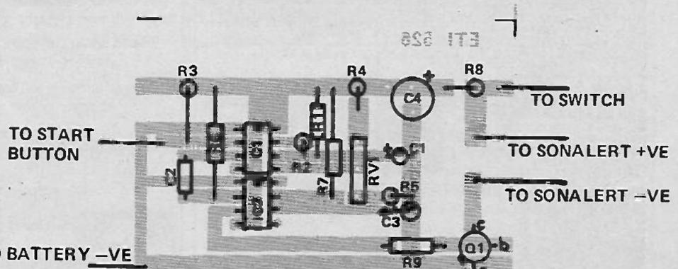
Fig. 4. Component overlay.
