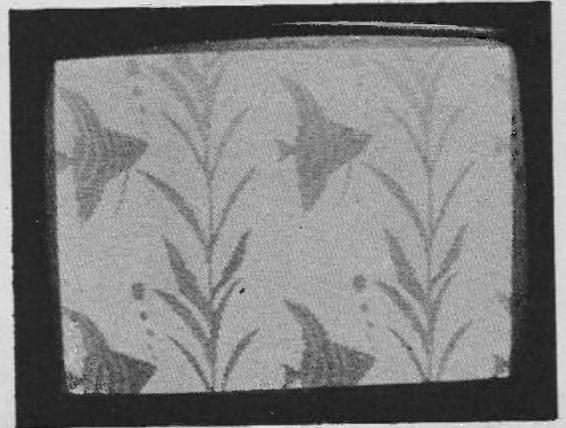
Fig. 7. The designer needs only to produce one cycle of the pattern — the computer-based colour display repeats it to provide a view of the complete pattern.
