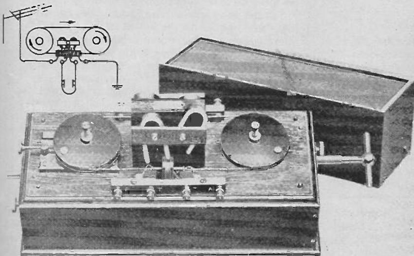
Fig. 2. Marconi's magnetic detector of 1902.
