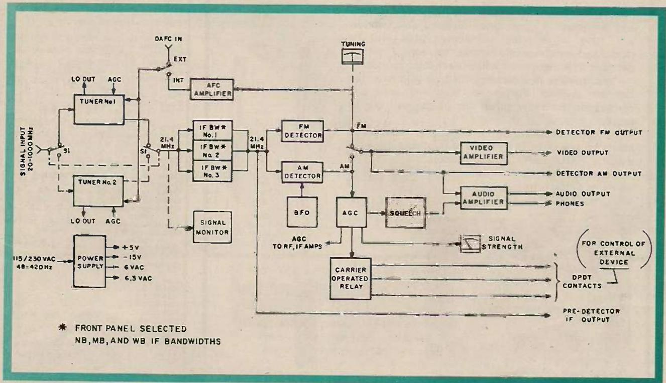
Block schematic of typical surveillance receiver used for radio bug location.
