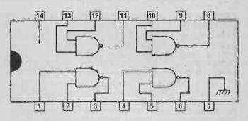
7400, using single strand insulated wire. Use the LED which is connected to pin 3 of the 7400 as an indicator.
