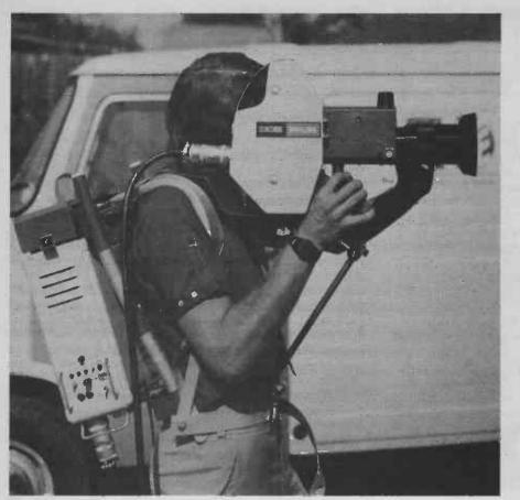
To the left is a picture of the new Philips LDK-11 colour camera.
