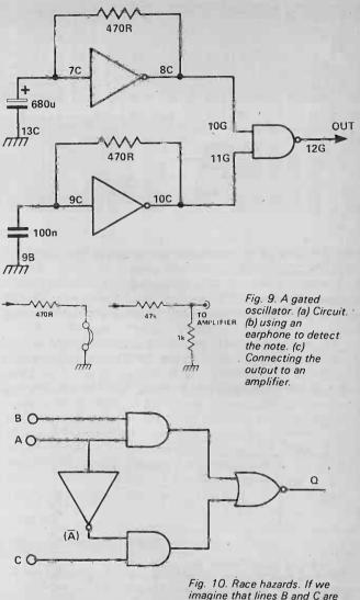
IF B=1 AND C=1, THEN A CHANGE OF A FROM 1 TO D CAUSES A BRIEF PULSE AT Q. Fig. 10. Race hazards. If we imagine that lines B and C are both at one, then the change from A = 1 to A = 0 should cause no change in the output. Because of the delay in the inverter, however, A goes low just before  $\overline{A}$  goes high so that there is a narrow negative pulse developed at the output. This could cause problems if a counter were being driven from the output.
