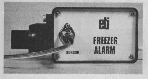
The completed Freezer Alarm showing how we mounted the audio warning device on our prototype.
