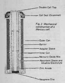
electrolyte is a solution of alkaline hydroxide, the ions of which act as carriers for the cell's chemical action. The electrolyte is not consumed during discharge. The cell containers are nickel plated steel and thus do not corrode.
