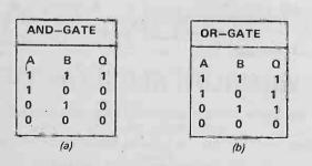
Fig. 2. Truth tables. (a) AND-gate. (b) OR-gate.
