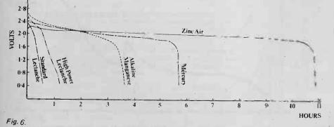
Discharge curves of various types of cell compared to a zinc-air battery of the same physical size.
