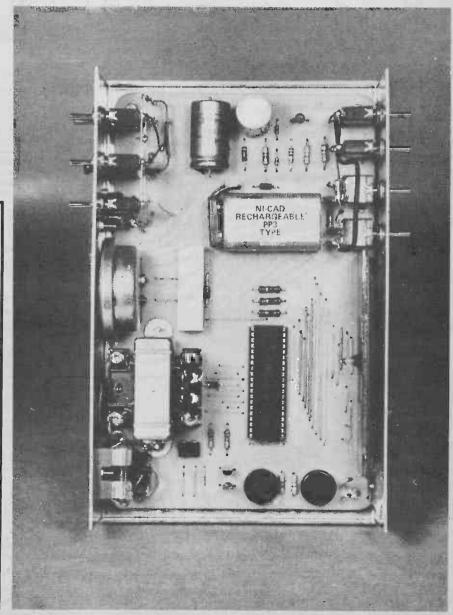
Right: Internal layout of the design. You can just see the display sitting in the bottom right of the board. Next to this are the links to rearrange the chip pinouts into the same order as the display pin-ins. Below these the two presets are for brightness and alarm volume. In case you're wondering what that white
