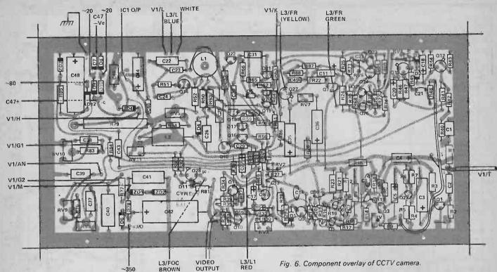
camera's chassis. IC1 should also be mounted on the chassis, taking care that there is a good thermal contact between the regulator and chassis as the device dissipates a fair amount of heat in normal operation.
