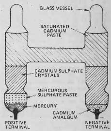
Fig. 7. The Weston Cadmium cell.
