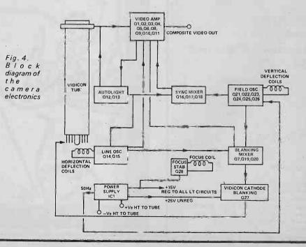
As can be seen from the block diagram the electronics of the camera can be broken down into nine distinct sections.
