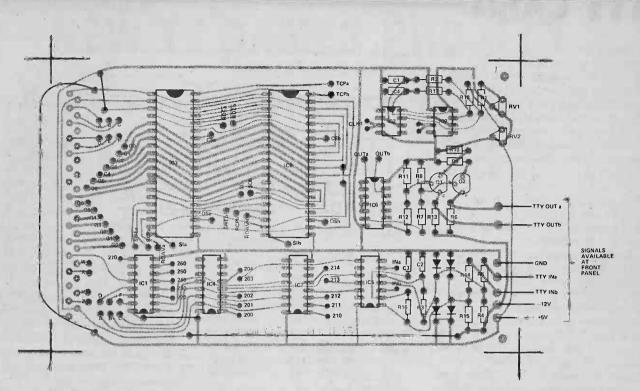
To the left we show the full size foil pattern for the TTY card (160mm) wide. Above is the component overlay while below is a flow chart for a typical 1 / 0 routine.
