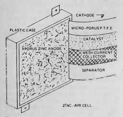
Fig. 5. Section of rectangular zinc-air cell.
