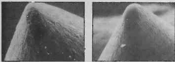
Above left: a conventionally polished stylus tip under extreme magnification. Above right: the V15V MASAR polish under the same power magnification. Note how much smoother the contact area appears. This could lead to lower surface noise and reduced record wear.
