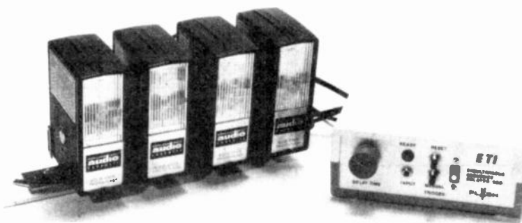
The ETI Flash Sequencer can control up to four flashguns.
