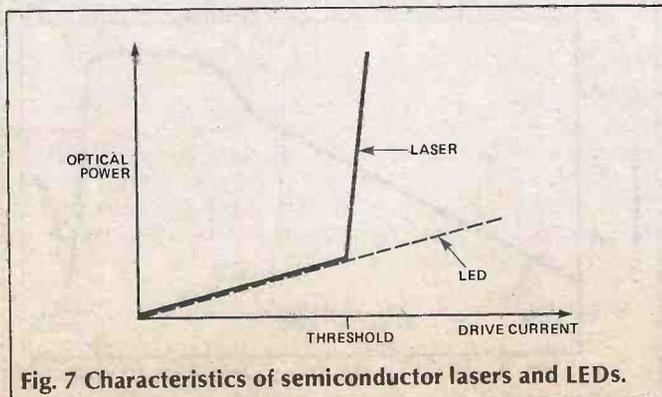
Fig. 7 Characteristics of semiconductor lasers and LEDs.
