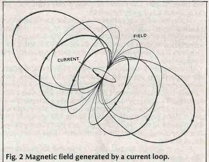
Fig. 2 Magnetic field generated by a current loop.
