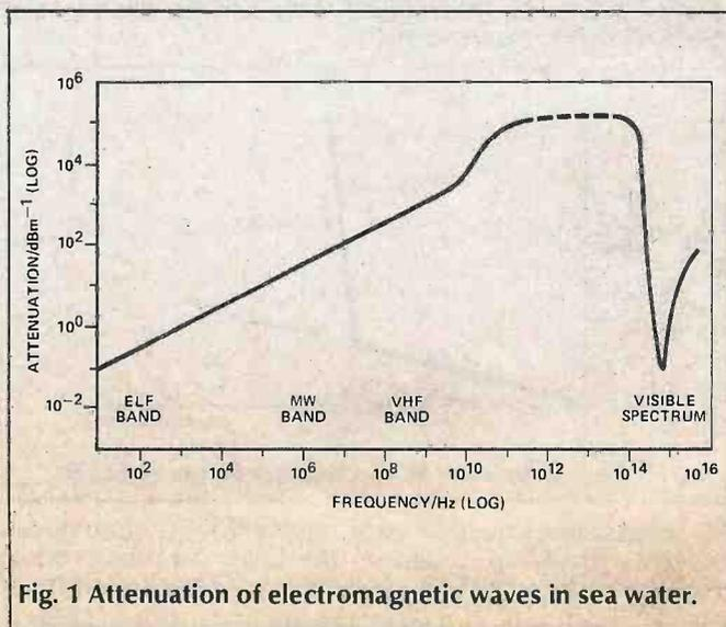
Fig. 1 Attenuation of electromagnetic waves in sea water.
