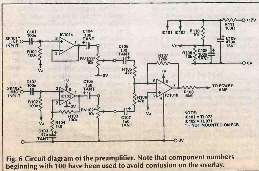
Fig. 6 Circuit diagram of the preamplifier. Note that component numbers beginning with 100 have been used to avoid confusion on the overlay.
