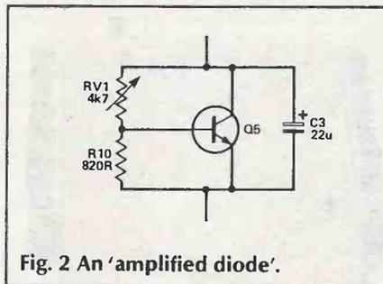
Fig. 2 An 'amplified diode'.
