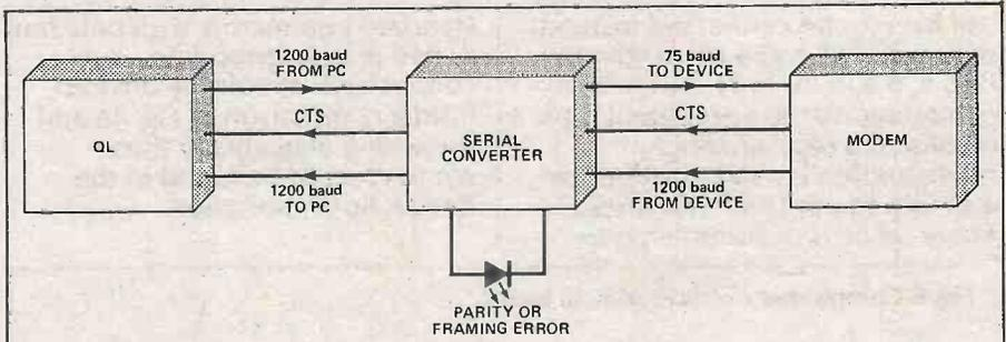
Fig. 7 The QL linked to a back channel (75/1200) modem.
