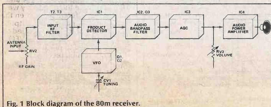
Fig. 1 Block diagram of the 80m receiver.
