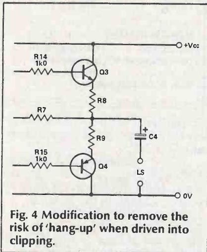
Fig. 4 Modification to remove the risk of 'hang-up' when driven into clipping.
