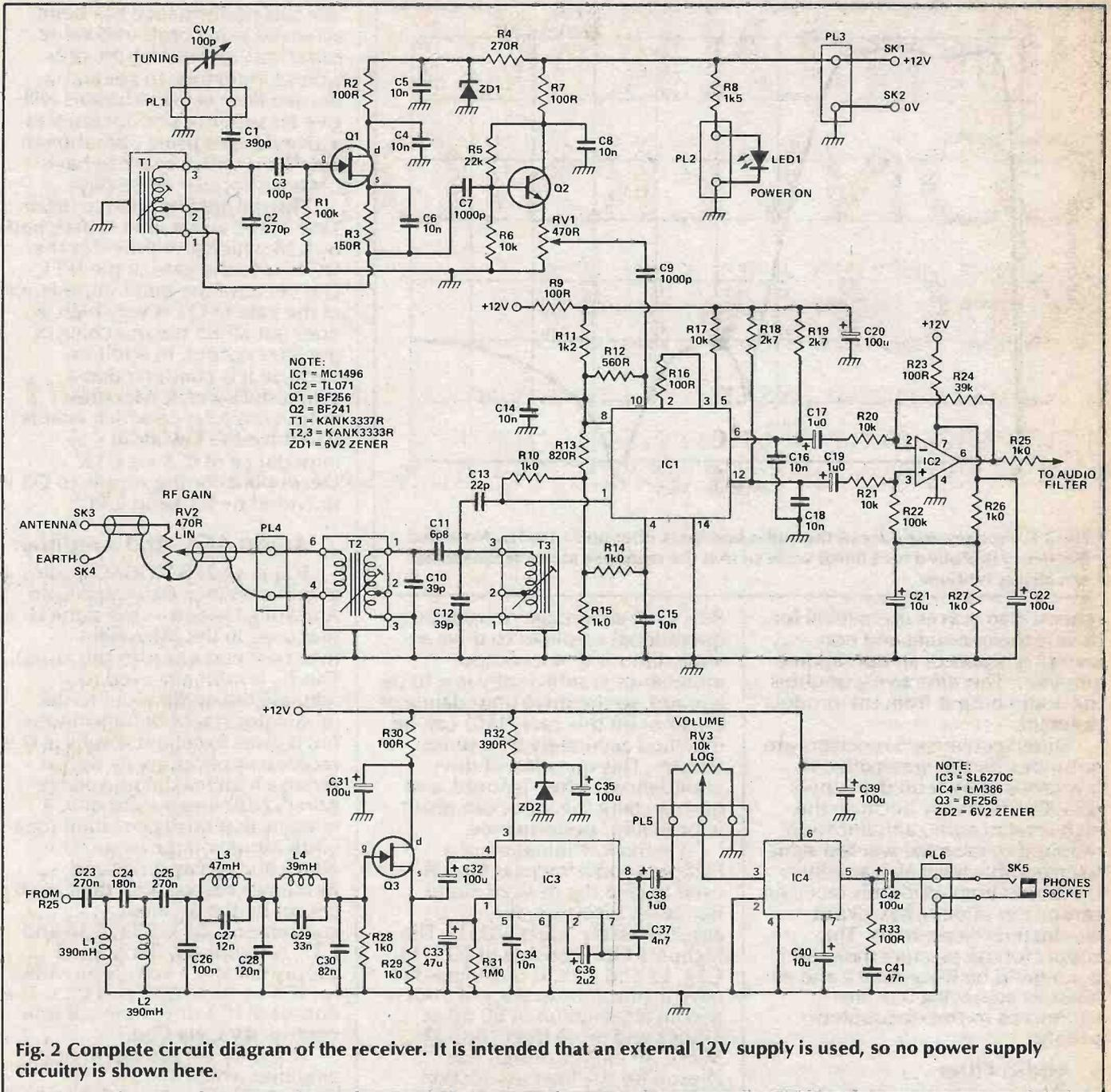
Fig. 2 Complete circuit diagram of the receiver. It is intended that an external 12V supply is used, so no power supply circuitry is shown here.
