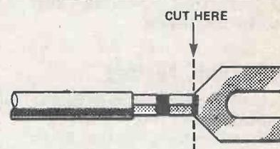
TURN TERMINAL OVER, SCRAPE-CLEAN THE UNDERSIDE, SOLDER TO THIS SURFACE
