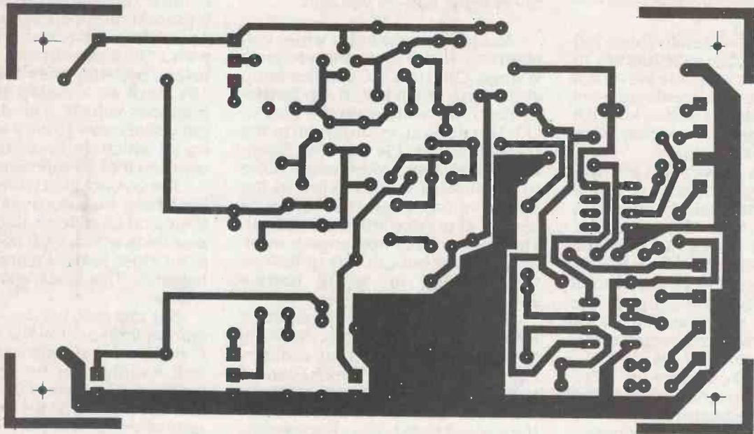
The foil pattern for the JLLH PA amplifier board.
