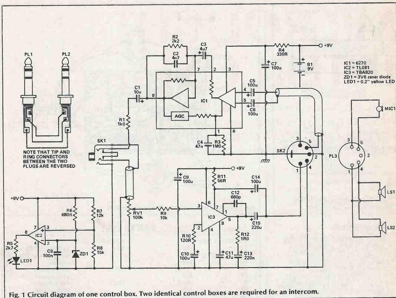
Fig. 1 Circuit diagram of one control box. Two identical control boxes are required for an intercom.
