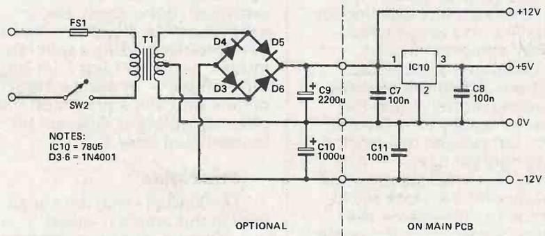
Fig. 3 Optional PSU — components to right of dotted line are on main board.
