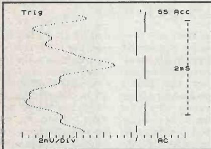
The AliDin Scope Module plugs into the ZX Spectrum expansion port and is completely controlled from the computer's keyboard, thus there are no knobs or dials and all settings are displayed on the screen, see above screen dump.
