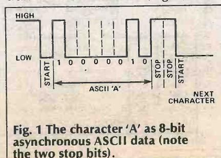
Fig. 1 The character 'A' as 8-bit asynchronous ASCII data (note the two stop bits).
