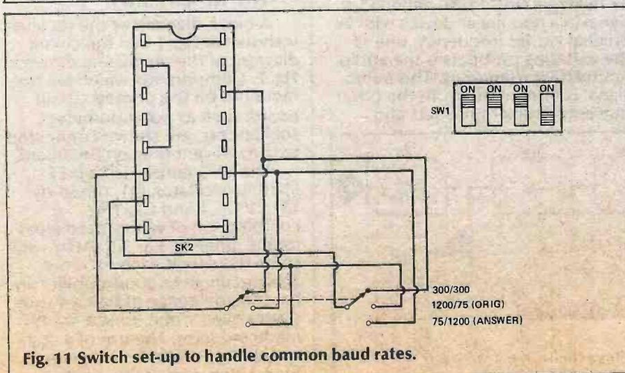
**Fig. 11 Switch set-up to handle common baud rates.**
