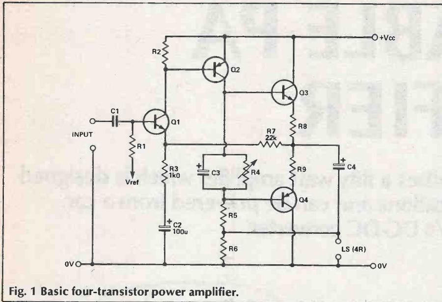
Fig. 1 Basic four-transistor power amplifier.
