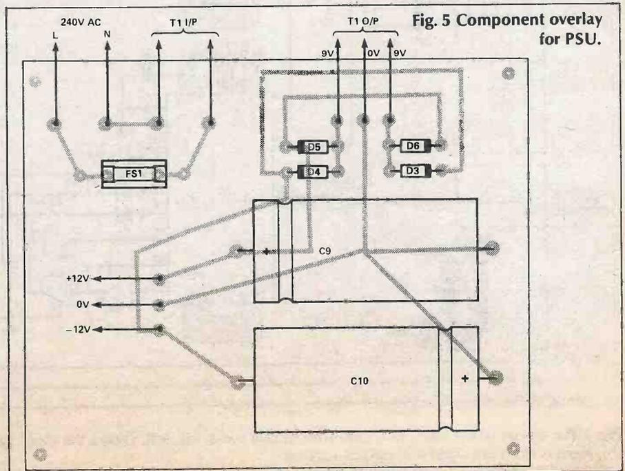
Fig. 5 Component overlay for PSU.
