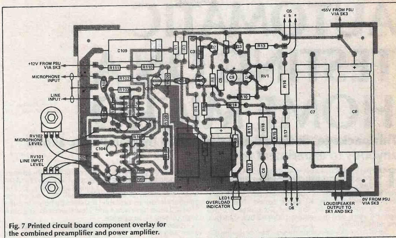
Fig. 7 Printed circuit board component overlay for the combined preamplifier and power amplifier.
