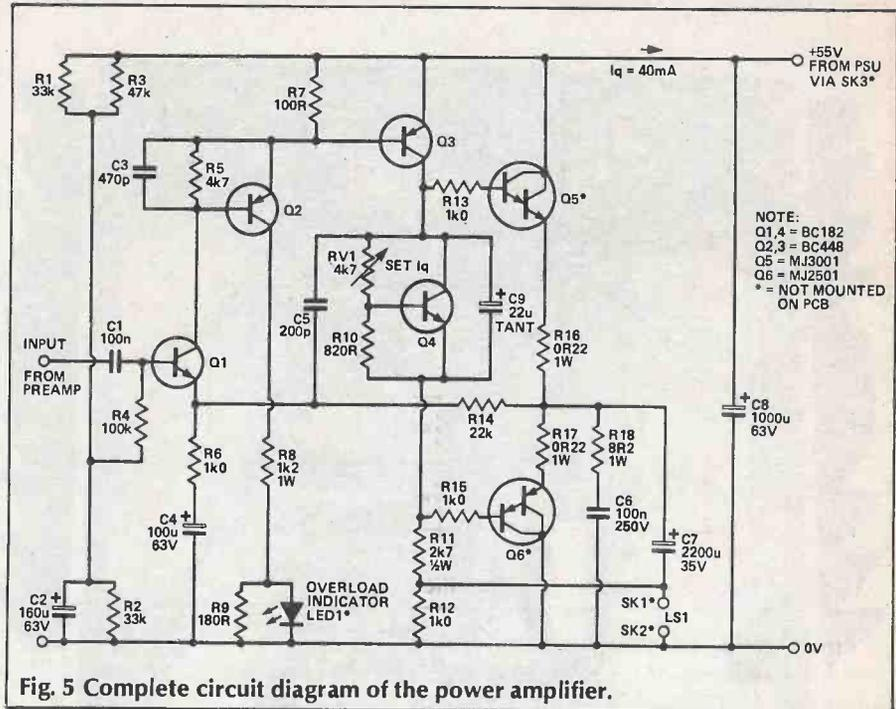
Fig. 5 Complete circuit diagram of the power amplifier.
