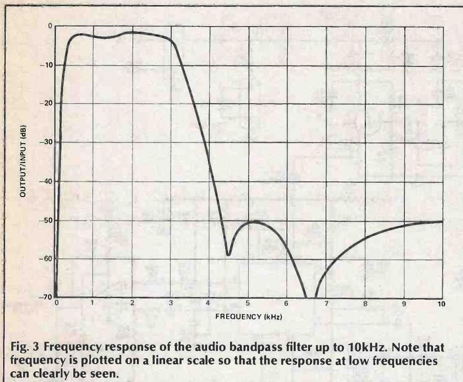
Fig. 3 Frequency response of the audio bandpass filter up to 10kHz. Note that frequency is plotted on a linear scale so that the response at low frequencies can clearly be seen.
