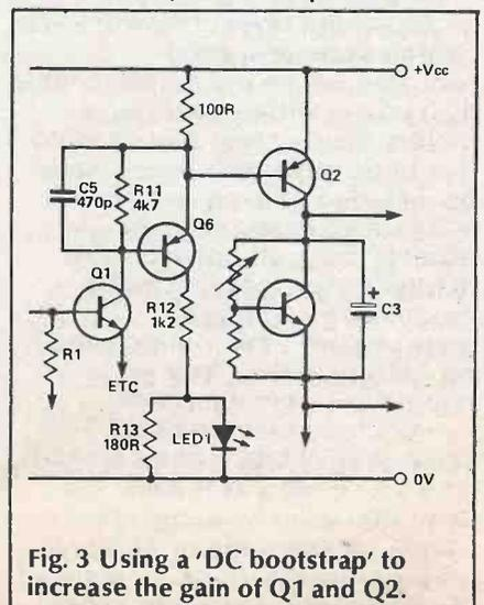
Fig. 3 Using a 'DC bootstrap' to increase the gain of Q1 and Q2.
