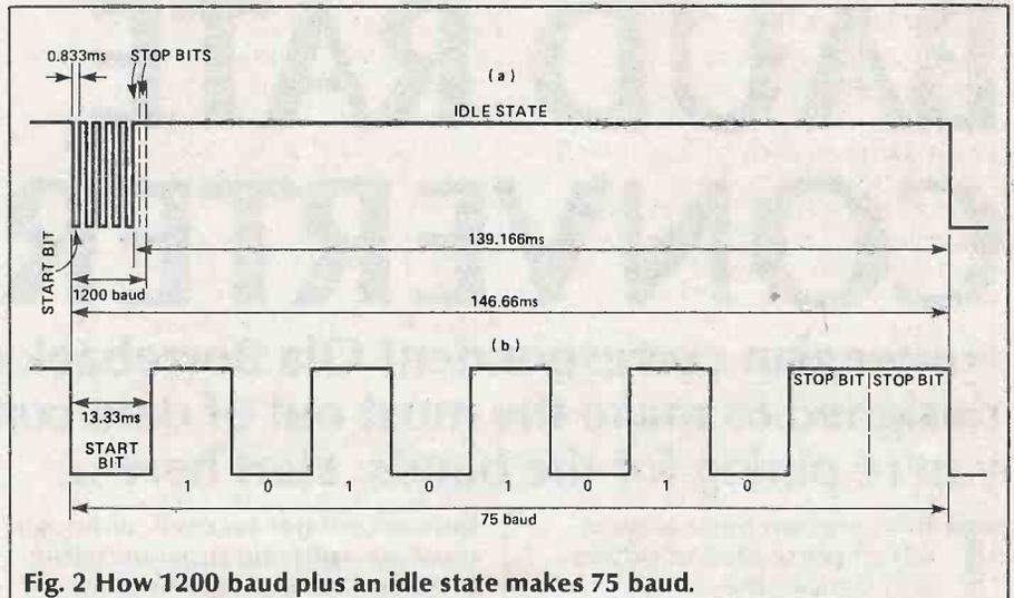
Fig. 2 How 1200 baud plus an idle state makes 75 baud.
