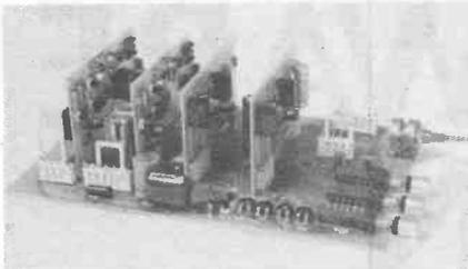
Complete record and replay circuits for very high quality low noise stereo cassette recorder. Circuits are optimised for our HS16 Super Quality Sendust Alloy Head. Switched bias and equalisation to cater for chrome and ferric tapes. Very easy to assemble on plug-in PCBs. Complete with full instructions.
