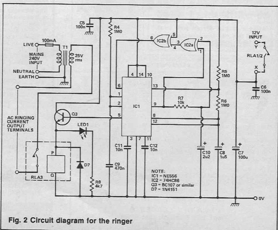
Fig. 2 Circuit diagram for the ringer
