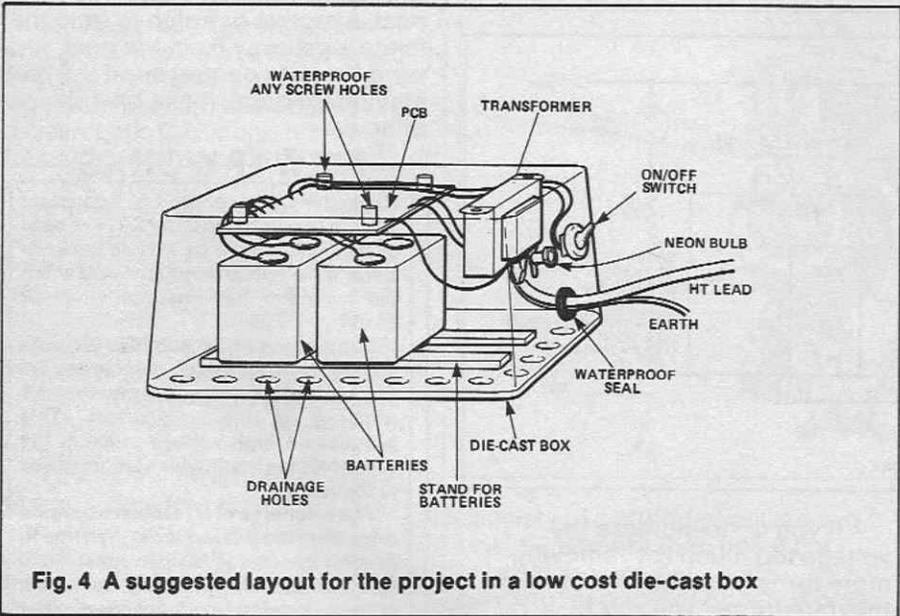
Fig. 4 A suggested layout for the project in a low cost die-cast box
