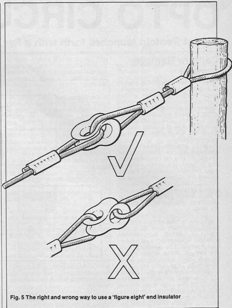
Fig. 5 The right and wrong way to use a 'figure eight' end insulator
