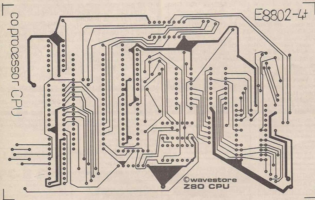
The Co-processor CPU board topside foil
