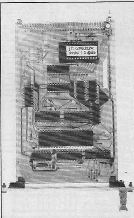
Spectrum. This consists of a connector for the Spectrum's expansion port, the bi-directional communication circuits and a three position mini-backplane for the co-processor CPU, DRAM and any other circuits the user may wish to add later such as analogue input or output or serial/parallel interfacing to the outside world.
