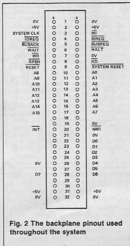
Fig. 2 The backplane pinout used throughout the system
