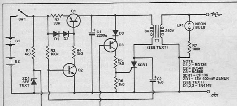
Fig. 2 The circuit of the ETI Electric Fencer
