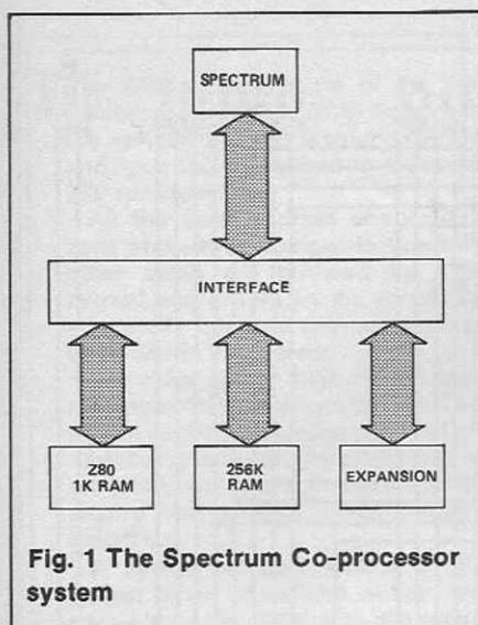
Fig. 1 The Spectrum Co-processor system
