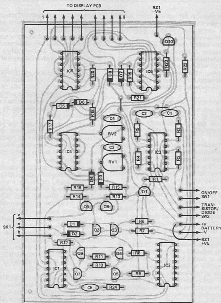
Fig. 2 Component overlay for the main PCB
