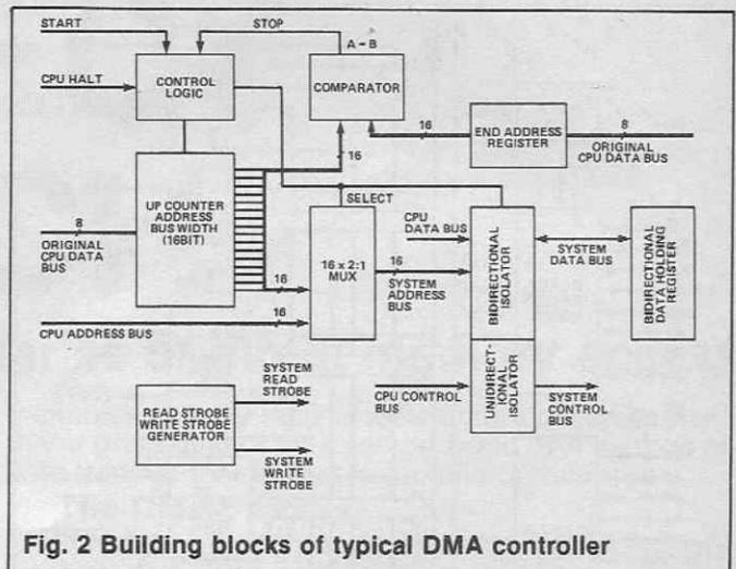
Fig. 2 Building blocks of typical DMA controller
