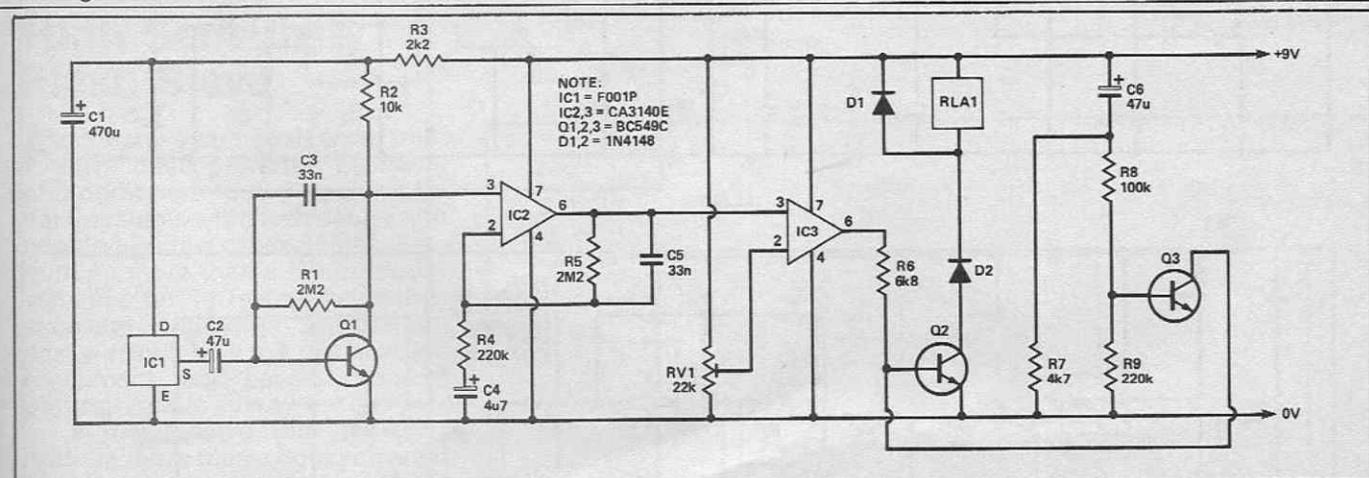
stand-by conditions the output of IC3 is in the low state and both Q2 and the relay are switched off.
