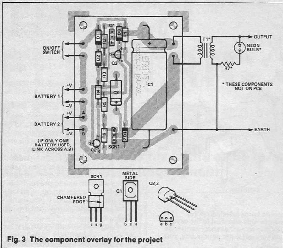
Fig. 3 The component overlay for the project
