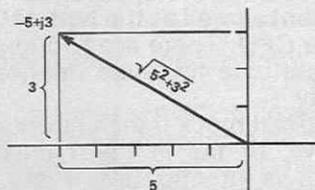
Fig. 5 The modulus of a complex number
