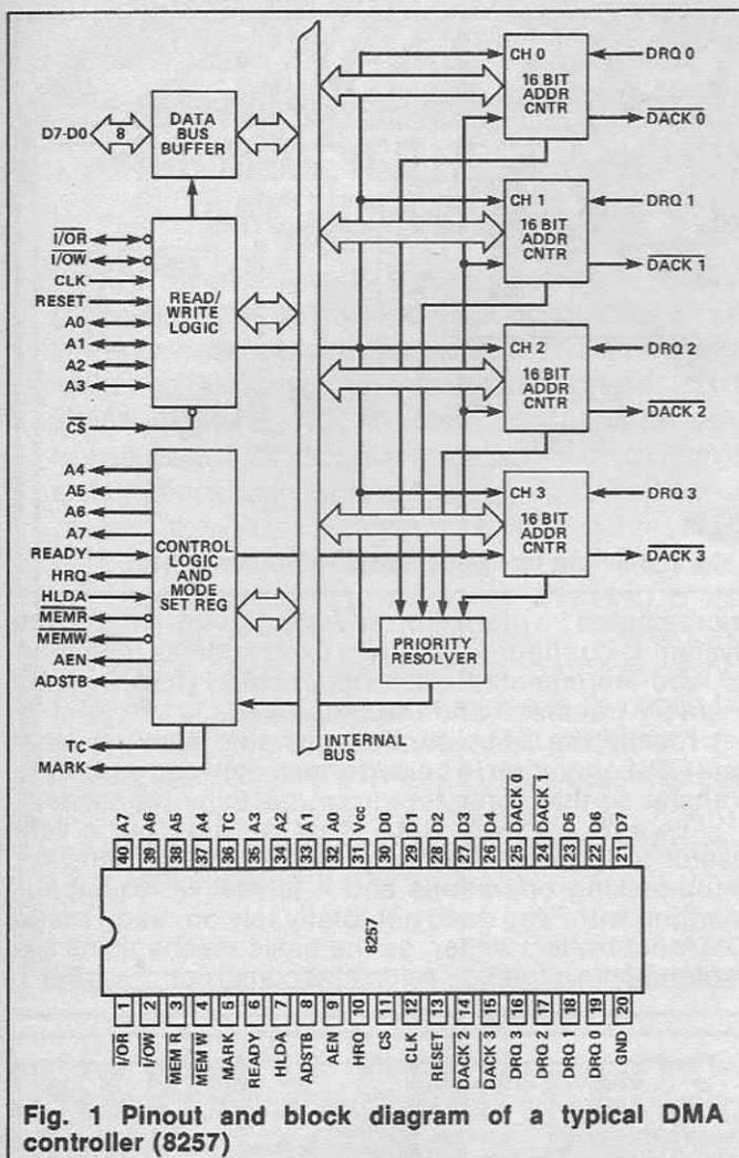
**Fig. 1 Pinout and block diagram of a typical DMA controller (8257)**
