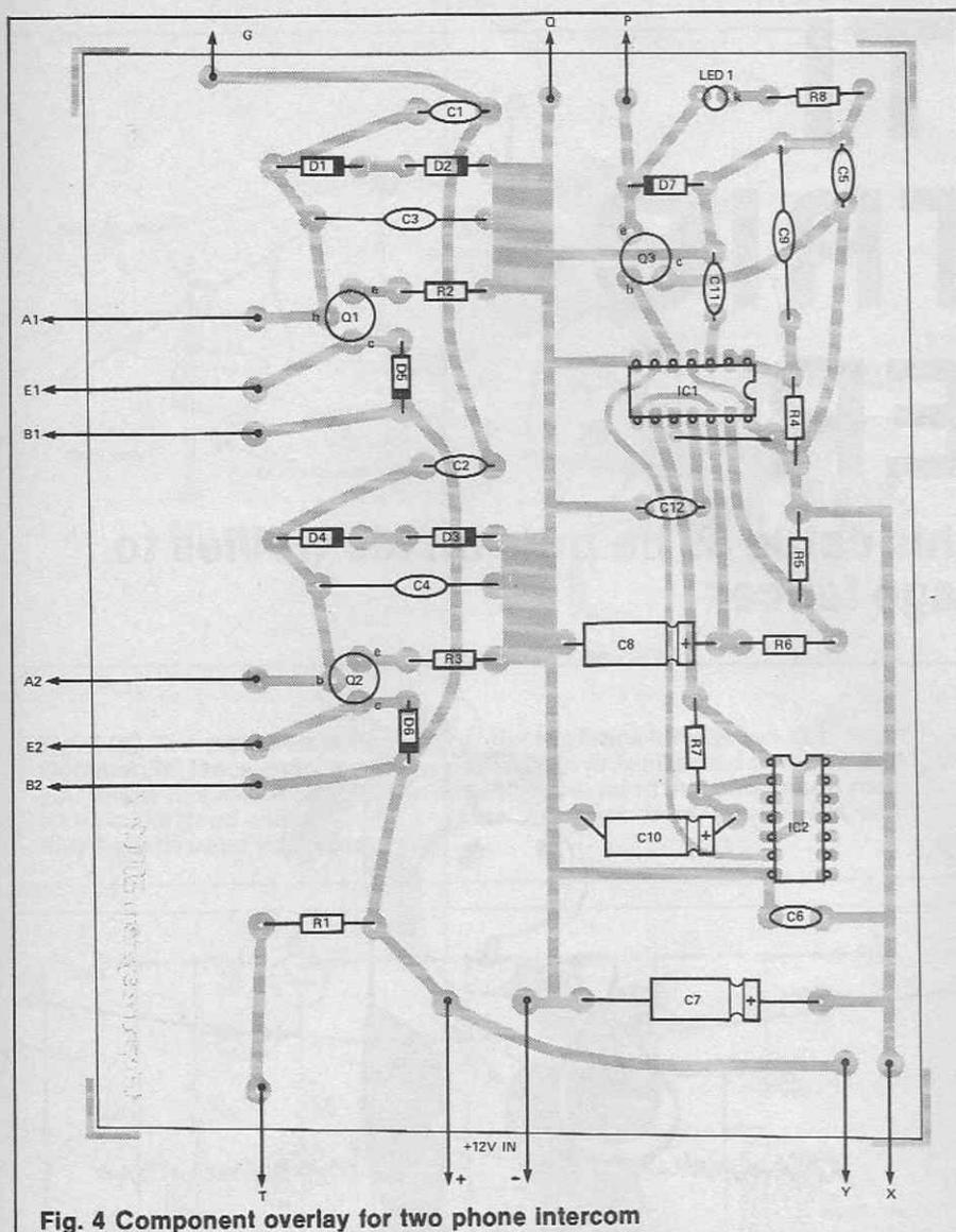
Fig. 4 Component overlay for two phone intercom
