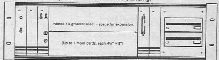
64K CPU | 64K DRAM | 64 x 24 | 100" | YOUR OWN EXPANSION (EG. SPEECH, SOUND, EPROM, PRINTER, MODEM, TAPE, RELAY, CONTROL, INTERFACING, ETC. ETC.) | ASCII ASCII | ASCII ASCII | 2 x 1 MBYTE 3 1/2" DISKS (EXAMPLE)
