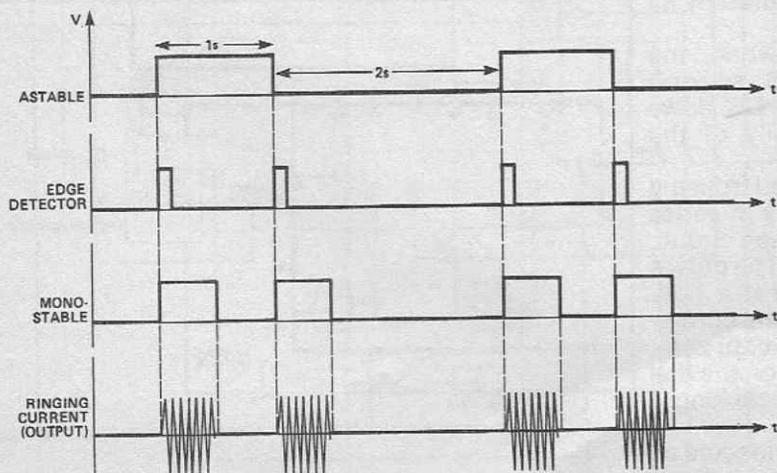
Fig. 3 Ringing generator waveforms and timing diagram
