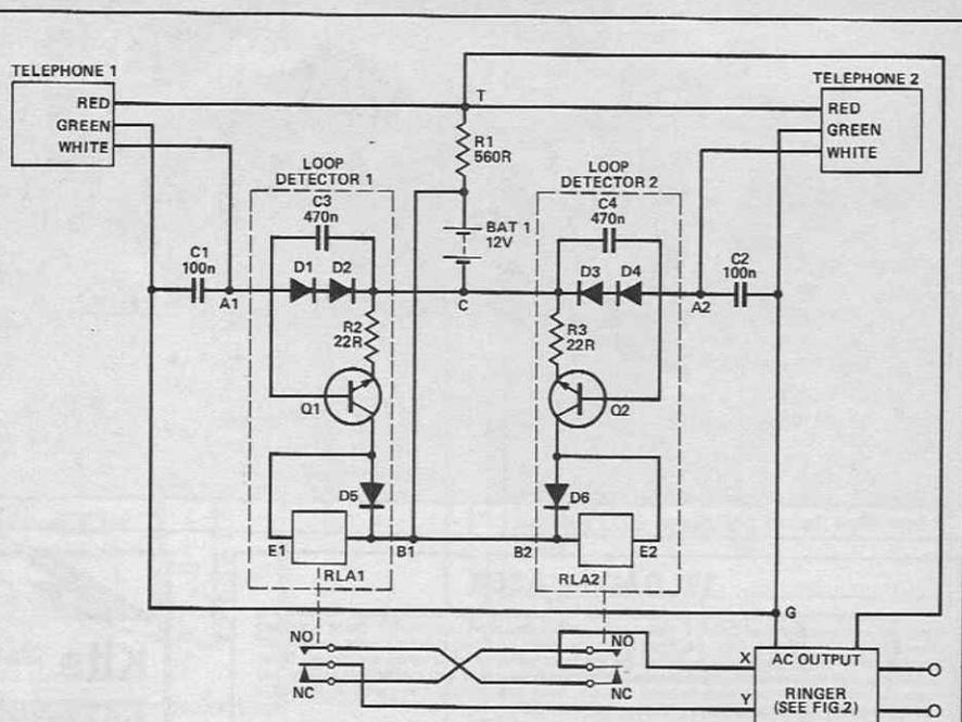
Fig. 1 Circuit diagram for a two phone intercom
