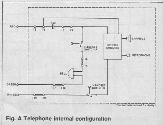
Fig. A Telephone internal configuration
