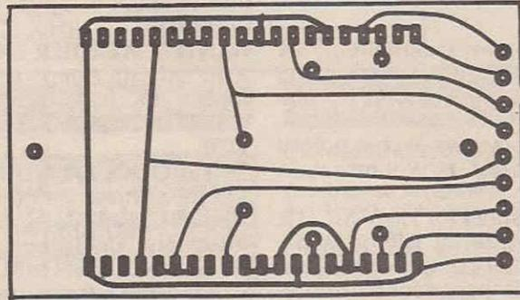
The Transistor Tester display board
