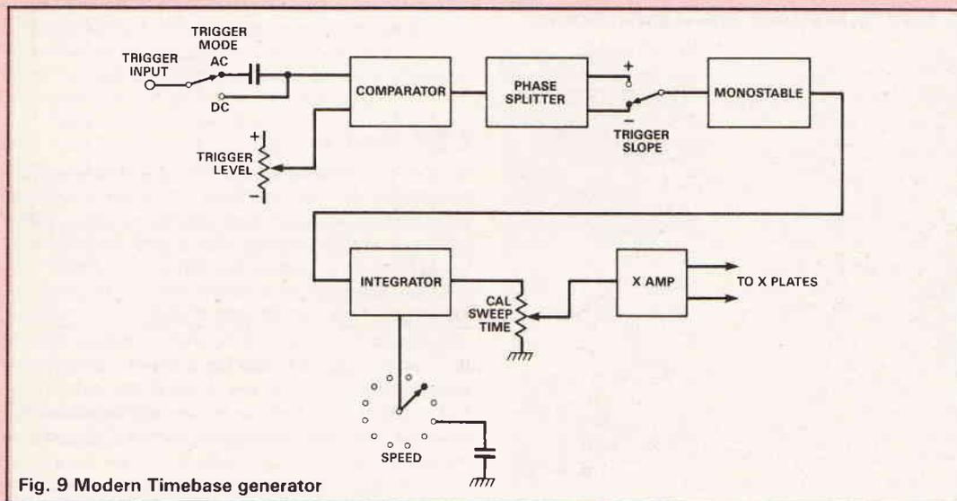
Fig. 9 Modern Timebase generator
