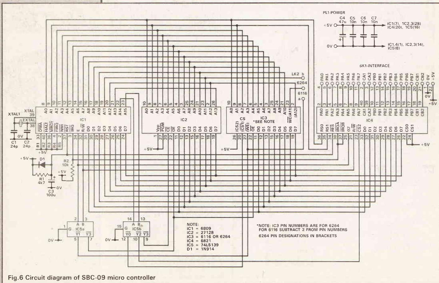
Fig.6 Circuit diagram of SBC-09 micro controller
