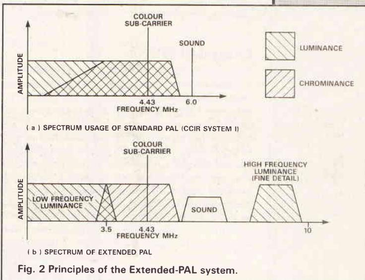
Fig. 2 Principles of the Extended-PAL system.
