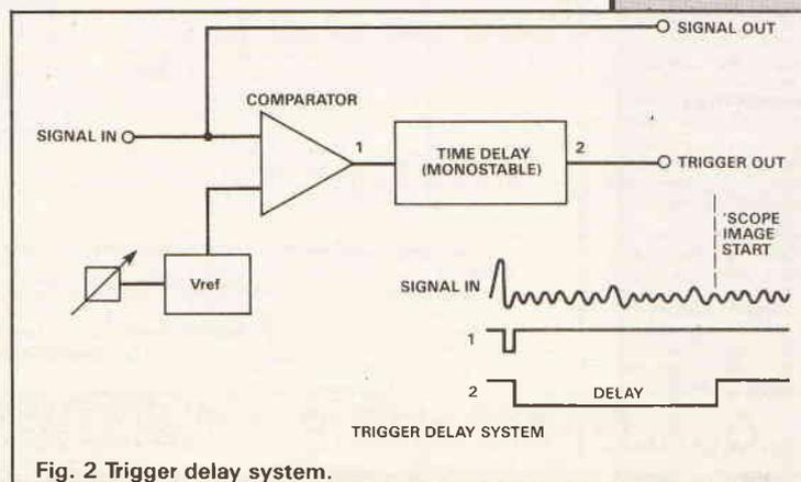
Fig. 2 Trigger delay system.
