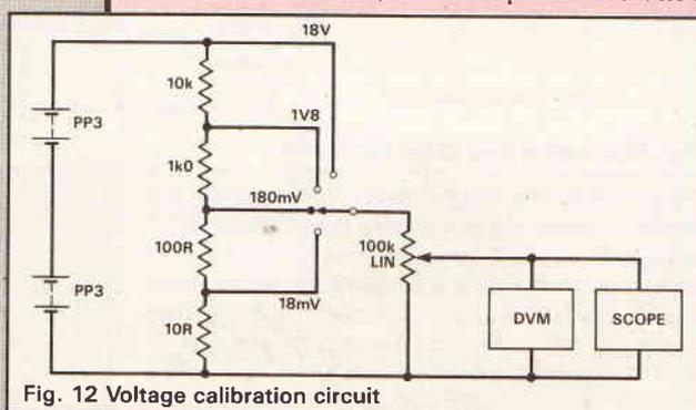
Fig. 12 Voltage calibration circuit
