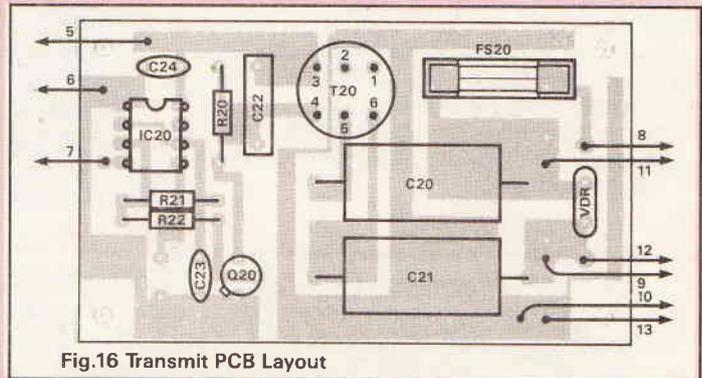
Fig.16 Transmit PCB Layout
