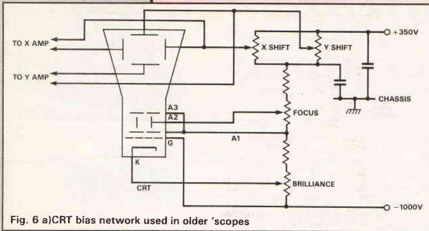
Fig. 6 a) CRT bias network used in older 'scopes
