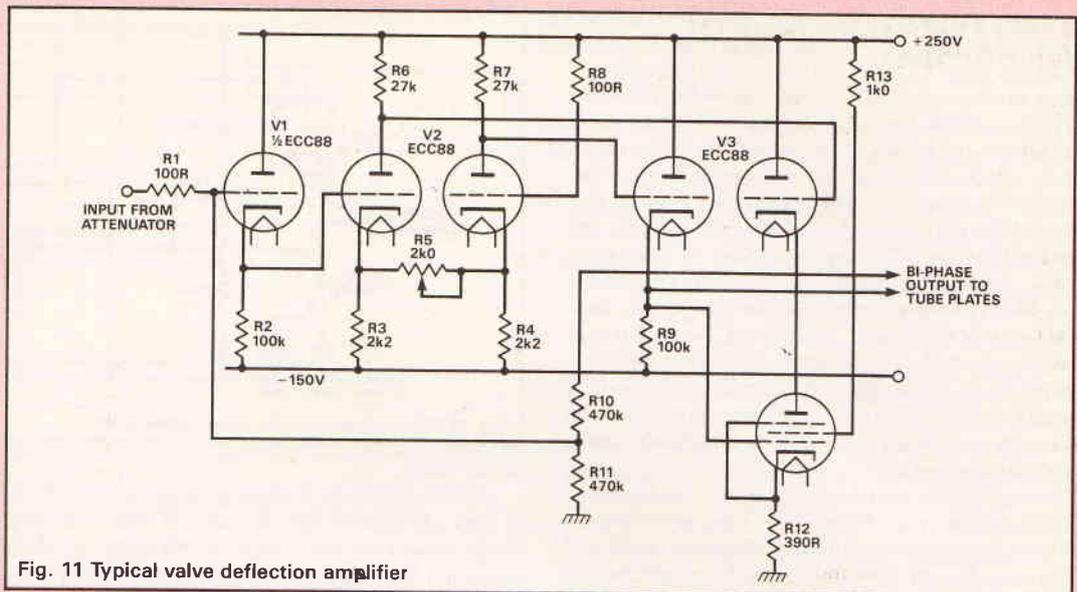
Fig. 11 Typical valve deflection amplifier
