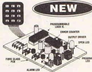
before the alarm is triggered is selected by you. Further entries will be ignored for a time also set by you. Only the correct sequence will open the lock and switch off the alarm. The sequence may easily be changed by entering a special number and code on the supplied keyboard. Kit includes; keyboard, alarm buzzer, high quality PCB and all electronic components. Supply 5-15V DC. Will drive our Latch Mechanism (701 150 @ £16.50) or relay directly.
