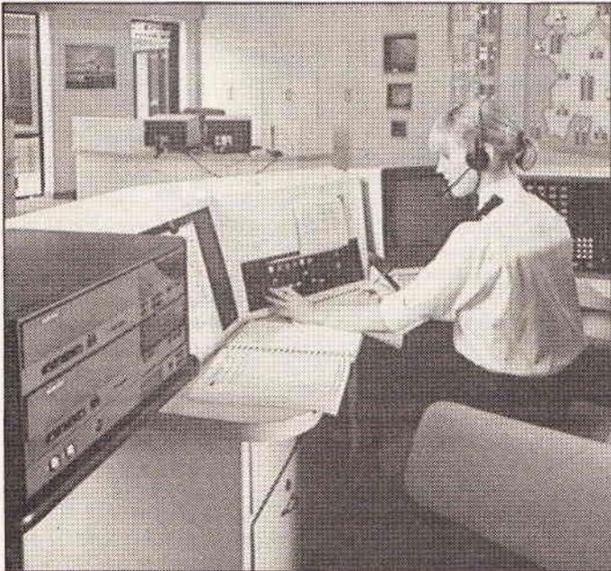
Wordsafe, the world's first desk-top multi-channel voice logging recorder incorporating helical scan technology, has been unveiled by Racal Recorders Limited. Wordsafe is the first communications recorder to provide up to 32 channels and more than 24 hours' continuous recording on a standard VHS cassette in a compact machine.
