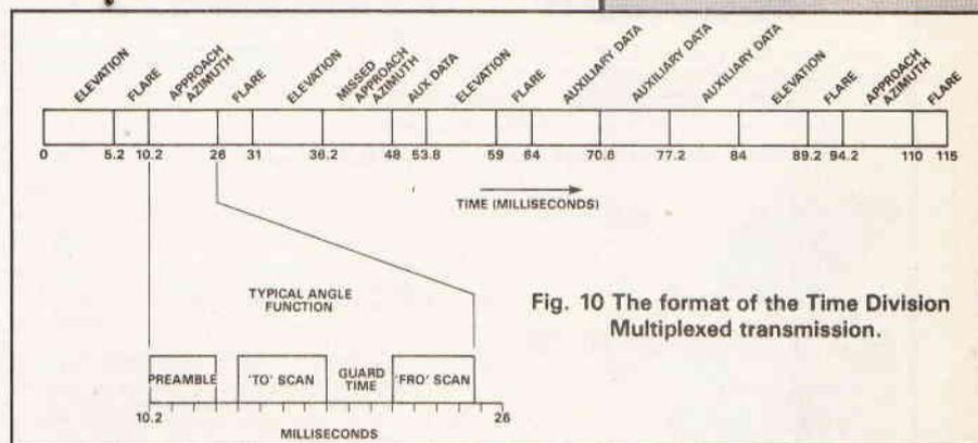
Fig. 10 The format of the Time Division Multiplexed transmission.
