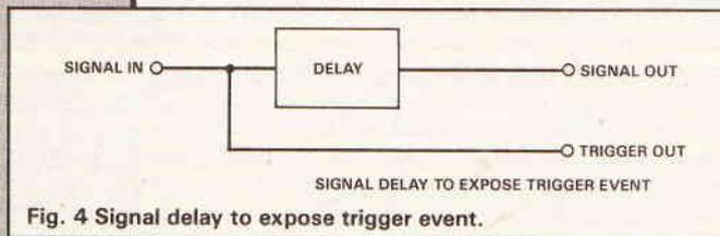
Fig. 4 Signal delay to expose trigger event.
