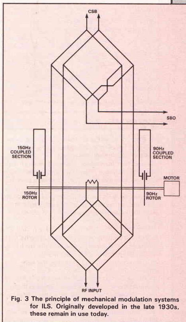
Fig. 3 The principle of mechanical modulation systems for ILS. Originally developed in the late 1930s, these remain in use today.
