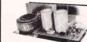
**OMP/MF200 Mos-Fet** Output power 200 watts R.M.S. into 4 ohms, Frequency Response 1Hz - 100KHz -3dB, Damping Factor >300, Slew Rate 50V/uS, T.H.D. Typical 0.001%, Input Sensitivity 500mV, S.N.R. -130dB, Size 300 x 155 x 100mm, PRICE £62.99 + £3.50 P&P.
