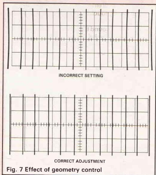
Fig. 7 Effect of geometry control
