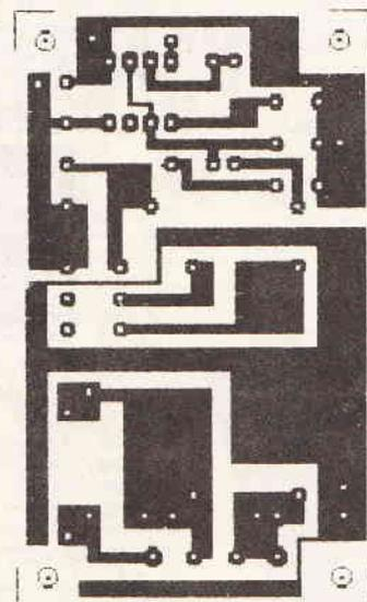
Remote Control Timeswitch Transmitter Board
