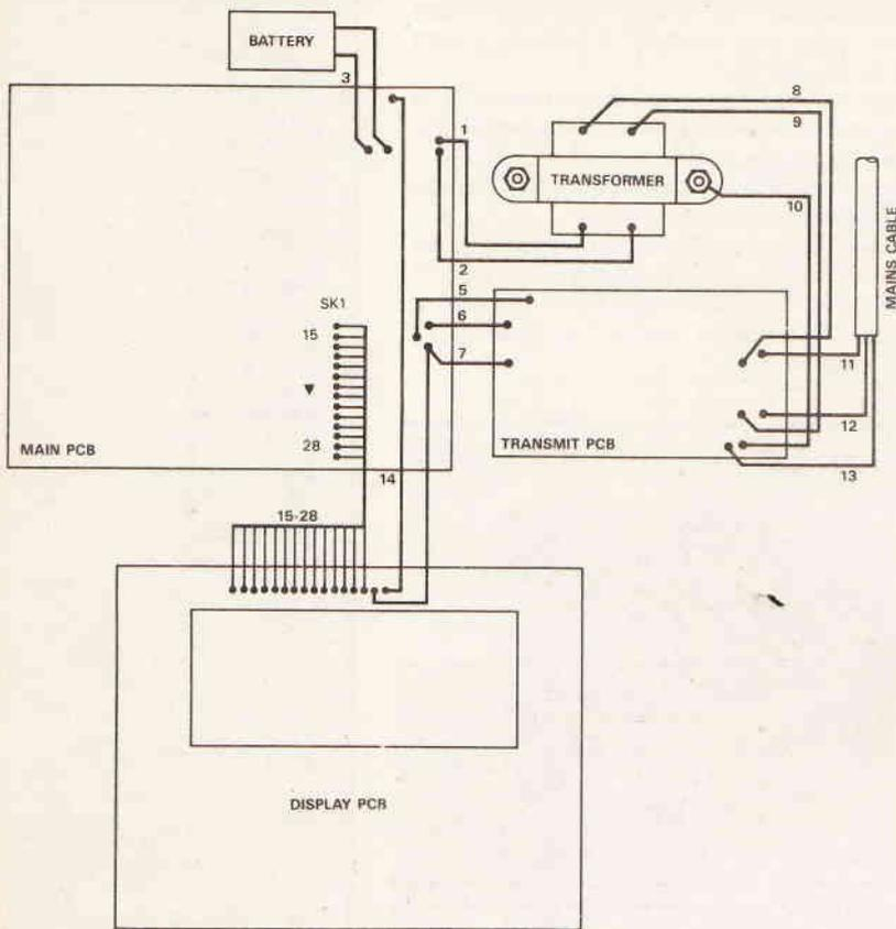
Fig.15 Main Control Unit — Inter PCB wiring
