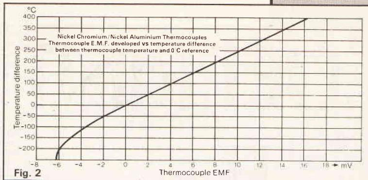
Figure 2 shows the typical response of a thermocouple. As can be seen, the output signal over the normal range of operation is 40V per °C. While measurable, this signal is too low for most electronic applications, so the first task is to amplify it. The circuit shown in Figure 3 incorporates on its input an amplifier which raises the signal level to approximately 2mV per °C.
