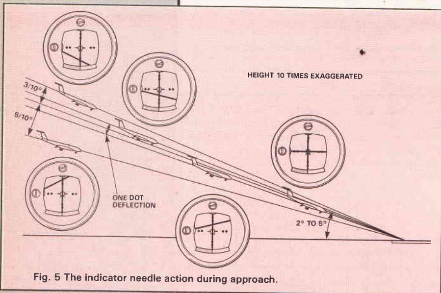
Fig. 5 The indicator needle action during approach.
