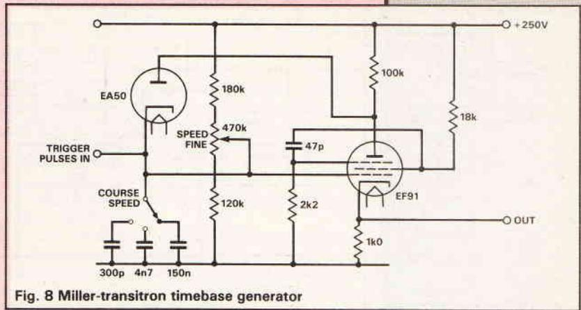
Fig. 8 Miller-transitron timebase generator
