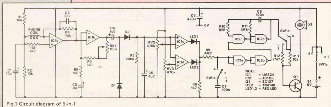
Fig.1 Circuit diagram of 5-in-1
