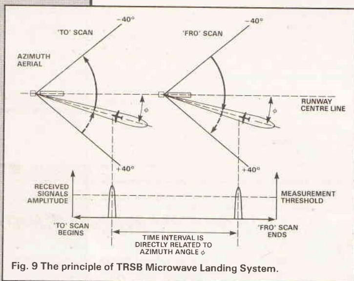
Fig. 9 The principle of TRSB Microwave Landing System.
