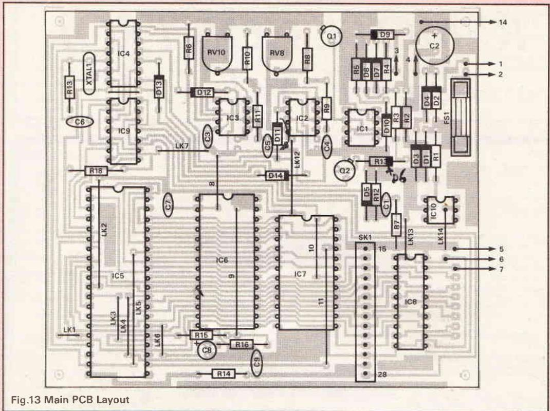
Fig.13 Main PCB Layout
