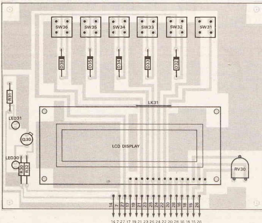
Fig.14 Display PCB Layout
