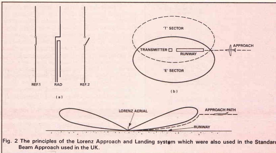
Fig. 2 The principles of the Lorenz Approach and Landing system which were also used in the Standard Beam Approach used in the UK.
