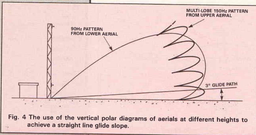
Fig. 4 The use of the vertical polar diagrams of aeriels at different heights to achieve a straight line glide slope.
