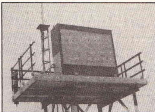
Fig. 11 The Azimuth transmitter of the MLS installation at Port Hawkesbury, Nova Scotia. The equipment is mounted on a tower to ensure coverage over a hump in the runway. The vertical aerial to the left of the main array is for Distance Measuring Equipment which gives the aircraft its distance from touchdown.
