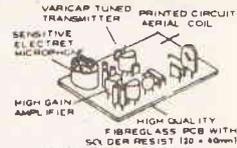
Only 45x25x15mm, including built-in mic. 88-100MHz (standard FM radio). Range approx. 300m depending on terrain. Powered by 9V PP3 (7mA). Ideal for surveillance, baby alarm etc.
