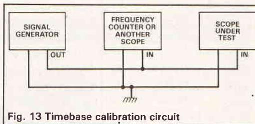
Fig. 13 Timebase calibration circuit
