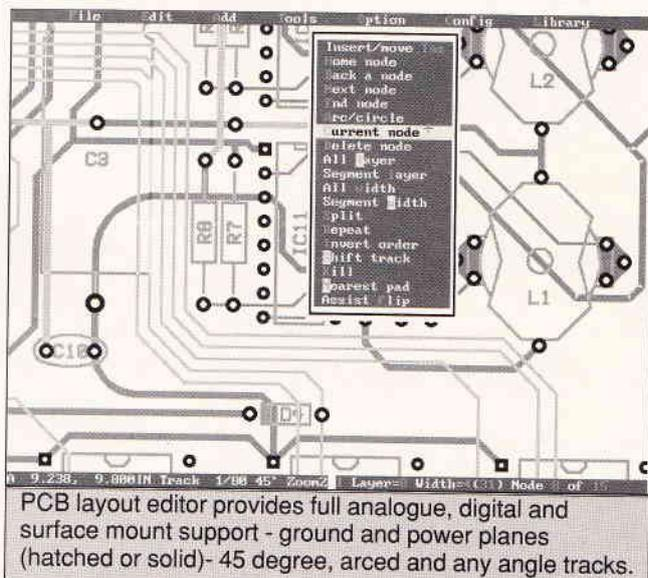
PCB layout editor provides full analogue, digital and surface mount support - ground and power planes (hatched or solid) - 45 degree, arced and any angle tracks.
