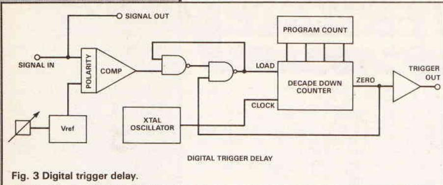
Fig. 3 Digital trigger delay.
