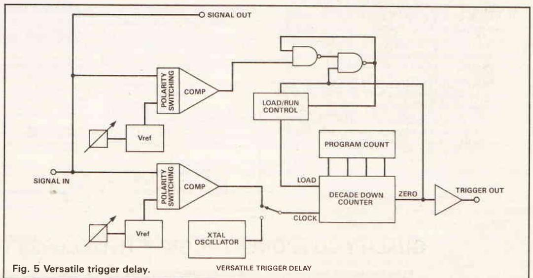
Fig. 5 Versatile trigger delay.
