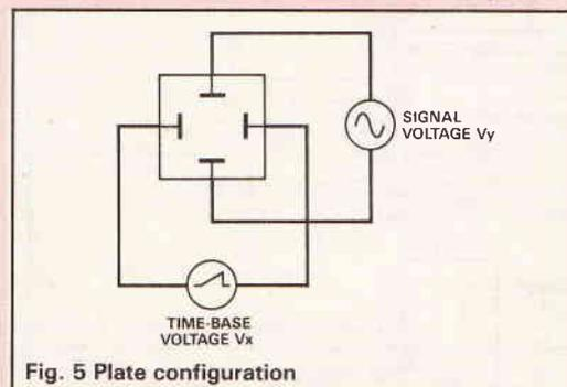
Fig. 5 Plate configuration
