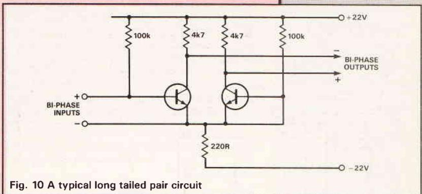
Fig. 10 A typical long tailed pair circuit
