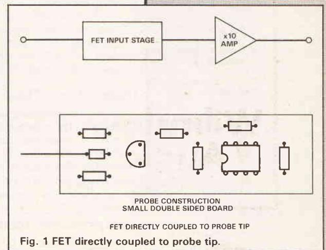
Fig. 1 FET directly coupled to probe tip.
