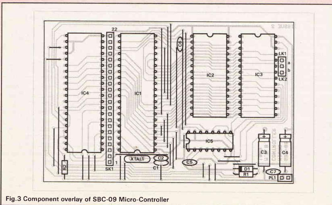
Fig.3 Component overlay of SBC-09 Micro-Controller
