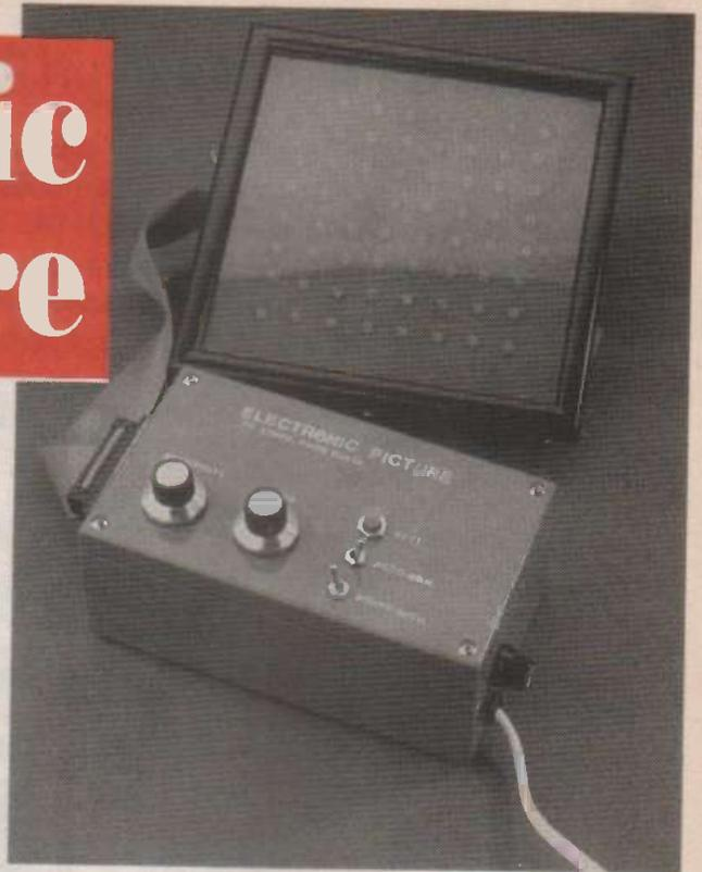
This feature is of little use for text messages but very good visual effects can be created. Both modes of operation have controls that allow the sensitivity or speed to be altered. A switch allows either sound or automatic mode to be selected. The circuit can store 16 different sequences, which can be individually selected (a push button allows you to cycle through the sequences), or all the sequences can be displayed in turn after a set number of repetitions.
