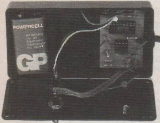
resistance mode (i.e. R3 selected), the audio alarm should be activated if a 4R7 resistor is connected across the prods. However, changing to a 22R resistor should not give a response from the unit. With the tester set to the low resistance mode (i.e. R2 selected), connecting the 4R7 or 22R test resistors across the test prods should fail to activate the audio tone generator. Using a 0R47
